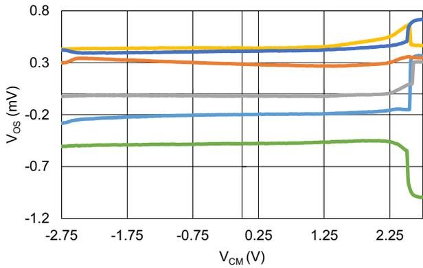
Figure 11. Offset Voltage vs Common-Mode Voltage
