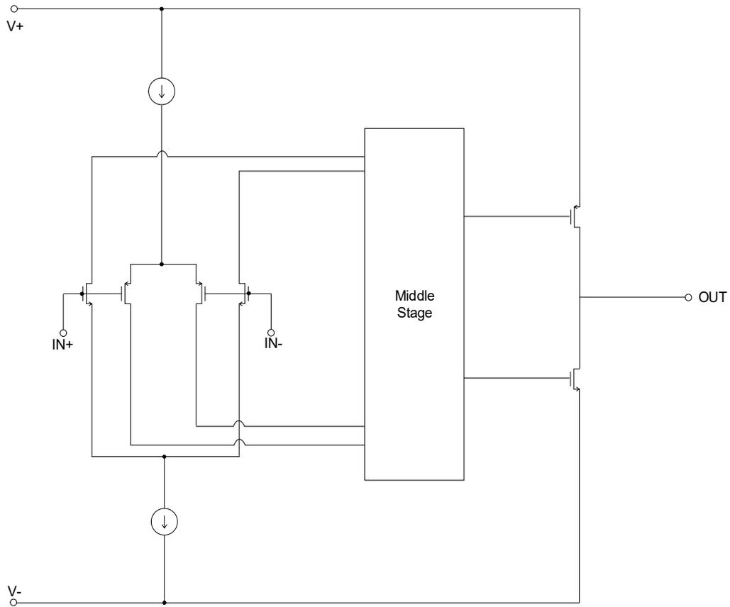
Figure 2. Block Diagram of a Single Amplifier Stage
