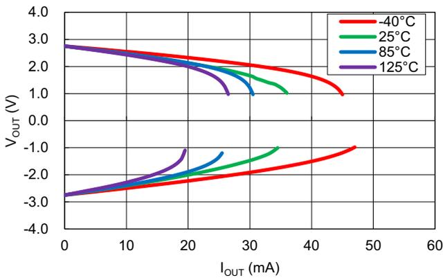
Figure 19. Output Voltage vs Output Current
