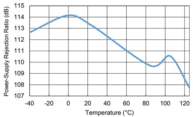
Figure 22. DC PSRR vs Temperature
