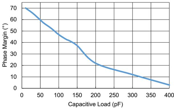
**Figure 33. Phase Margin vs Capacitive Load**
