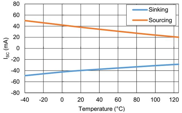
Figure 8. Short-Circuit Current vs Temperature
