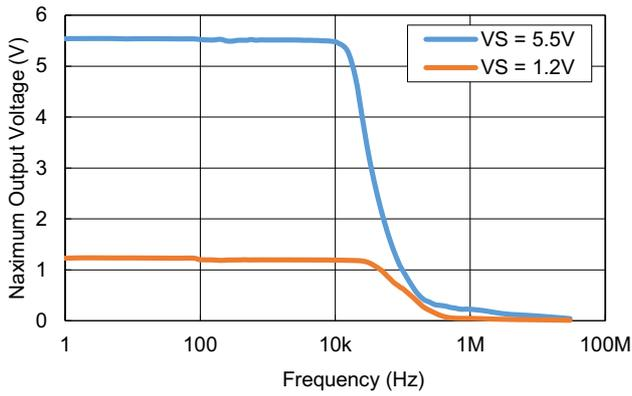
Figure 41. Maximum Output Voltage vs Frequency
