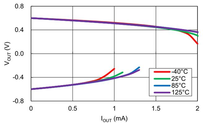
Figure 20. Output Voltage vs Output Current
