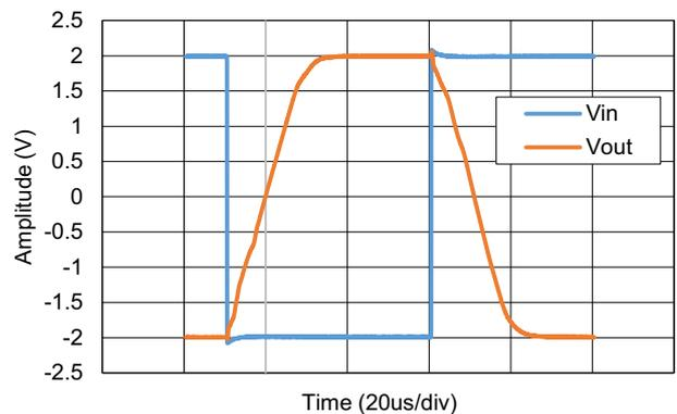
**Figure 40. Large Signal Step Response**
