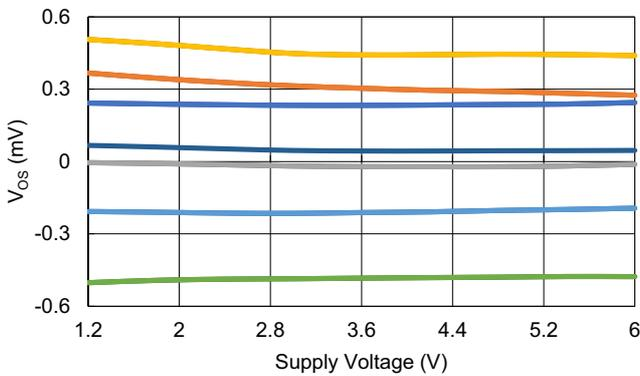
Figure 13. Offset Voltage vs Supply Voltage  $V_{CM} = (V-)$
