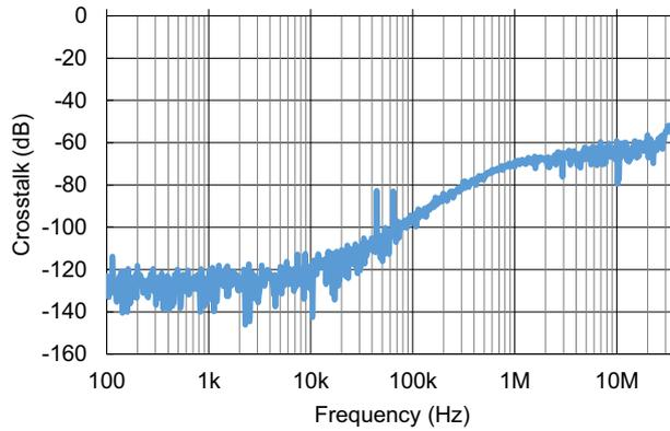
Figure 43. Channel Separation
