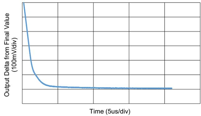
**Figure 38. Large Signal Settling Time (Negative)**
