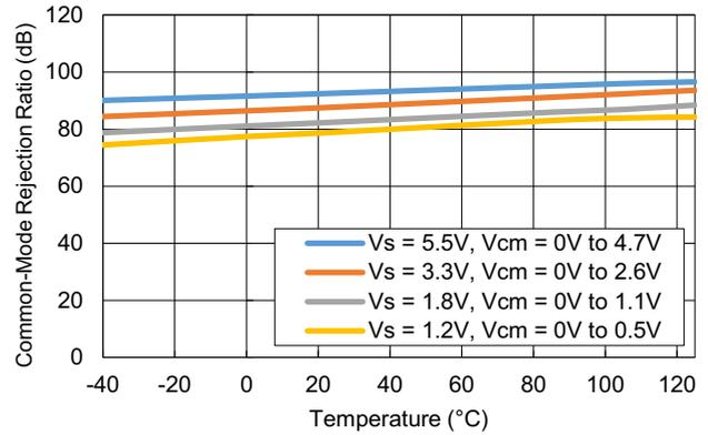
Figure 24. DC CMRR vs Temperature
