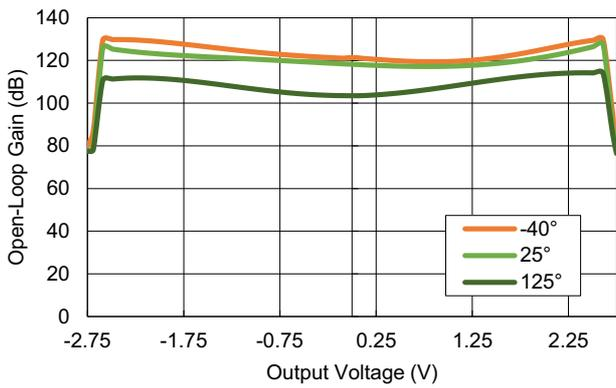
Figure 17. Open-Loop Gain vs Output Voltage
