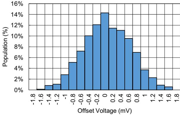
Figure 7. Offset Voltage Distribution
