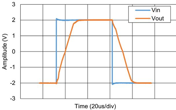
**Figure 37. Large Signal Step Response**
