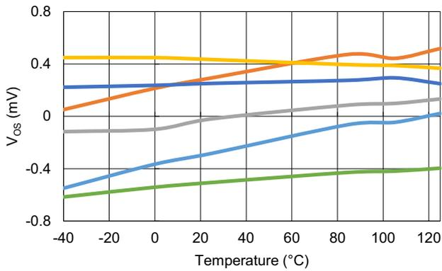
Figure 9. Offset Voltage vs Temperature
