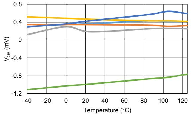
Figure 10. Offset Voltage vs Temperature
