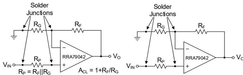
Figure 47. Schematic Representation
