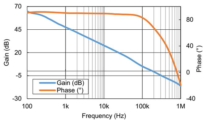
Figure 16. Open-Loop Gain and Phase vs Frequency
