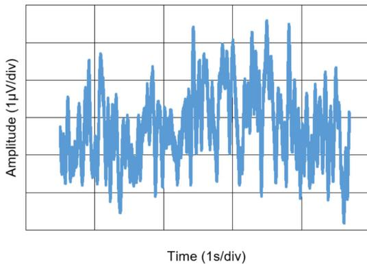
Figure 25. 0.1Hz to 10Hz Voltage Noise in Time Domain
