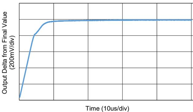
**Figure 39. Large Signal Settling-Time (Positive)**
