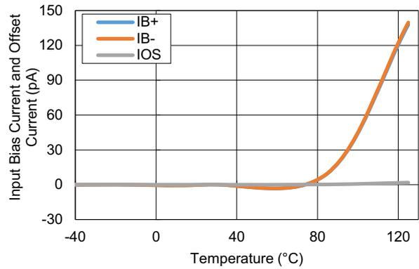
Figure 14. Input Bias and Offset Current vs Temperature
