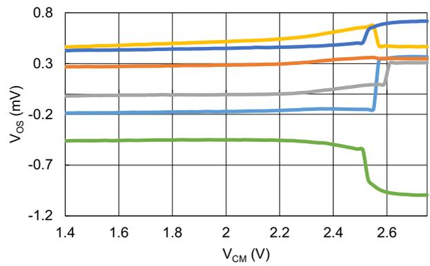
Figure 12. Offset Voltage vs Common-Mode Voltage  $V_{CM} > (V+) - 1.4V$
