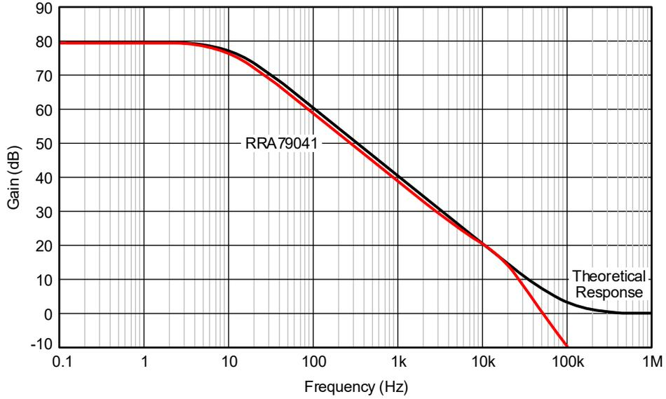
Figure 46. High-Gain Amplifier Frequency Response
