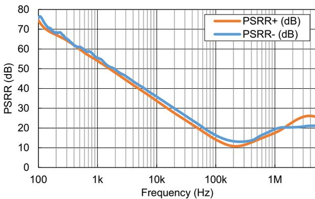
Figure 21. PSRR vs Frequency
