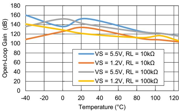
Figure 15. Open-Loop Gain vs Temperature
