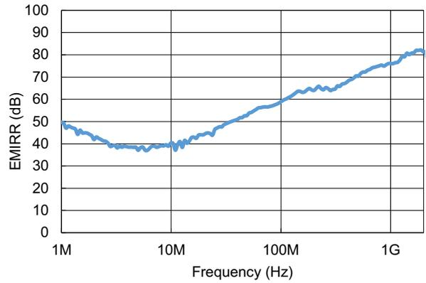
Figure 42. Electromagnetic Interference Rejection Ratio Referred to Non-Inverting Input (EMIRR+) vs Frequency
