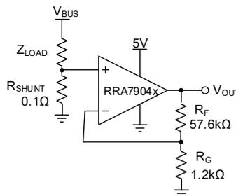
Figure 45. Low-Side Current Sensing Application
