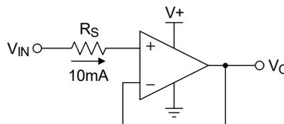
Figure 44. Input Current Protection
