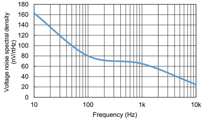
Figure 26. Voltage Noise Spectral Density
