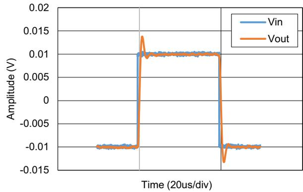
**Figure 36. Small Signal Step Response**
