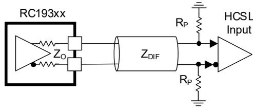
Figure 18. Direct-Coupled Double-Terminated HCSL
