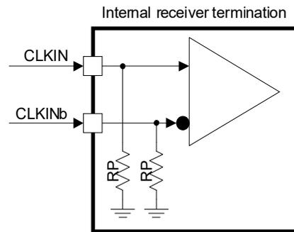
Figure 16. Receiver Termination
