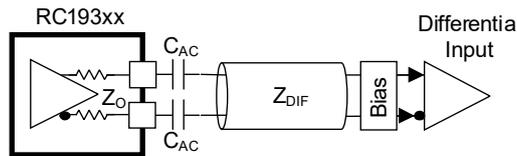
Figure 19. AC-Coupled Differential Input with Bias Network
