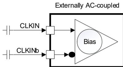
Figure 15. External AC-Coupling
