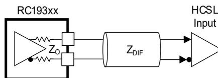
Figure 17. Direct-Coupled Source-Terminated HCSL ( $Z_{OUT\_SEL\_tri} = 0$  or  $1$ )
