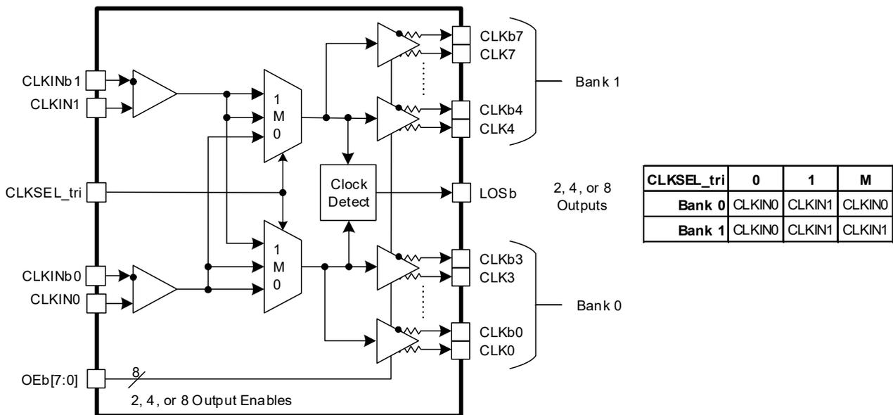
Figure 1. Simplified Block Diagram and Mux Logic
