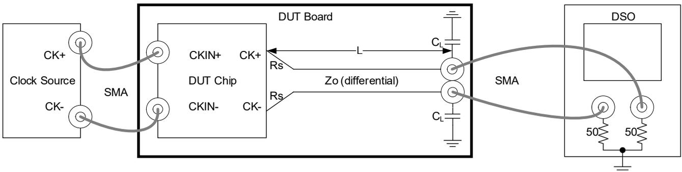
Figure 11. AC/DC Test Load for Differential Outputs (Double-Terminated or Receiver-Terminated)
