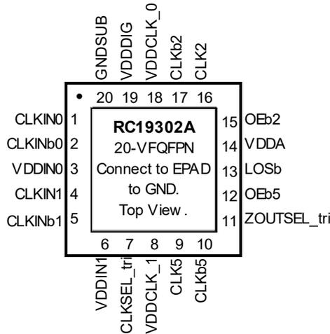
Figure 7. RC19302A Pin Assignments
