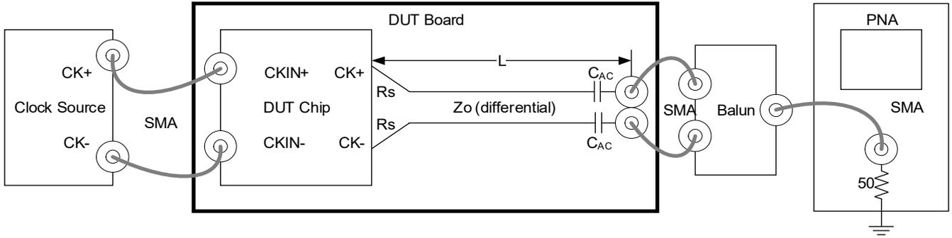
Figure 12. Test Load for PCIe Phase Jitter Measurements
