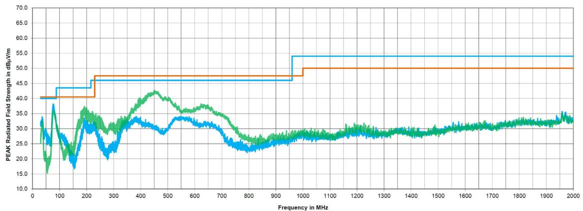
Figure 40. FCC Part15/CISPR22 Class B Radiated Emissions at 3 Meters, 230V<sub>AC</sub>, 50Hz (Peak Detector)
