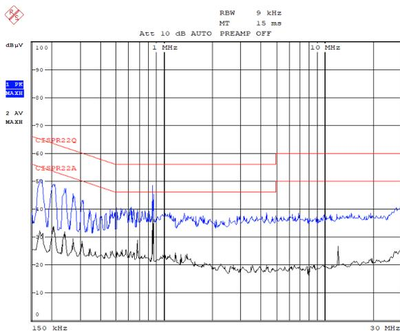
Figure 35. Line, 120V<sub>AC</sub>
