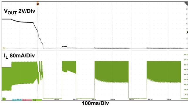
Figure 15. Overload Protection
