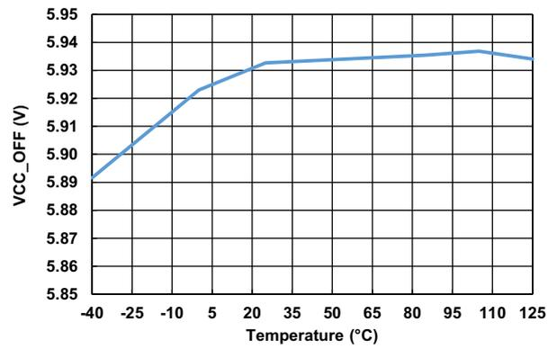
Figure 6. V<sub>CC</sub> Start/Upper Limit vs Temperature
