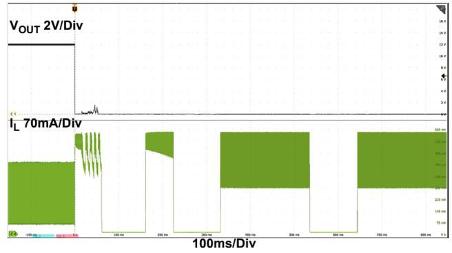
Figure 16. Short-Circuit Protection
