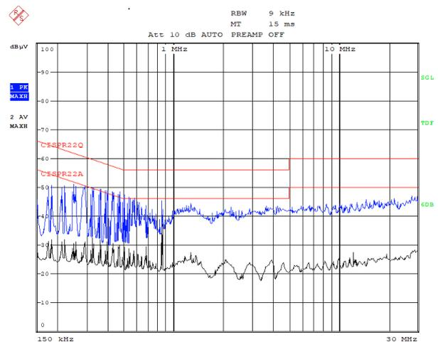
Figure 36. Line, 230V<sub>AC</sub>
