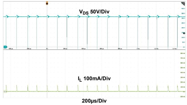
Figure 14. Light-Load Operation
