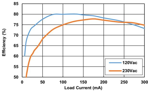
Figure 19. Efficiency ( $V_{OUT} = 12V$ )
