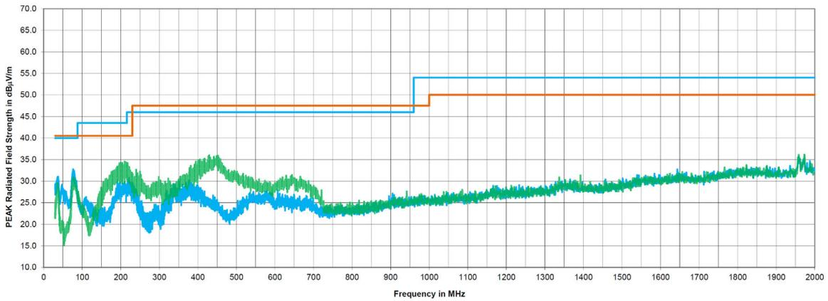
Figure 39. FCC Part15/CISPR22 Class B Radiated Emissions at 3 Meters, 120V<sub>AC</sub>, 60Hz (Peak Detector)
