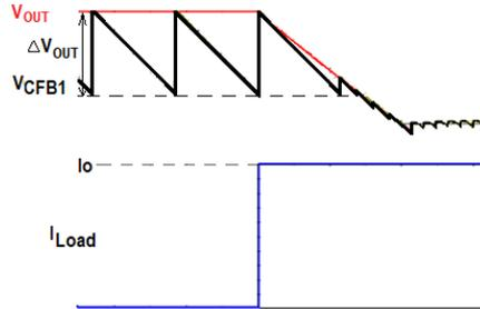
Figure 33. Output Capacitor Discharging at Step Load
