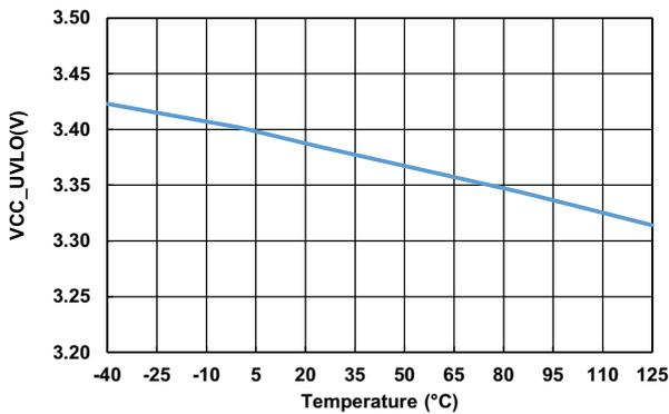
Figure 7. V<sub>CC</sub> Undervoltage Threshold vs Temperature
