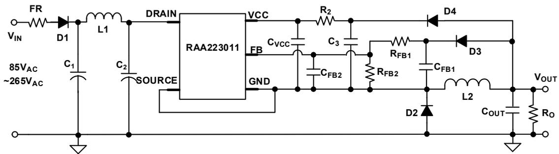
Figure 24. RAA223011 Low Standby Power Buck Regulator
