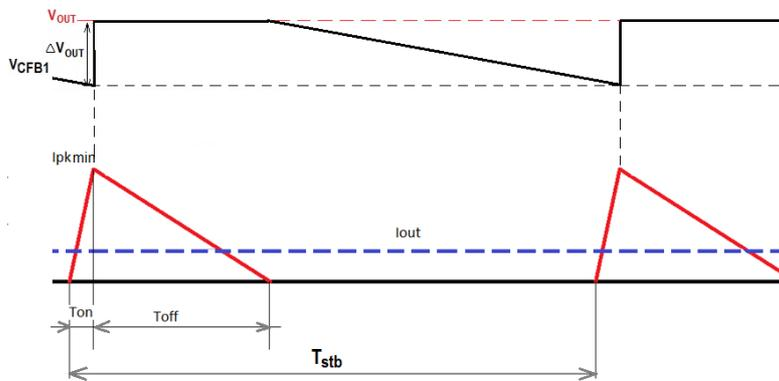
Figure 32. The Inductor Current at No Load Operation
