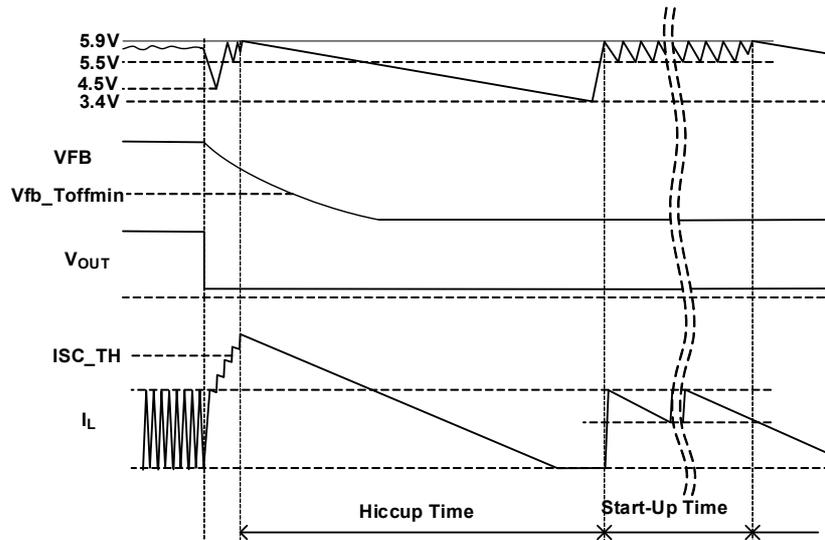
Figure 27. RAA223011 Short-Circuit Protection Diagram
