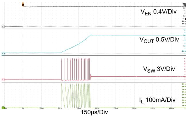
Figure 13. Startup through EN (No Load): RAA211803
