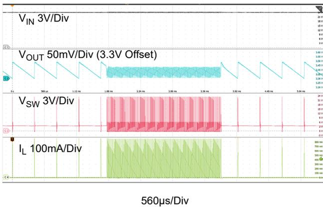
Figure 25. Load Transient (10mA to 300mA): RAA211803
