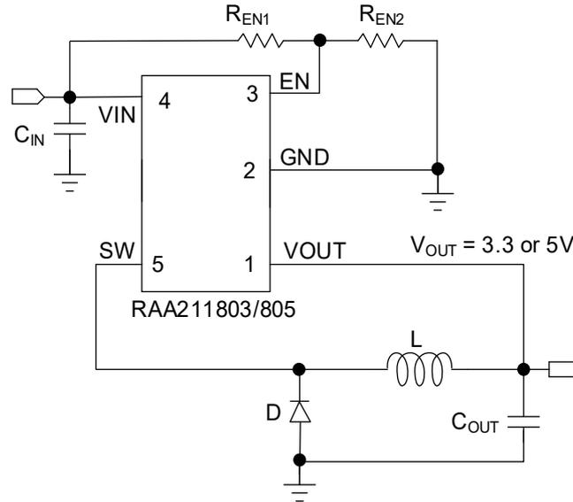
Figure 43. Typical Application Circuit Diagram with  $V_{IN}$  UVLO Programming by ENABLE
