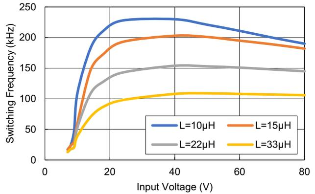
Figure 50. Switching Frequency vs Input Voltage
