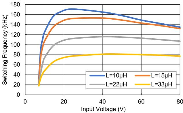
Figure 49. Switching Frequency vs Input Voltage
