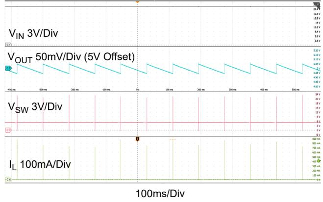
Figure 24. Typical Operation (No Load): RAA211805
