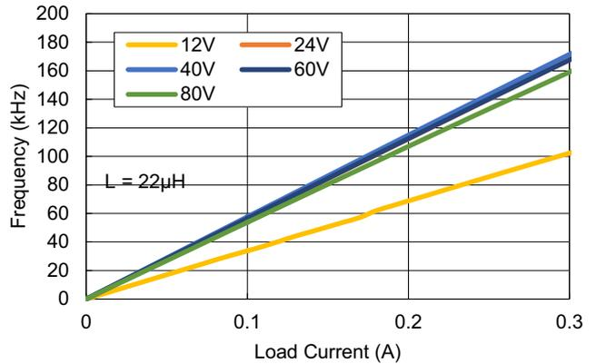
Figure 46. Switching Frequency vs Load Current RAA211805
