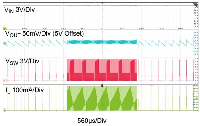
Figure 26. Load Transient (10mA to 300mA): RAA211805
