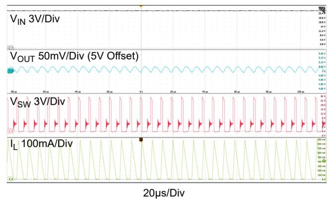
Figure 22. Typical Operation (Full Load): RAA211805
