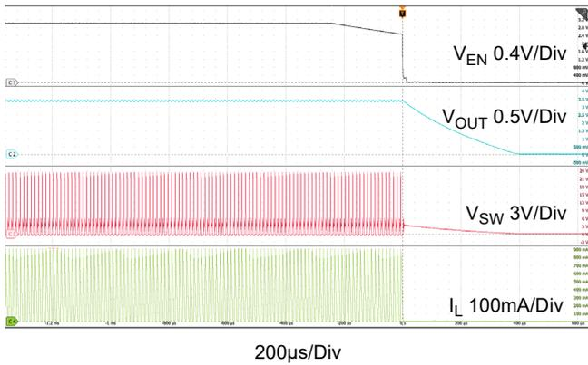
Figure 11. Shutdown through EN: RAA211803
