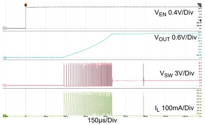
Figure 14. Shutdown through EN (No Load): RAA211805
