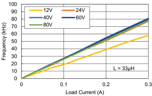
Figure 45. Switching Frequency vs Load Current RAA211803
