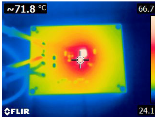
Figure 25. Thermal Image, 36V IN , 3.3V OUT , 400kHz, 5A, HTSSOP, T J = 71.8°C
