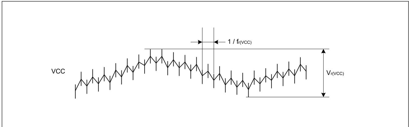
**Figure 2.2** Ripple waveform
