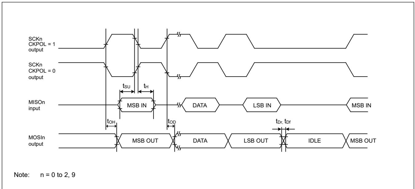
Figure 2.24 SCI simple SPI mode timing (master, CKPH = 0)
