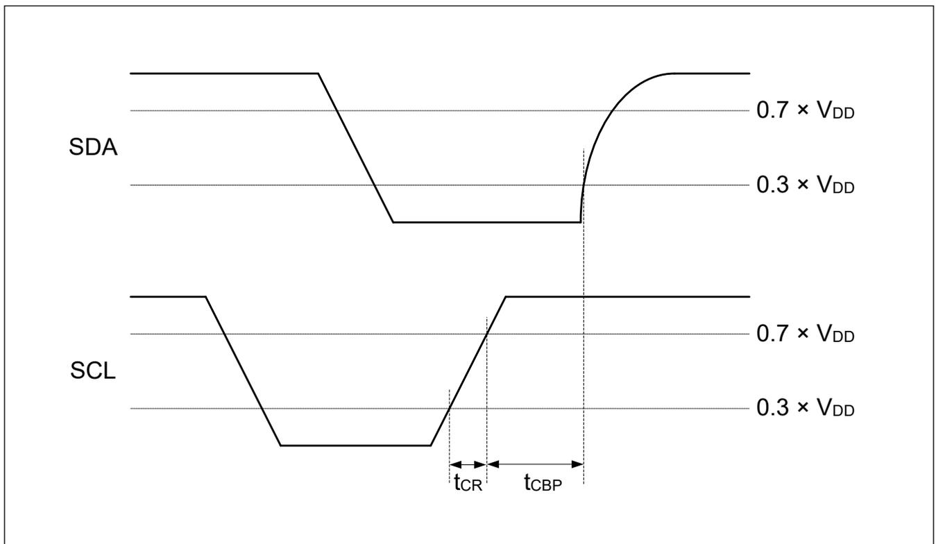
Figure 2.39 I3C STOP condition Timing
