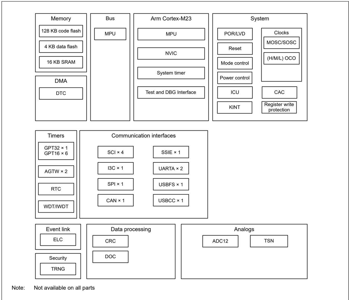
Figure 1.1 Block diagram
