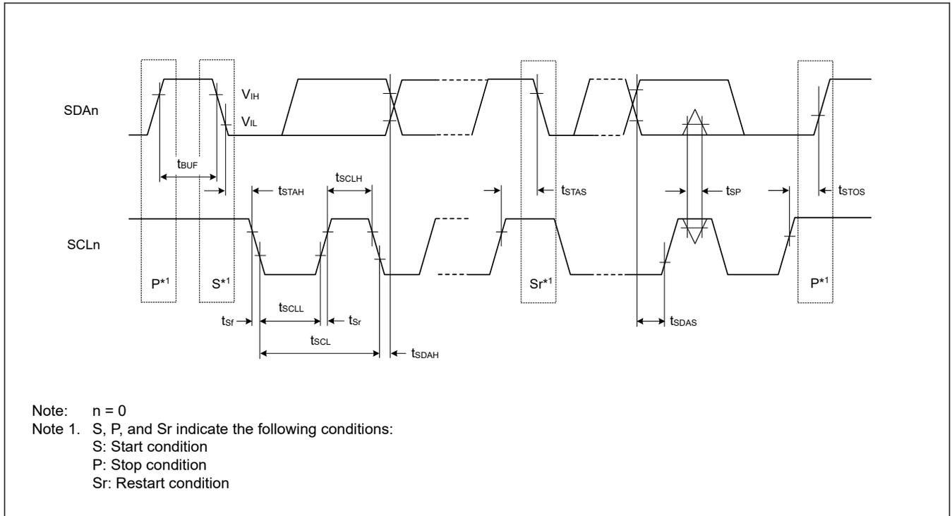
Figure 2.35 I<sup>2</sup>C bus interface input/output timing
