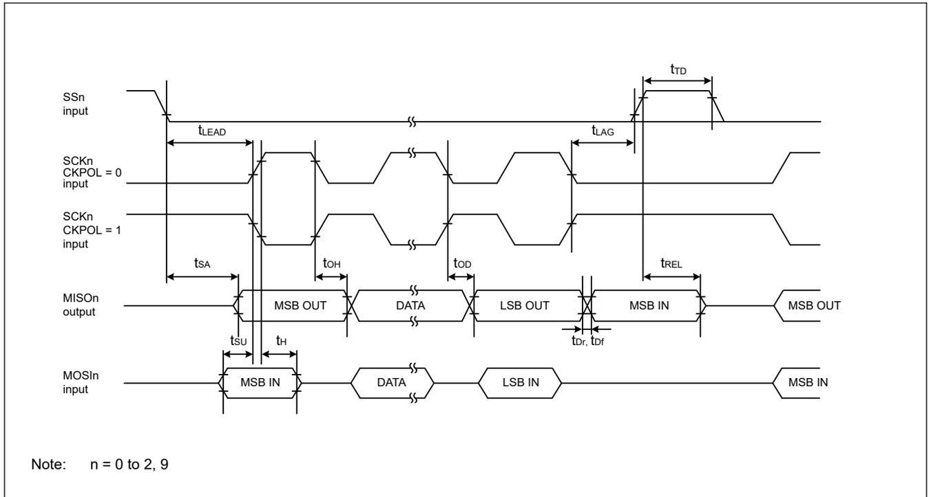
Figure 2.25 SCI simple SPI mode timing (slave, CKPH = 1)
