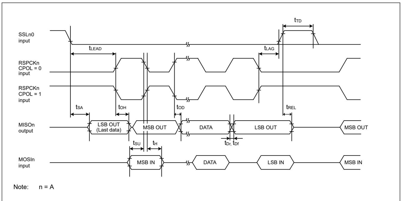
Figure 2.34 SPI timing (slave, CPHA = 1)
