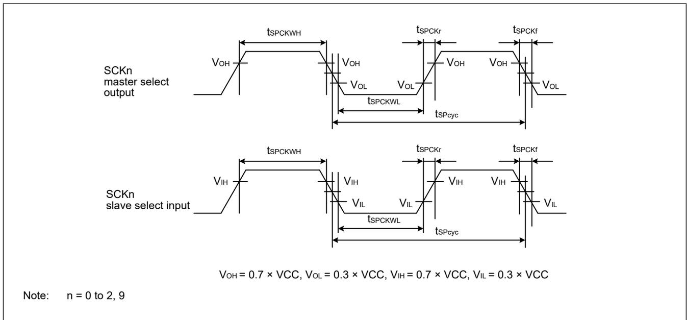
**Figure 2.22 SCI simple SPI mode clock timing**
