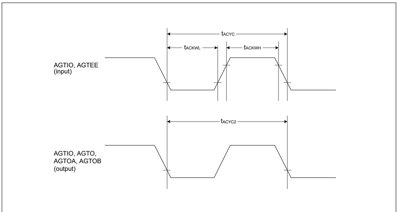
Figure 2.17 AGTW I/O timing
