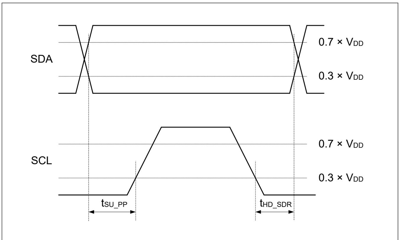
Figure 2.42 Master SDR Timing
