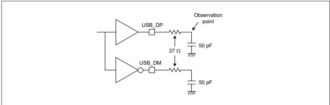
Figure 2.52 Test circuit in full-speed mode
