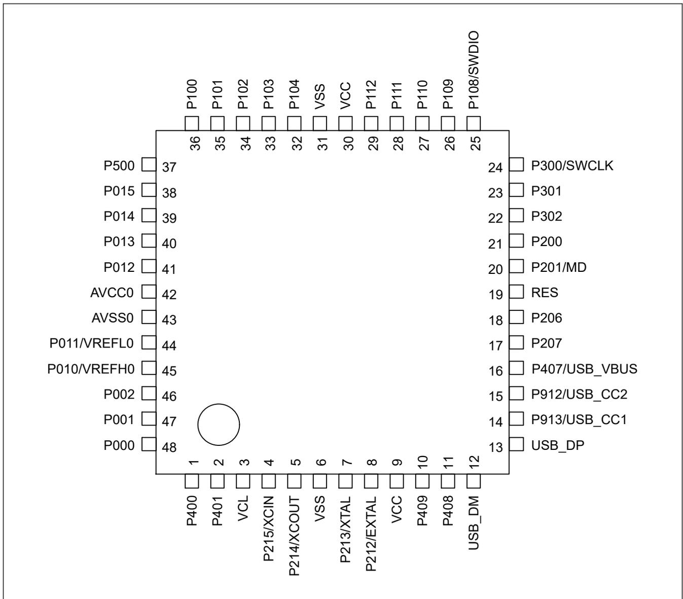
Figure 1.4 Pin assignment for LQFP/QFN 48-pin (top view)
