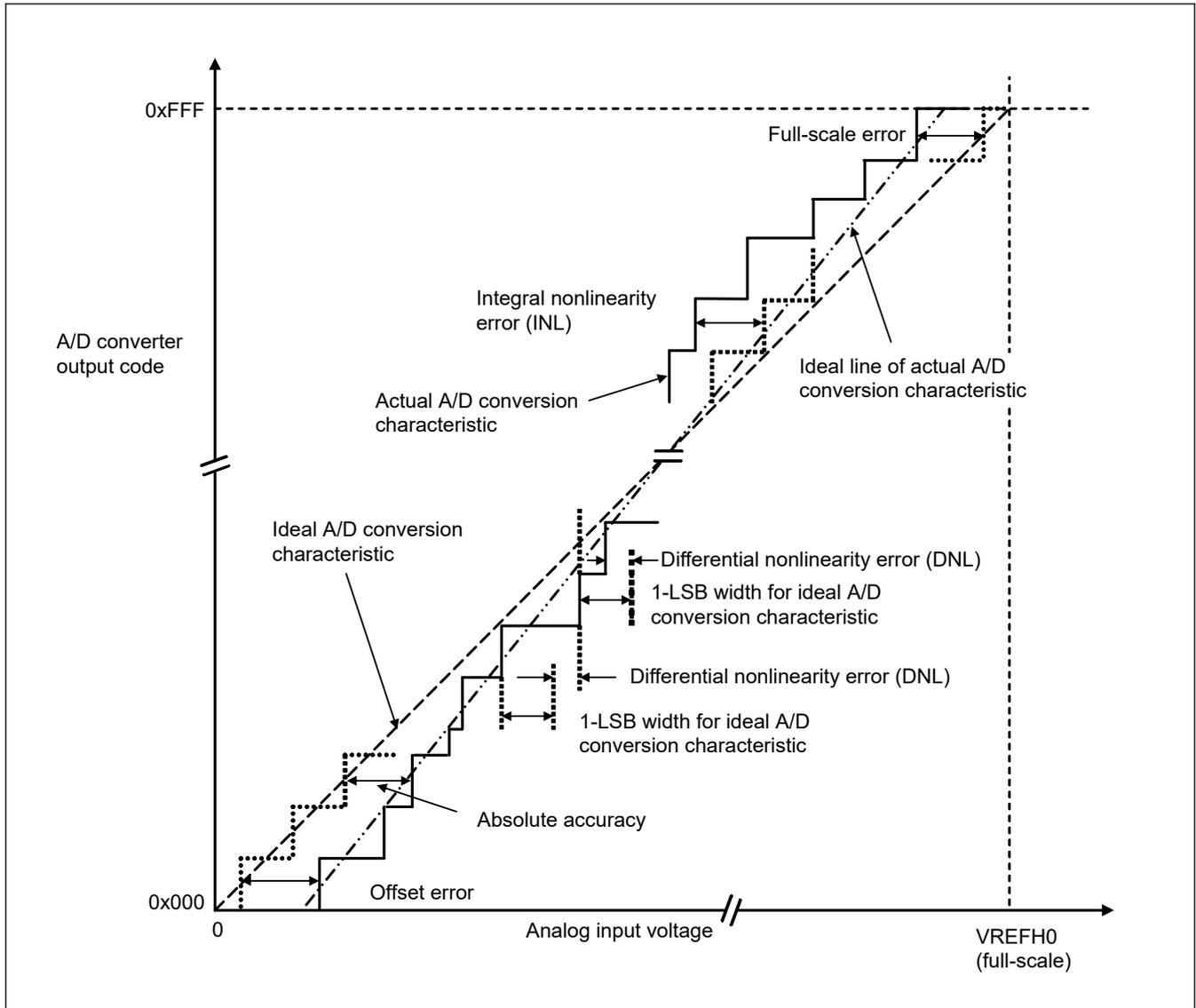
Figure 2.55 Illustration of 12-bit A/D converter characteristic terms
