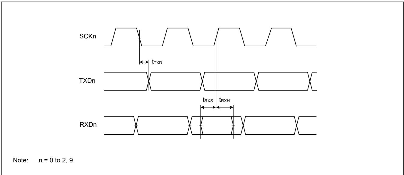
Figure 2.21 SCI input/output timing in clock synchronous mode
