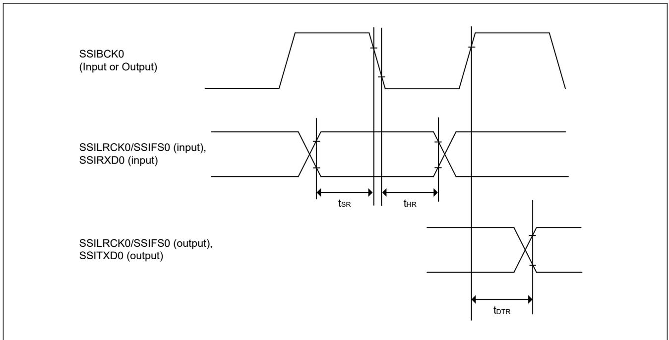
Figure 2.48 SSIE data transmit and receive timing when SSICR.BCKP = 1
