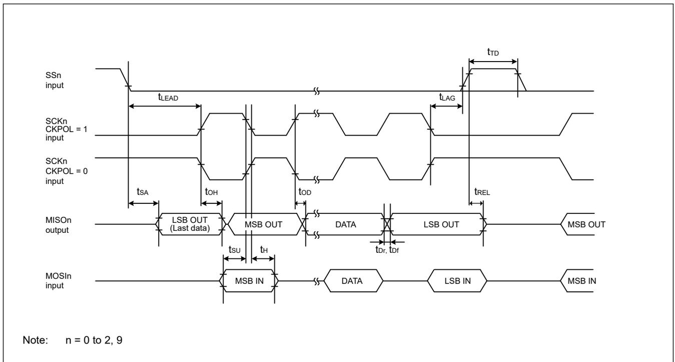
Figure 2.26 SCI simple SPI mode timing (slave, CKPH = 0)
