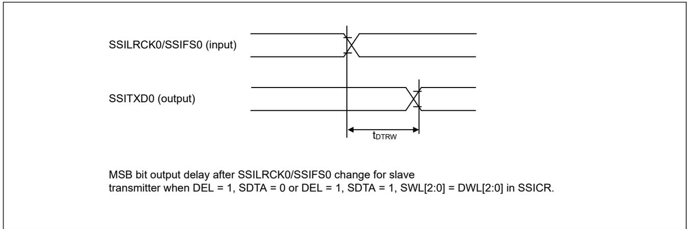
Figure 2.49 SSIE data output delay after SSILRCK0/SSIFS0 change
