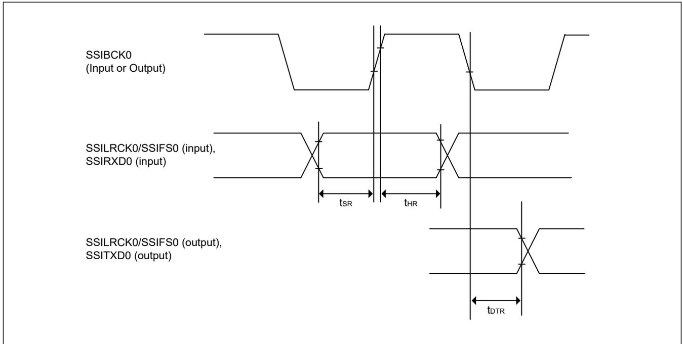
Figure 2.47 SSIE data transmit and receive timing when SSICR.BCKP = 0
