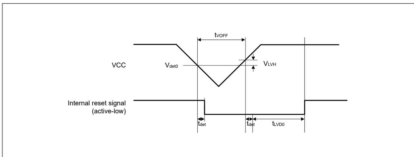
Figure 2.59 Voltage detection circuit timing (V<sub>det0</sub>)
