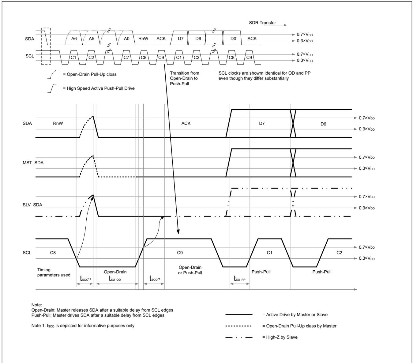
Figure 2.37 I3C Data Transfer – ACK by Slave
