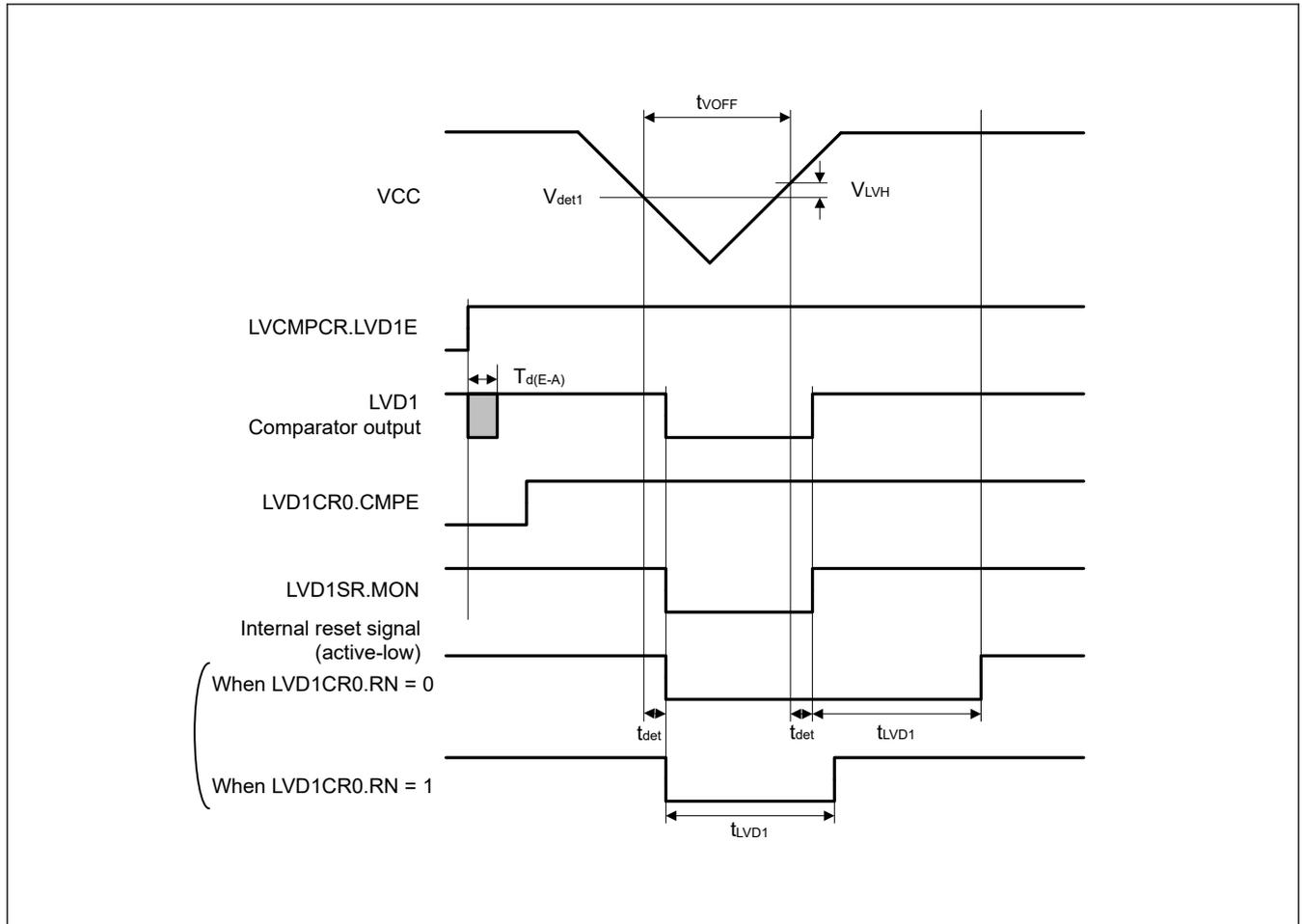
Figure 2.60 Voltage detection circuit timing ( $V_{det1}$ )
