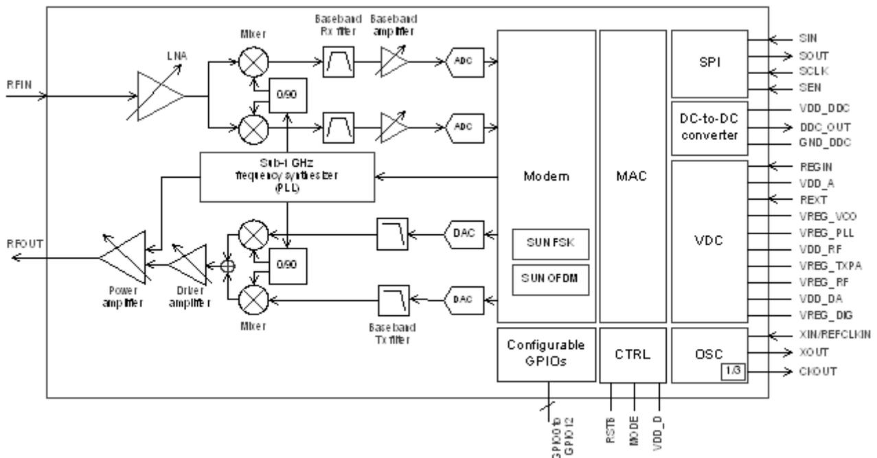
Figure 1-1 Block diagram
