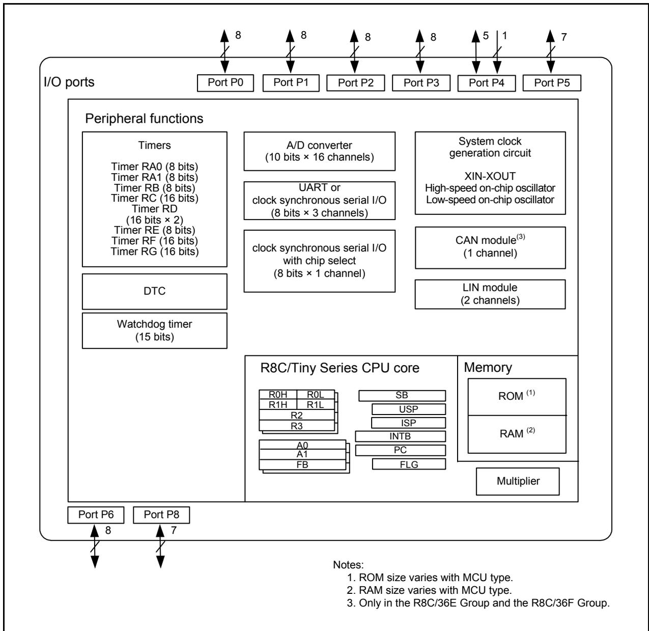
Figure 1.5 Block Diagram
