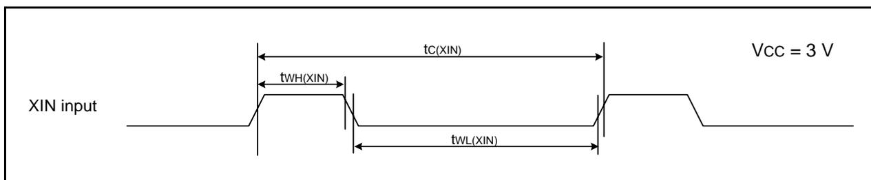
**Figure 5.8 XIN Input Timing Diagram when  $V_{CC} = 3\text{ V}$** **Table 5.23 TRAIO Input**
