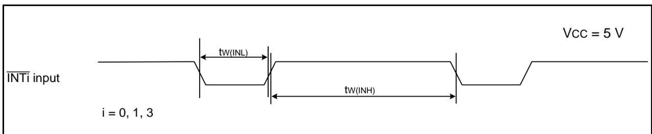
**Figure 5.7 External Interrupt  $\overline{\text{INT}}_i$  Input Timing Diagram when Vcc = 5 V**
