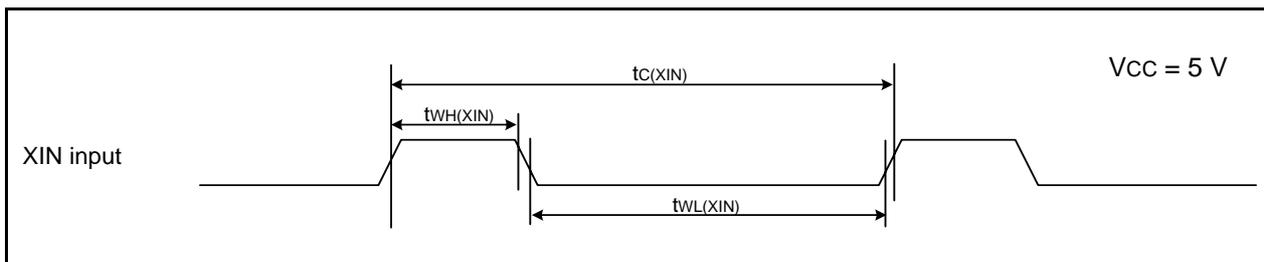
**Figure 5.4 XIN Input Timing Diagram when  $V_{CC} = 5\text{ V}$** **Table 5.17 TRAI0 Input**
