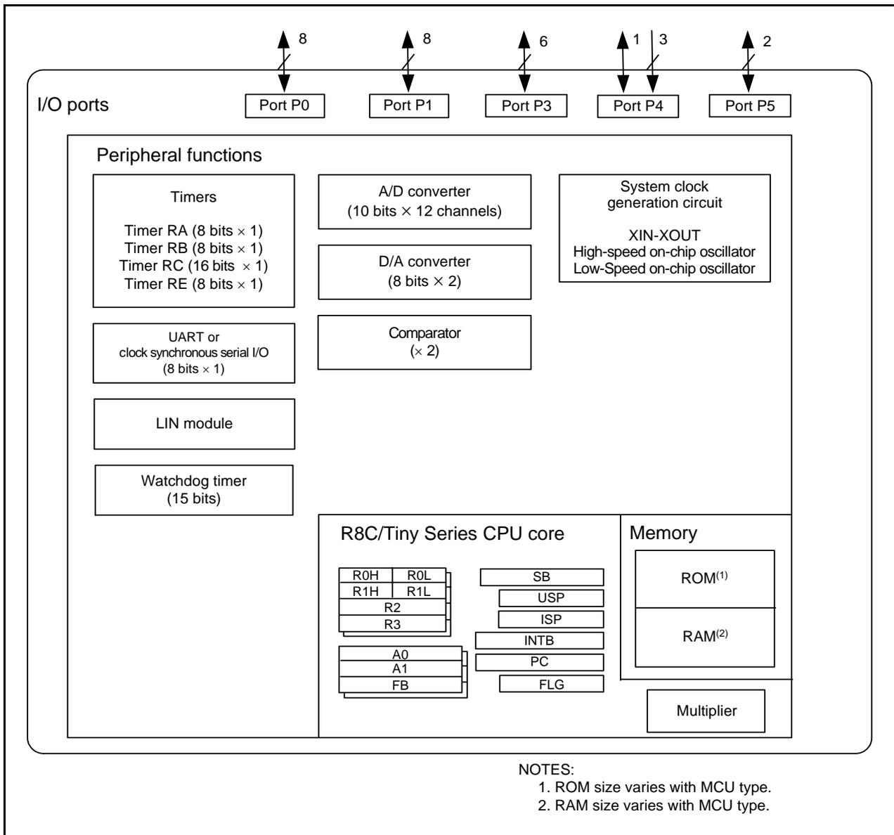
Figure 1.3 Block Diagram
