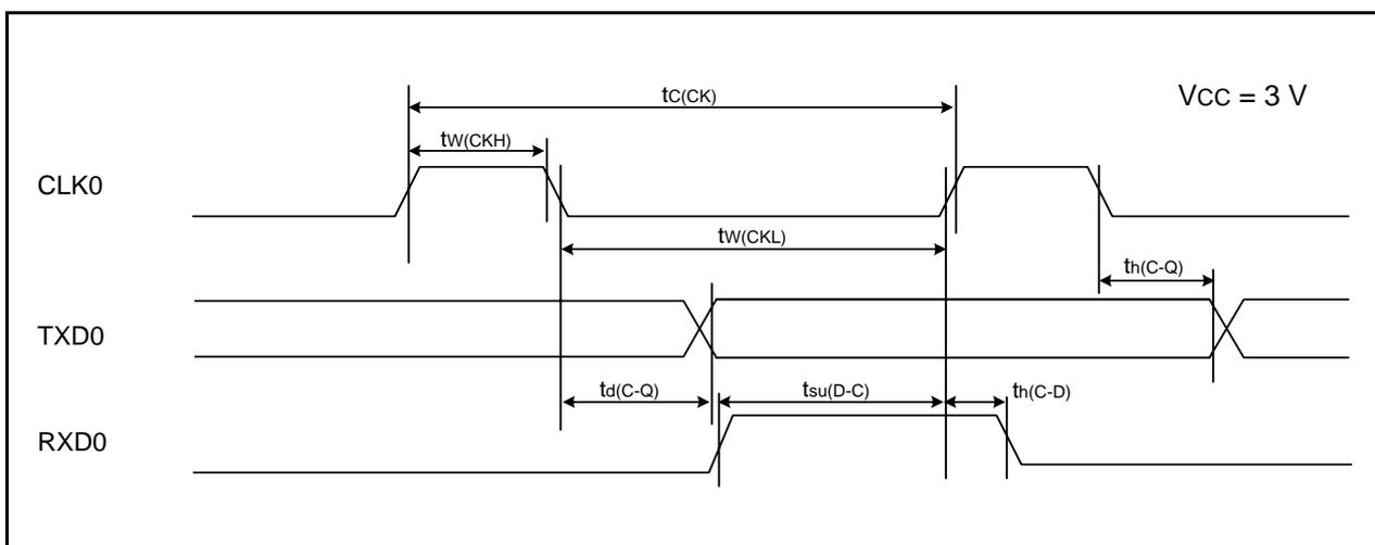
**Figure 5.10 Serial Interface Timing Diagram when Vcc = 3 V**
