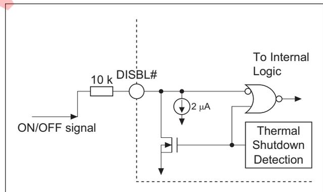
**Figure 5.2 ON/OFF Signal from the System Controller**
