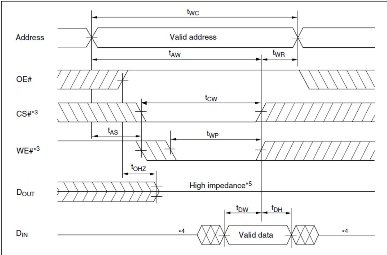
**Write Timing Waveform (2) (CS# Controlled)**
