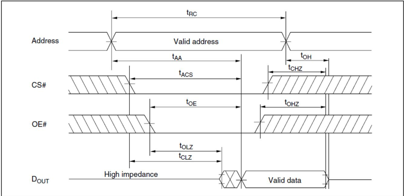
Read Timing Waveform (2) (WE# = V<sub>IH</sub>, LB# = V<sub>IL</sub>, UB# = V<sub>IL</sub>)
