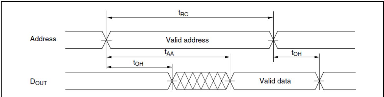
Read Timing Waveform (3) (WE# = V<sub>IH</sub>, CS# = V<sub>IL</sub>, OE# = V<sub>IL</sub>)\*2
