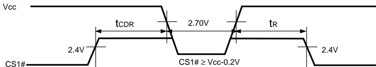
Data Retention timing Waveform (3) (CS2 Controlled)
