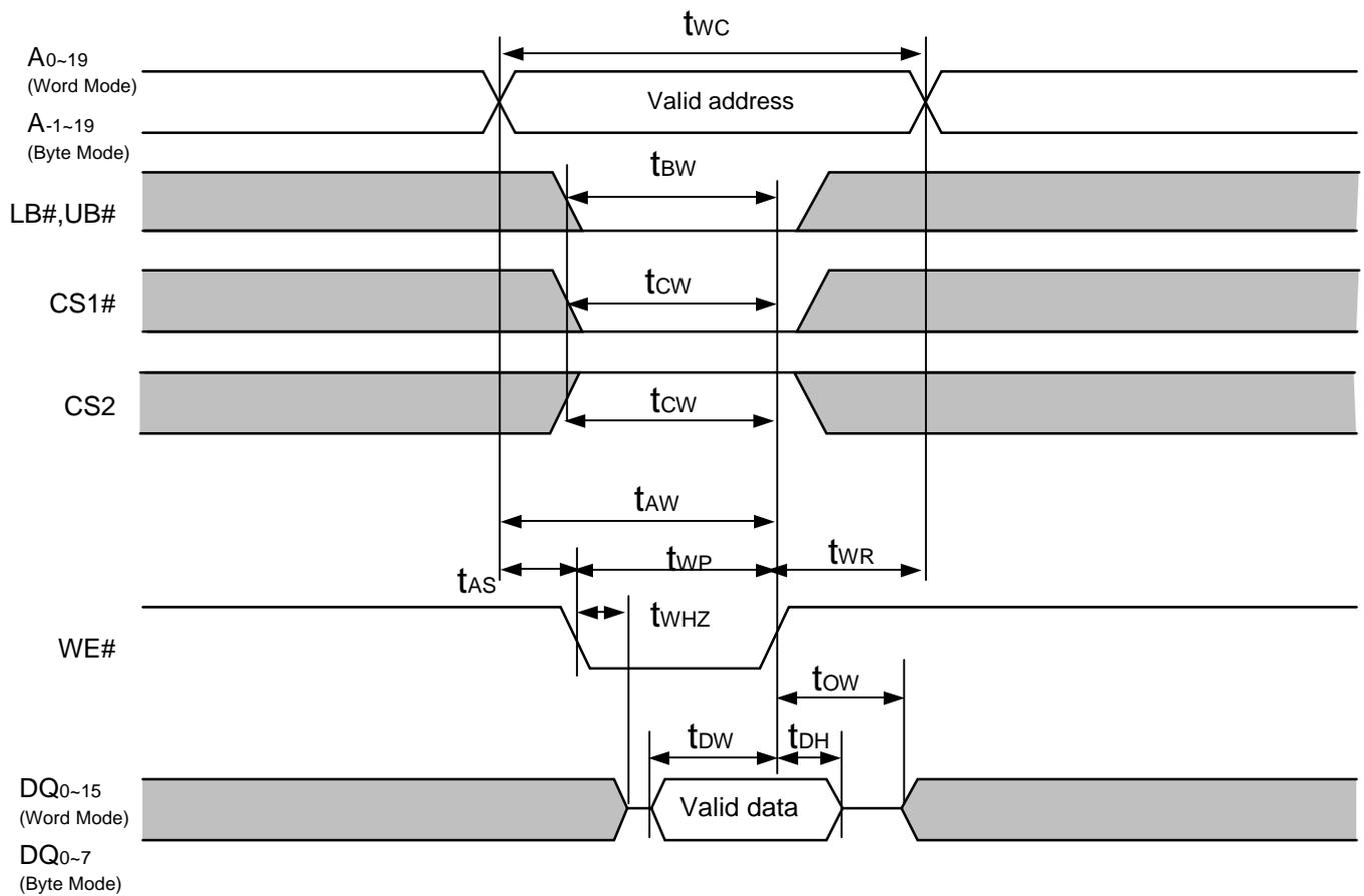
Write Cycle (2) (CS1# ,CS2 Clock, OE#=V<sub>IH</sub>)
