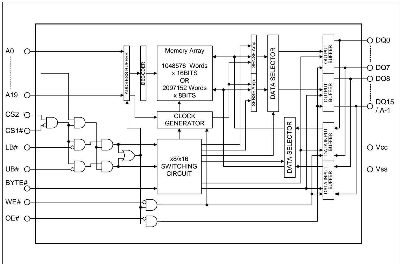
Note. BYTE# pin supported by only TSOP and uTSOP types.
