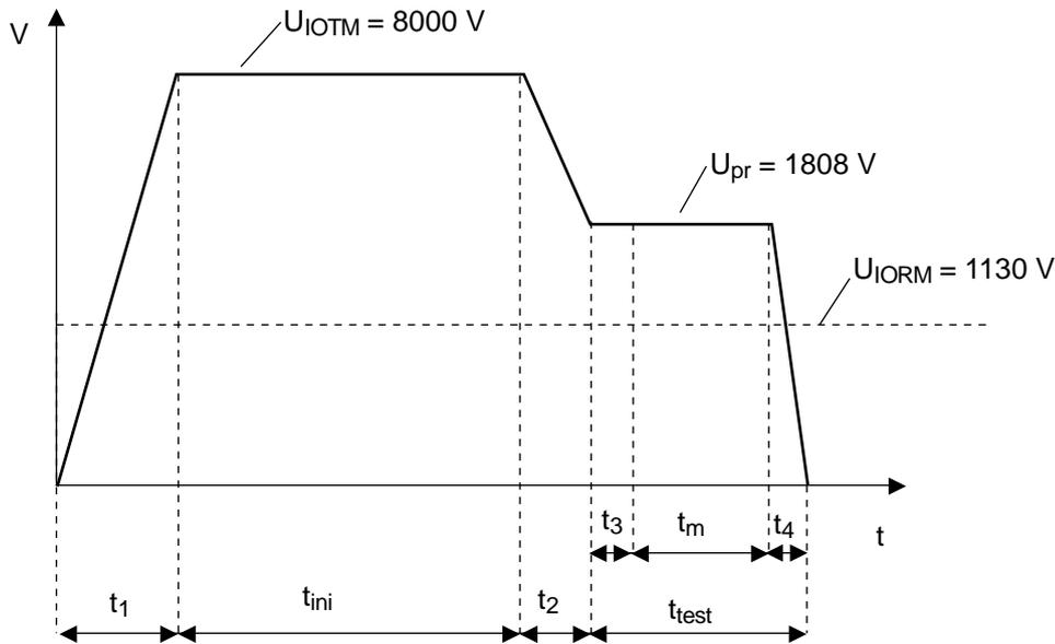
$t_1, t_2 = 1\text{ to }10\text{ sec}$
