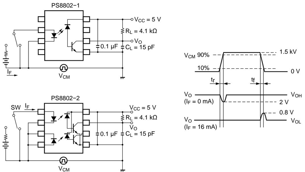
Remark: C<sub>L</sub> includes probe and stray wiring capacitance.
