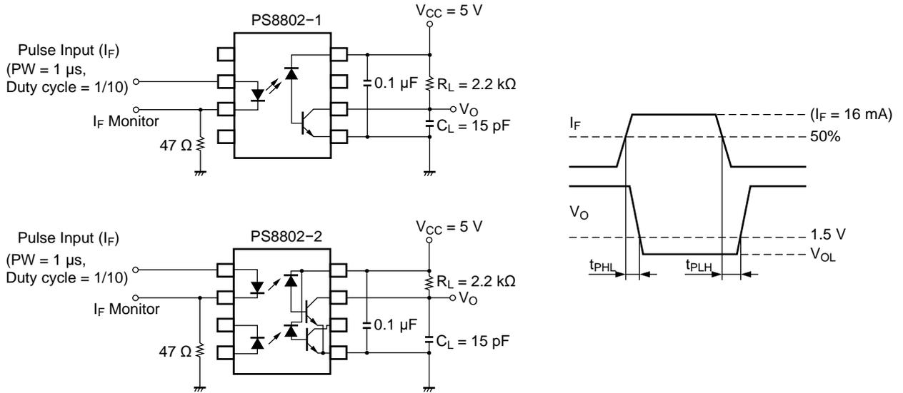
Remark: C<sub>L</sub> includes probe and stray wiring capacitance.
