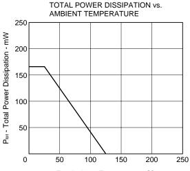
T<sub>A</sub> - Ambient Temperature - °C
