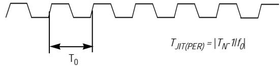
The deviation in cycle time of a signal with respect to the ideal period over a random sample of cycles
