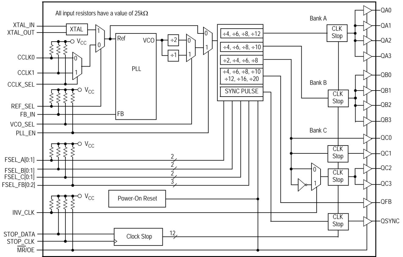
Figure 1. Logic Diagram
