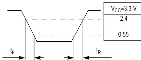
**Figure 22. Output Transition Time Test Reference**
