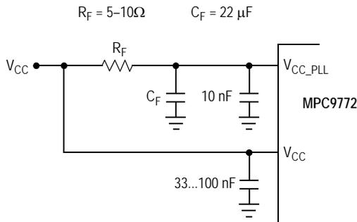
**Figure 7. V<sub>CC\_PLL</sub> Power Supply Filter**
