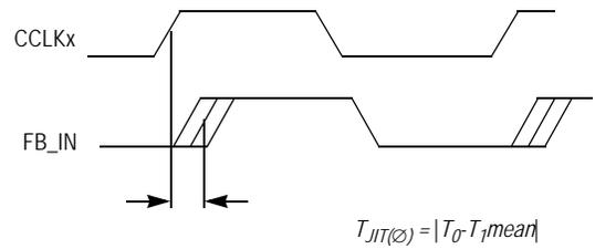
The deviation in  $t_0$  for a controlled edge with respect to a  $t_0$  mean in a random sample of cycles
