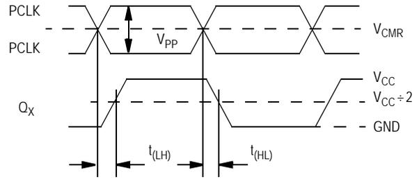
Figure 8. Propagation Delay ( $t_{PD}$ ) Test Reference
