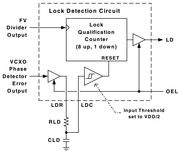
If the lock detection circuit is not used, the LDR output may remain unconnected, however the LDC input should be tied high or low. If the PCB was designed to accommodate the RLD and CLD components but the LD output will not be used, RLD can remain unpopulated and CLD can be replaced with a resistor (< 10 kohm).
