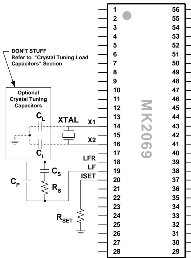
$C_P$  establishes a second pole in the VCXO PLL loop filter. For higher damping factors ( $> 1$ ), calculate the value of  $C_P$  based on a  $C_S$  value that would be used for a damping factor of 1. This will minimize baseband peaking and loop instability that can lead to output jitter.
