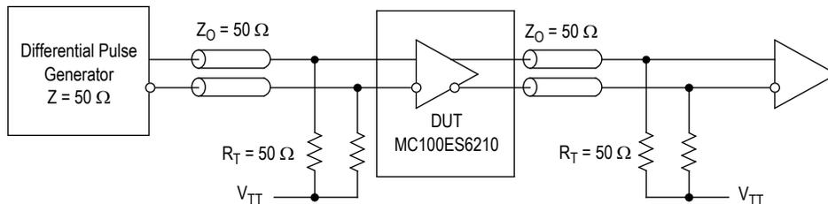
**Figure 4. MC100ES6210 AC Test Reference**
