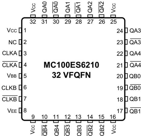
Figure 3. 32-Lead VFQFN Package Pinout (Top View)
