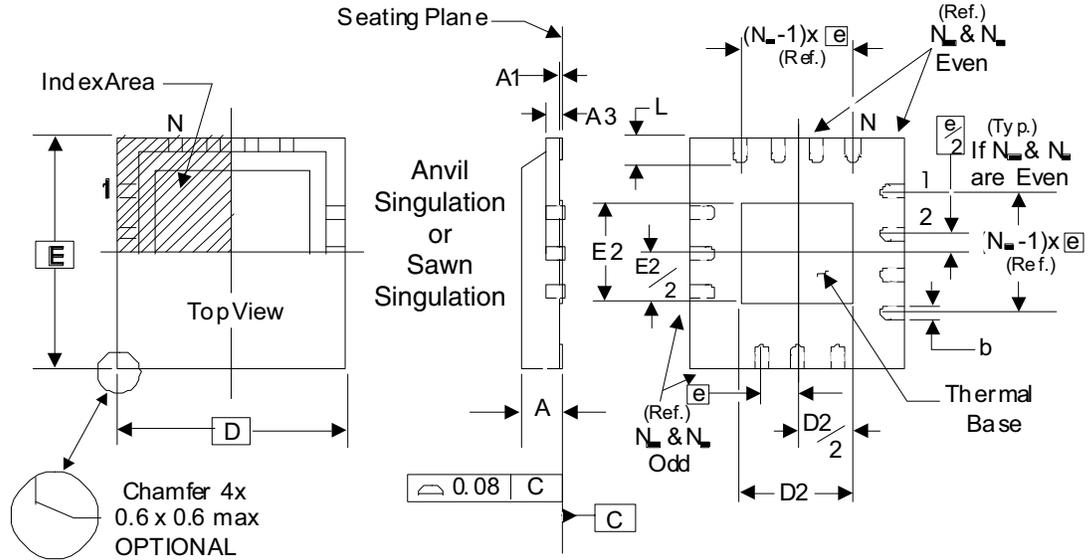
NOTE: The following package mechanical drawing is a generic drawing that applies to any pin count VFQFN package. This drawing is not intended to convey the actual pin count or pin layout of this device. The pin count and pinout are shown on the front page. The package dimensions are in Table 7 below.
