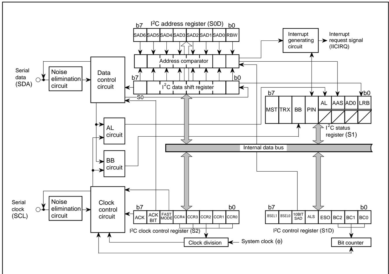
Fig. 8.6.1 Block Diagram of Multi-master I<sup>2</sup>C-BUS Interface
