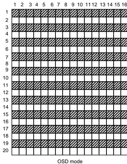
When the display dot line selection bit is "0," the "  " font is displayed at even field, the "  " font is displayed at odd field. Bit 6 of the I/O polarity control register can be read as the field determination flag : "1" is read at odd field, "0" is read at even field.
