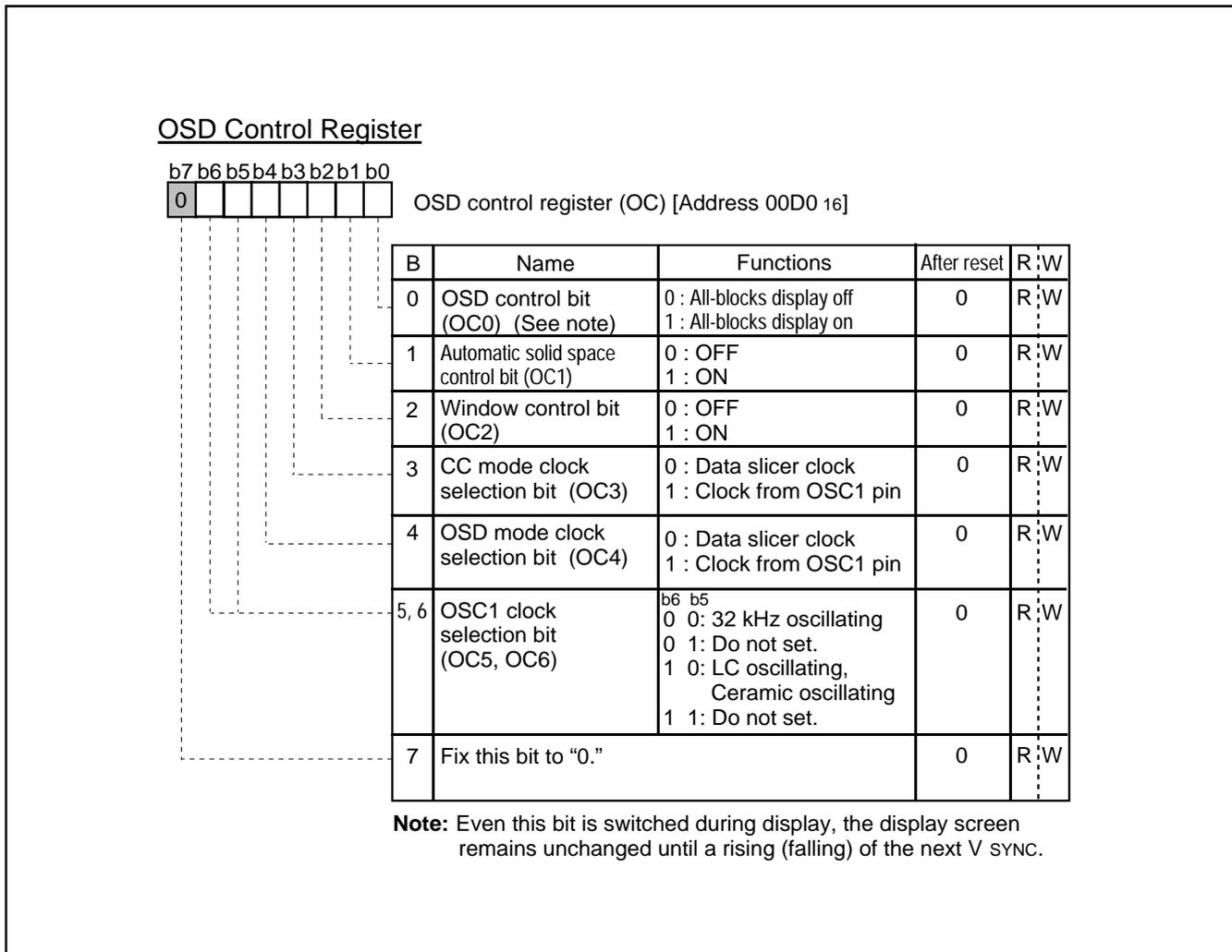
**Note:** Even this bit is switched during display, the display screen remains unchanged until a rising (falling) of the next V SYNC.
