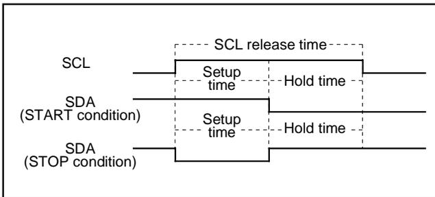
**Fig. 8.6.11 START Condition/STOP Condition Detect Timing Diagram**
