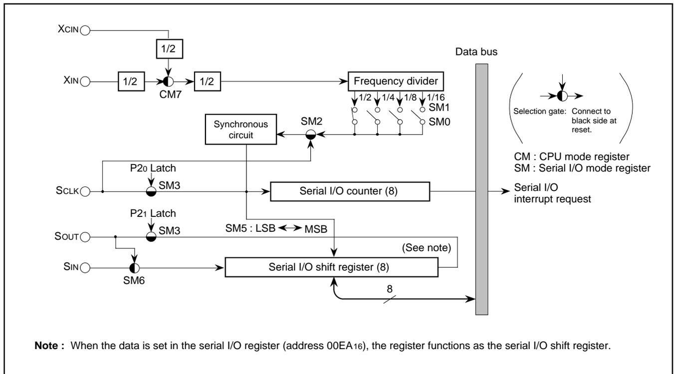
Fig. 8.5.1 Serial I/O Block Diagram
