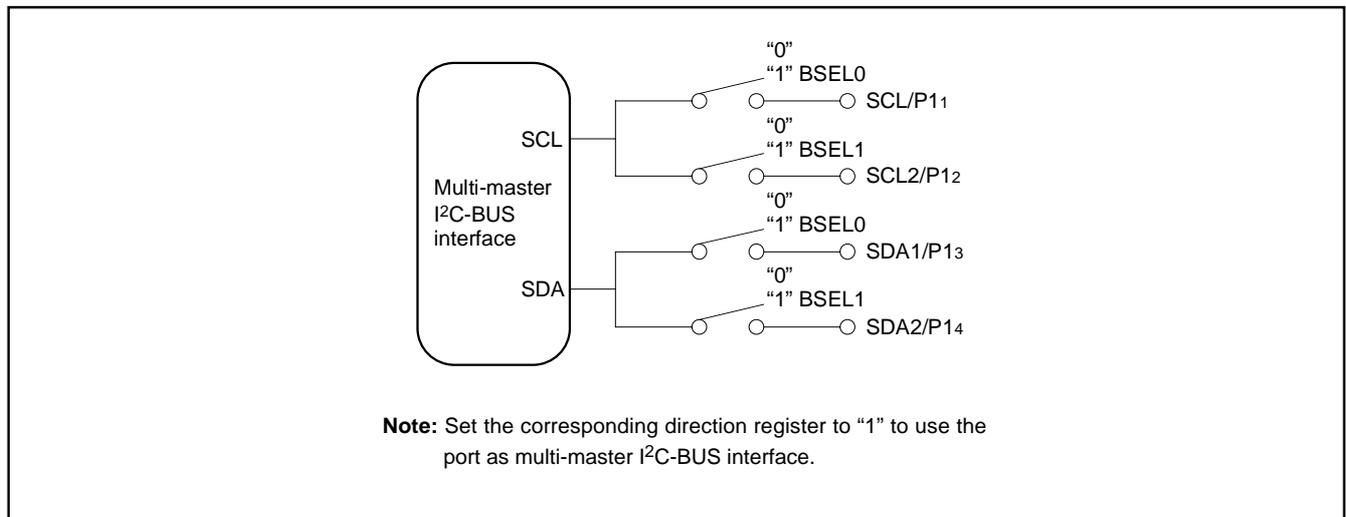
Fig. 8.6.5 Connection Port Control by BSEL0 and BSEL1
