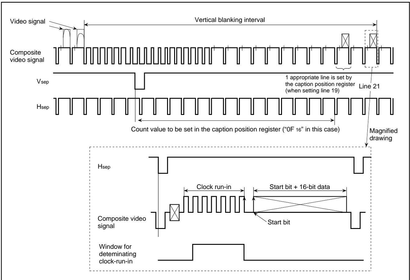
Fig. 8.10.8 Signals in Vertical Blanking Interval
