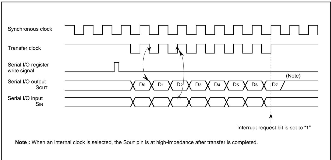
Fig. 8.5.2 Serial I/O Timing (for LSB first)
