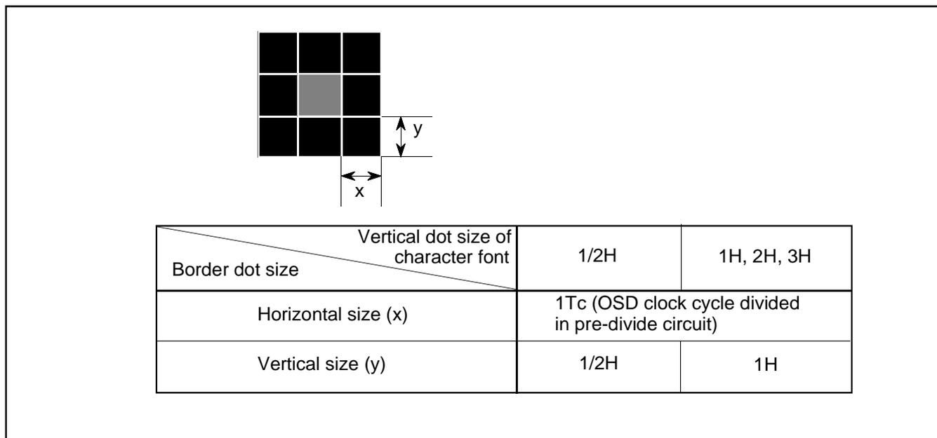
Fig. 8.11.21 Horizontal and Vertical Size of Border
