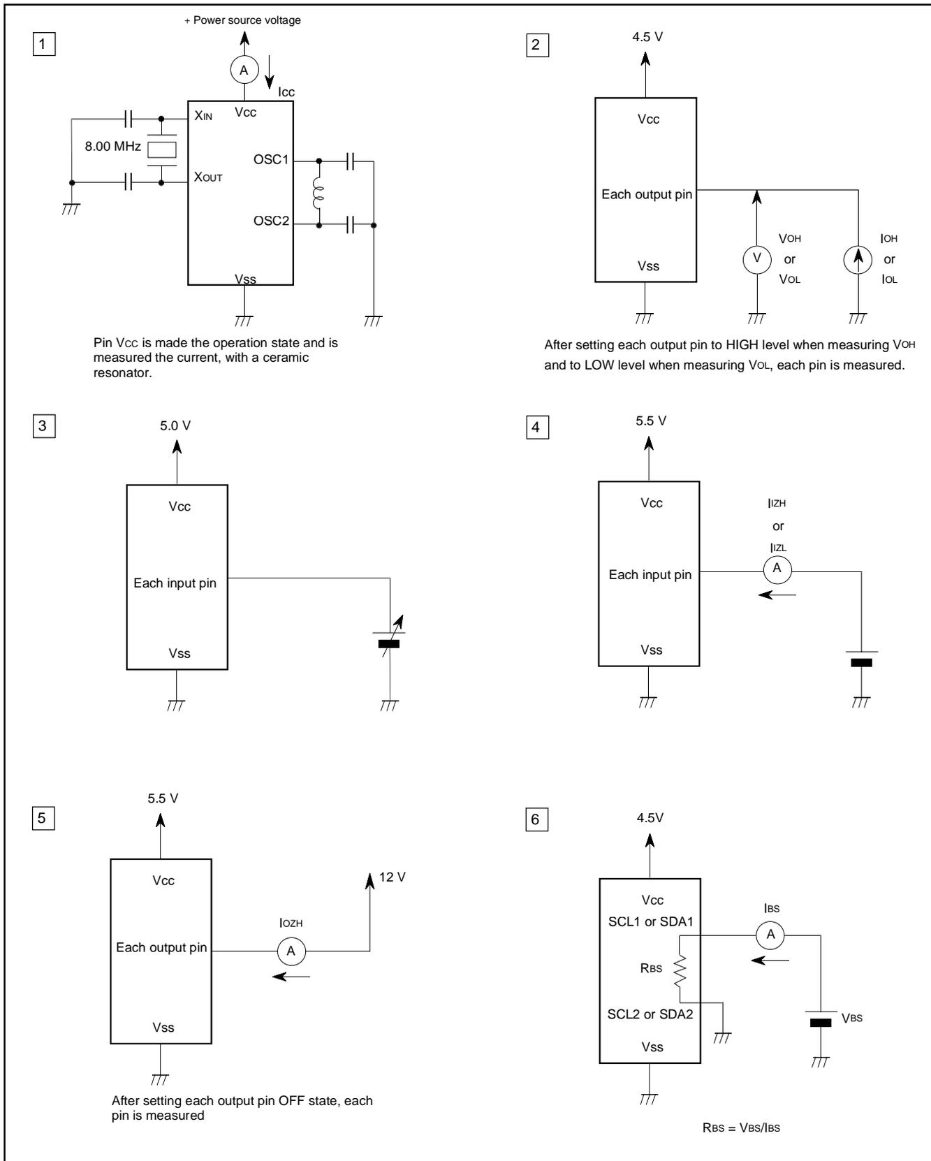
Fig.12.1 Measure Circuits
