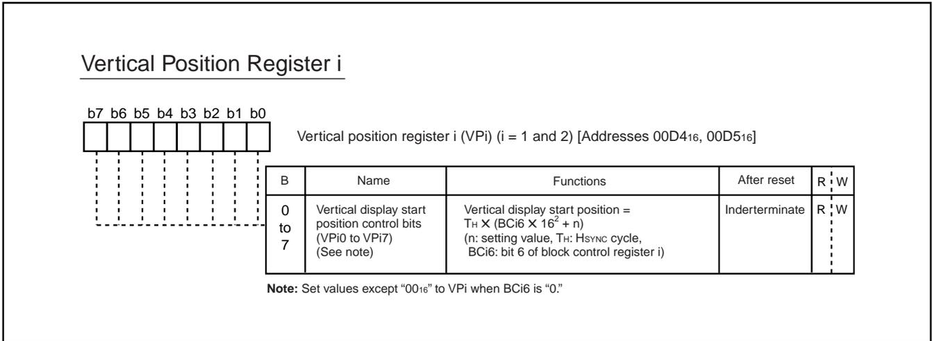
Fig. 8.11.7 Vertical Position Register i (i = 1 and 2)
