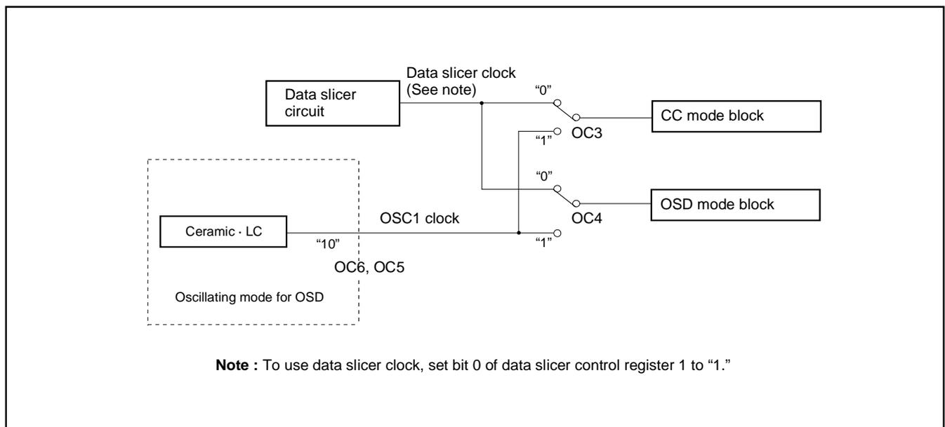
**Fig. 8.11.12 Block Diagram of OSD Selection Circuit**
