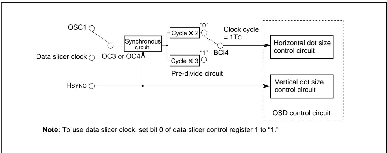
Fig. 8.11.10 Block Diagram of Dot Size Control Circuit
