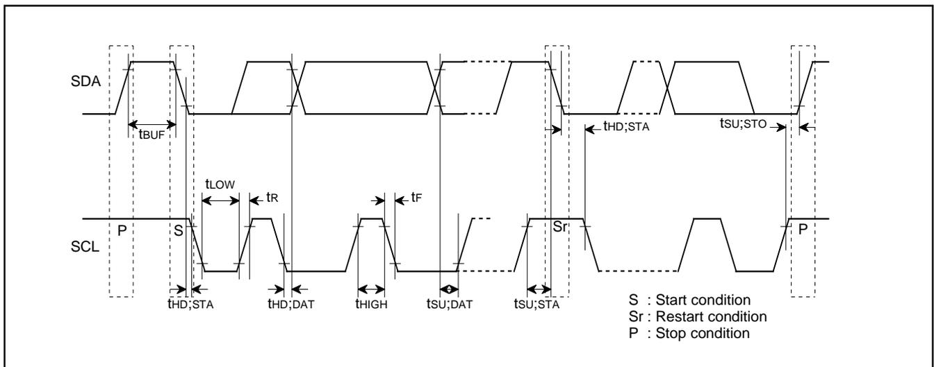
Fig.14.1 Definition Diagram of Timing on Multi-master I<sup>2</sup>C-BUS
