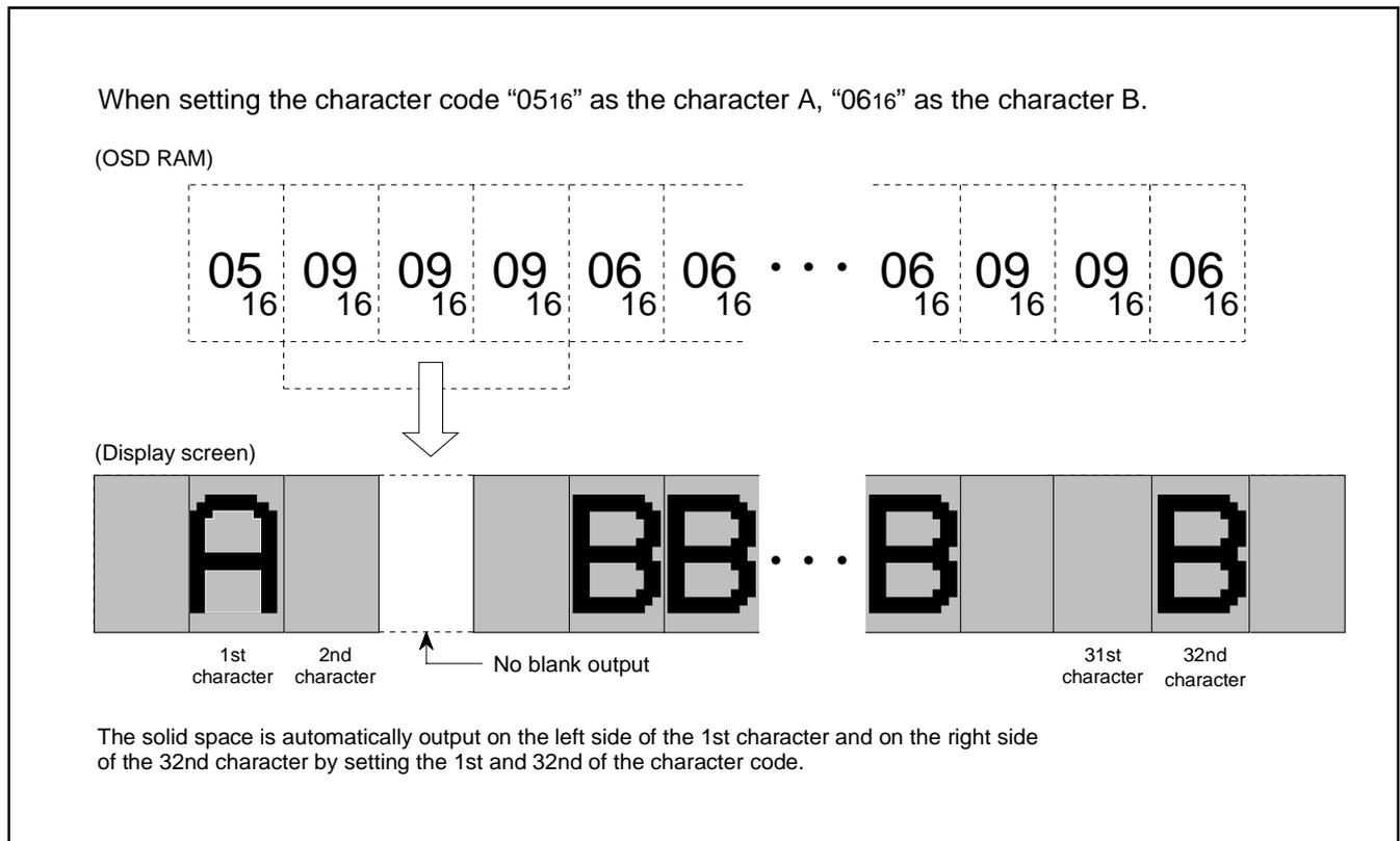
Fig. 8.11.24 Display Screen Example of Automatic Solid Space
