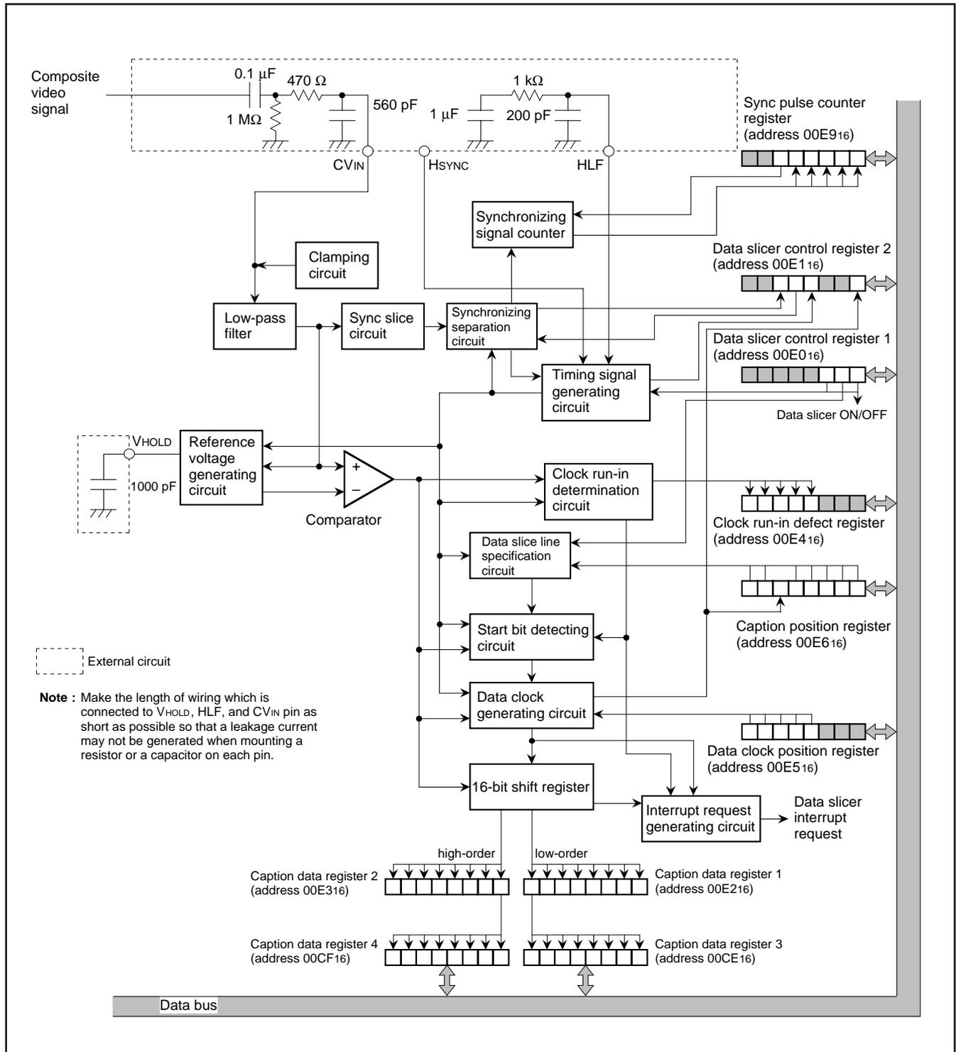
Fig. 8.10.1 Data Slicer Block Diagram
