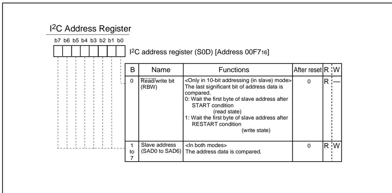
Fig. 8.6.3 I<sup>2</sup>C Address Register
