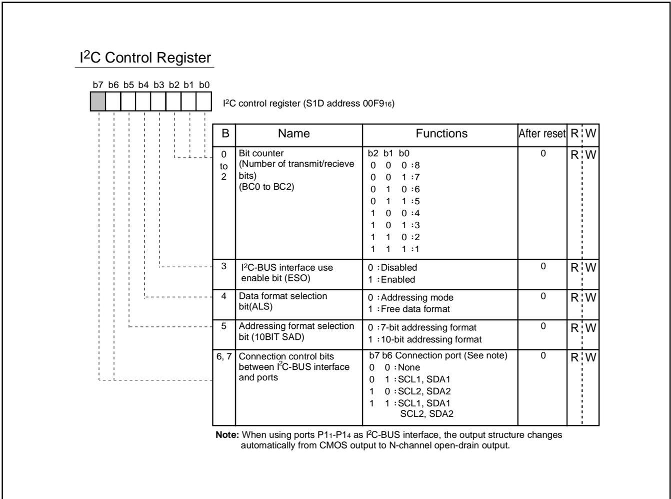
Fig. 8.6.6 I<sup>2</sup>C Control Register
