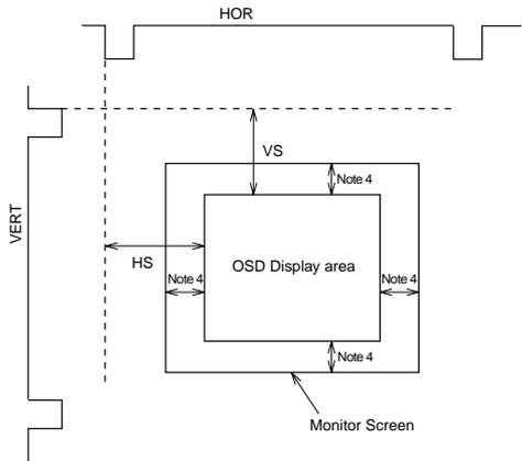
HS\* (shown left) shows horizontal display start location that is register B/F (address 128<sub>16</sub>) = 0 is set.
