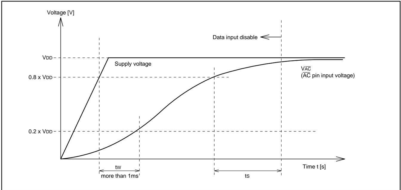
Fig. 19 Timing of power supplying to  $\overline{AC}$  pin
