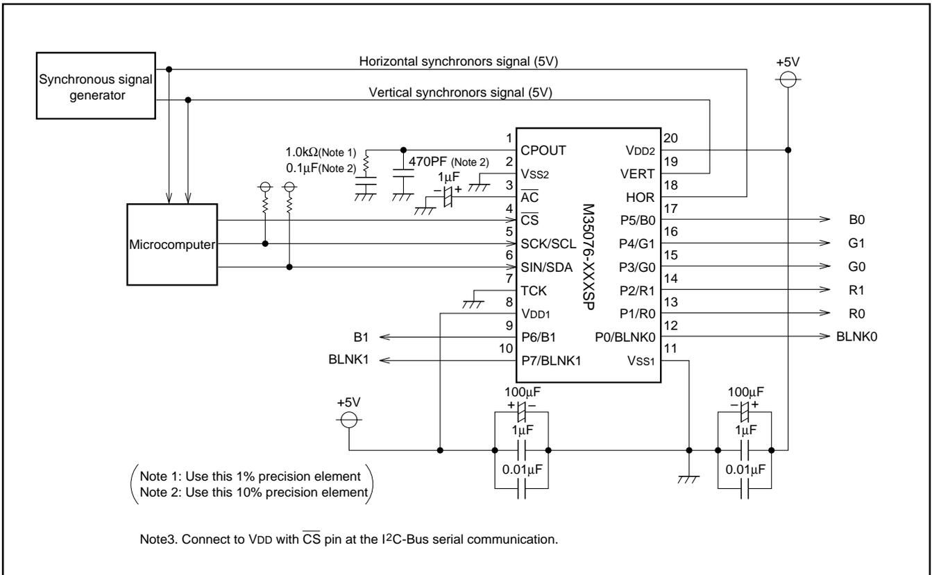
Fig 11. Example of the M35076-XXXSP peripheral circuit ( Internal clock mode. At EXCK1 = "0", EXCK0 = "1")
