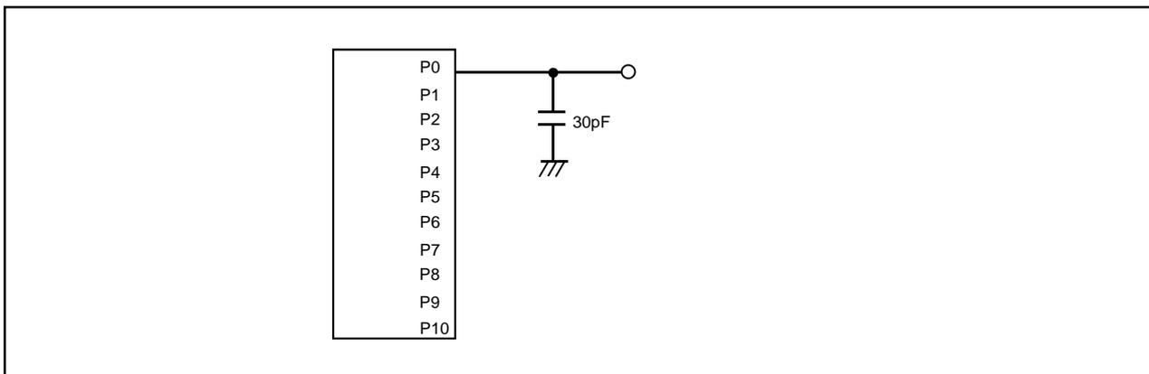
Figure 1.26.1. Port P0 to P10 measurement circuit
