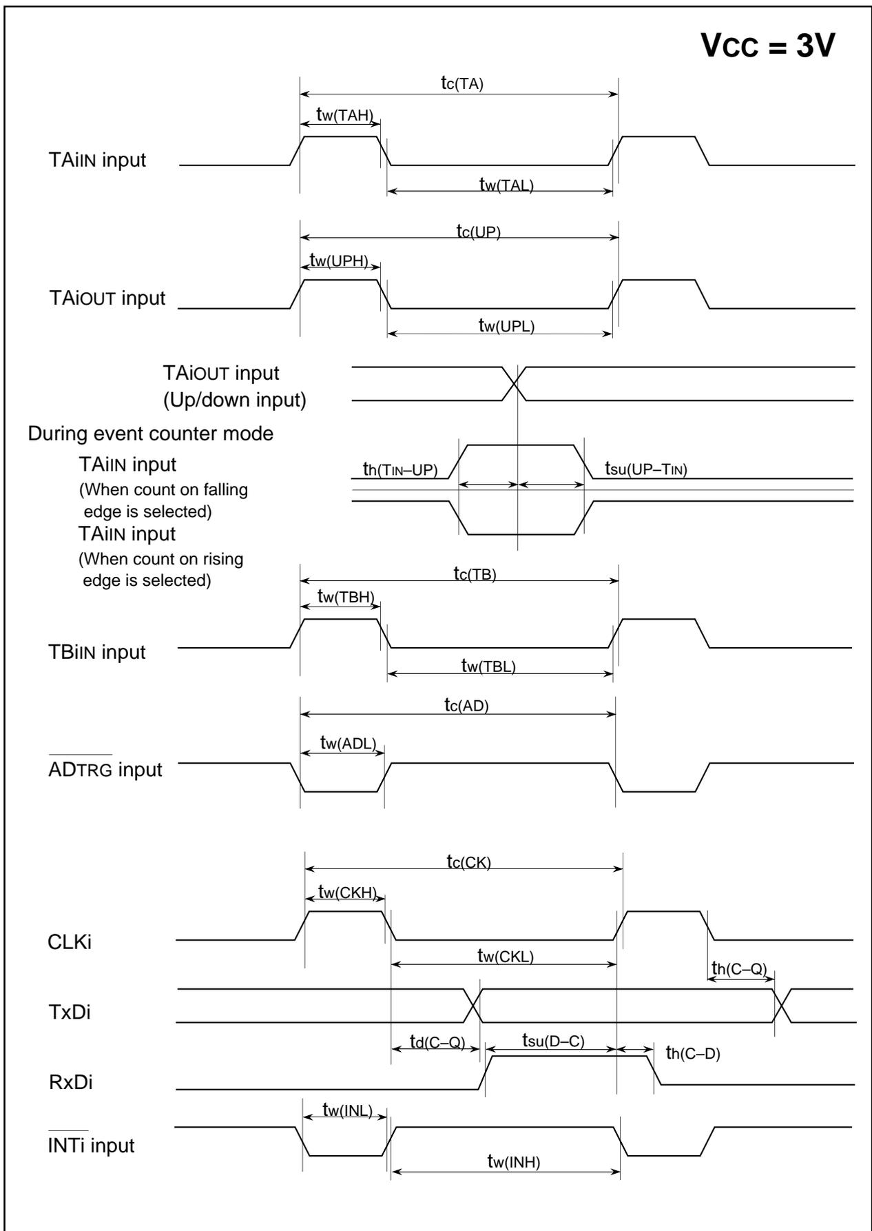
Figure 1.26.2. V<sub>CC</sub>=3V timing diagram (1)
