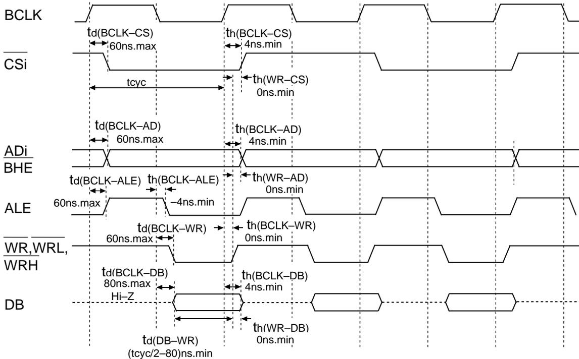
Figure 1.26.4. V<sub>CC</sub>=3V timing diagram (3)
