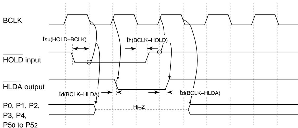
Note: The above pins are set to high-impedance regardless of the input level of the BYTE pin and bit (PM06) of processor mode register 0 selects the function of ports P40 to P43.
