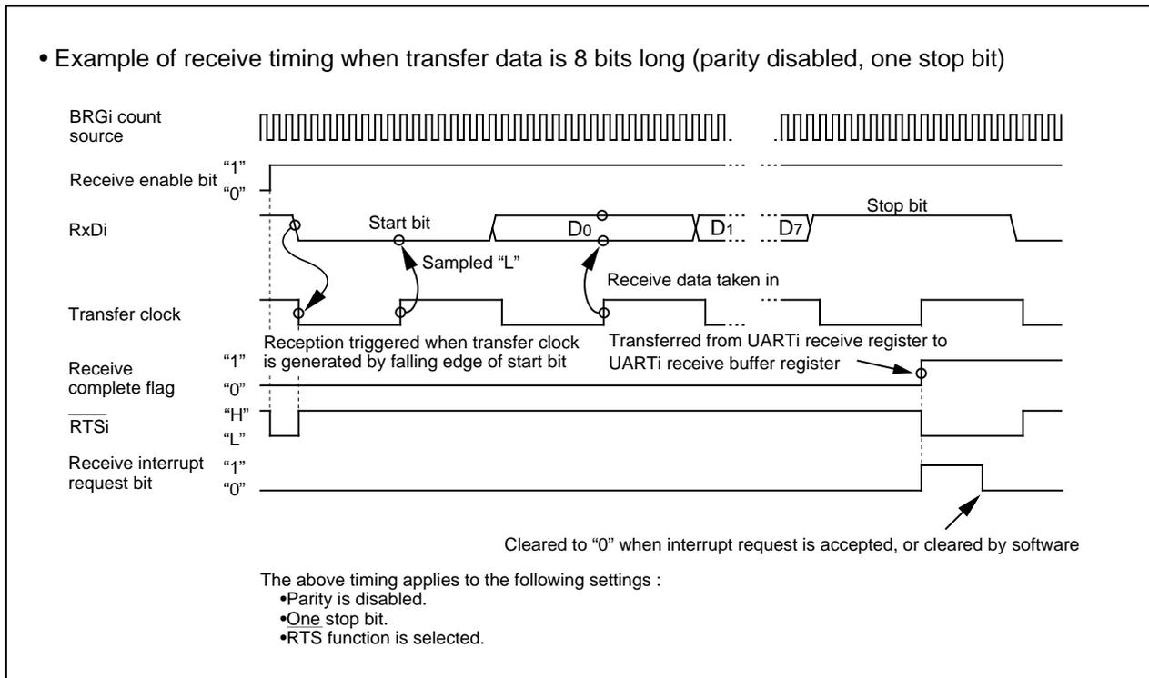
Figure 1.16.19. Typical receive timing in UART mode
