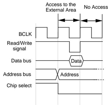
Note : These examples show the address bus and chip select signal within the successive two cycles. According to the combination of these examples, the chip select can be elongated to over 2cycles.
