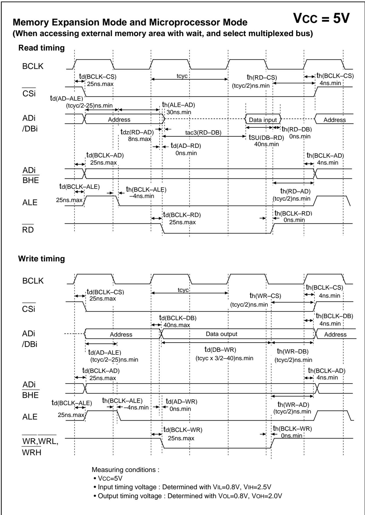
Figure 1.23.6. Vcc = 5V timing diagram (5)
