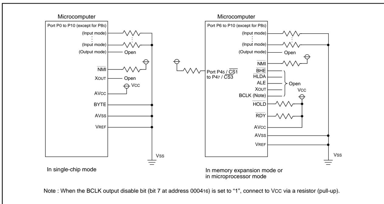
**Figure 1.20.10. Example connection of unused pins**
