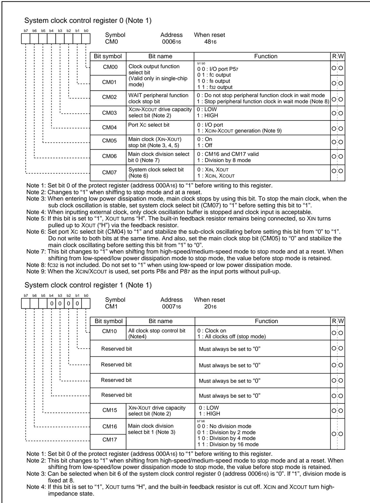
Figure 1.10.4. Clock control registers 0 and 1
