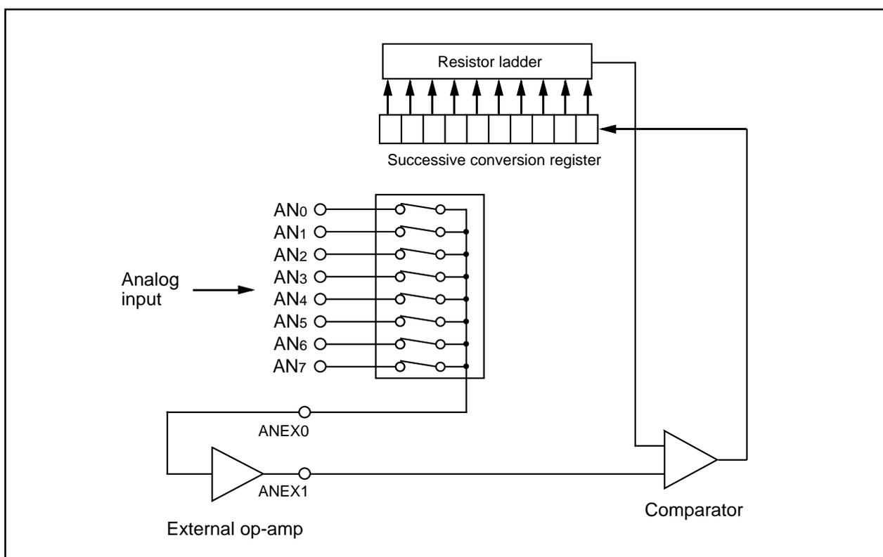
Figure 1.17.5. Example of external op-amp connection mode
