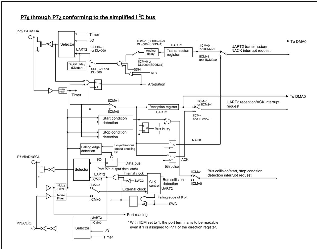
Figure 1.16.30. Functional block diagram for I<sup>2</sup>C mode
