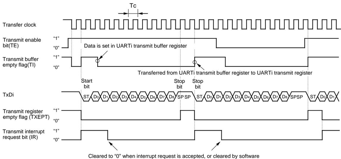
Figure 1.16.17. Typical transmit timings in UART mode(UART0,UART1)
