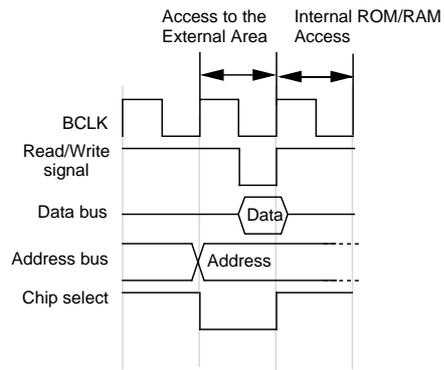
Example 3) After access the external area, only the address bus changes in the next cycle (the chip select signal does not change).
