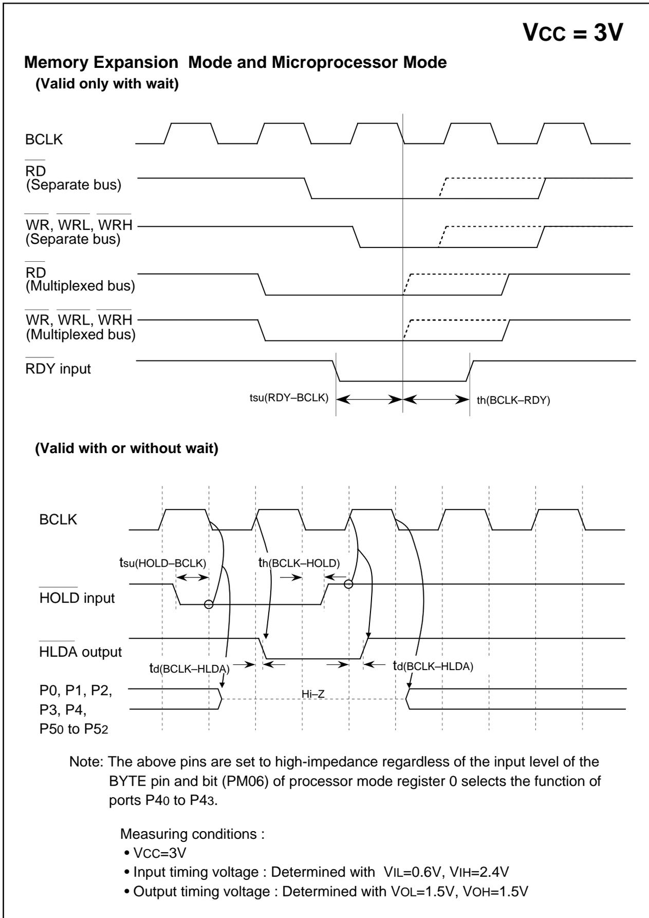
Figure 1.23.9.  $V_{CC} = 3V$  timing diagram (2)
