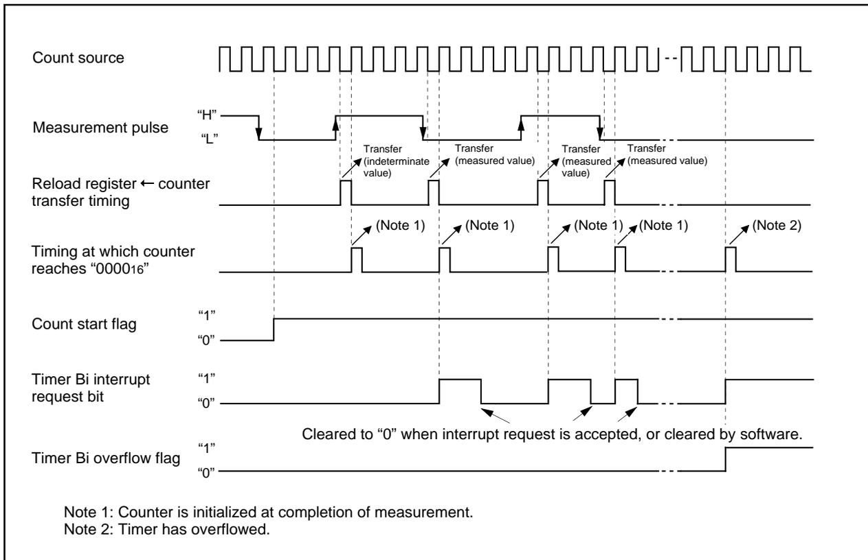
Figure 1.14.21. Operation timing when measuring a pulse width
