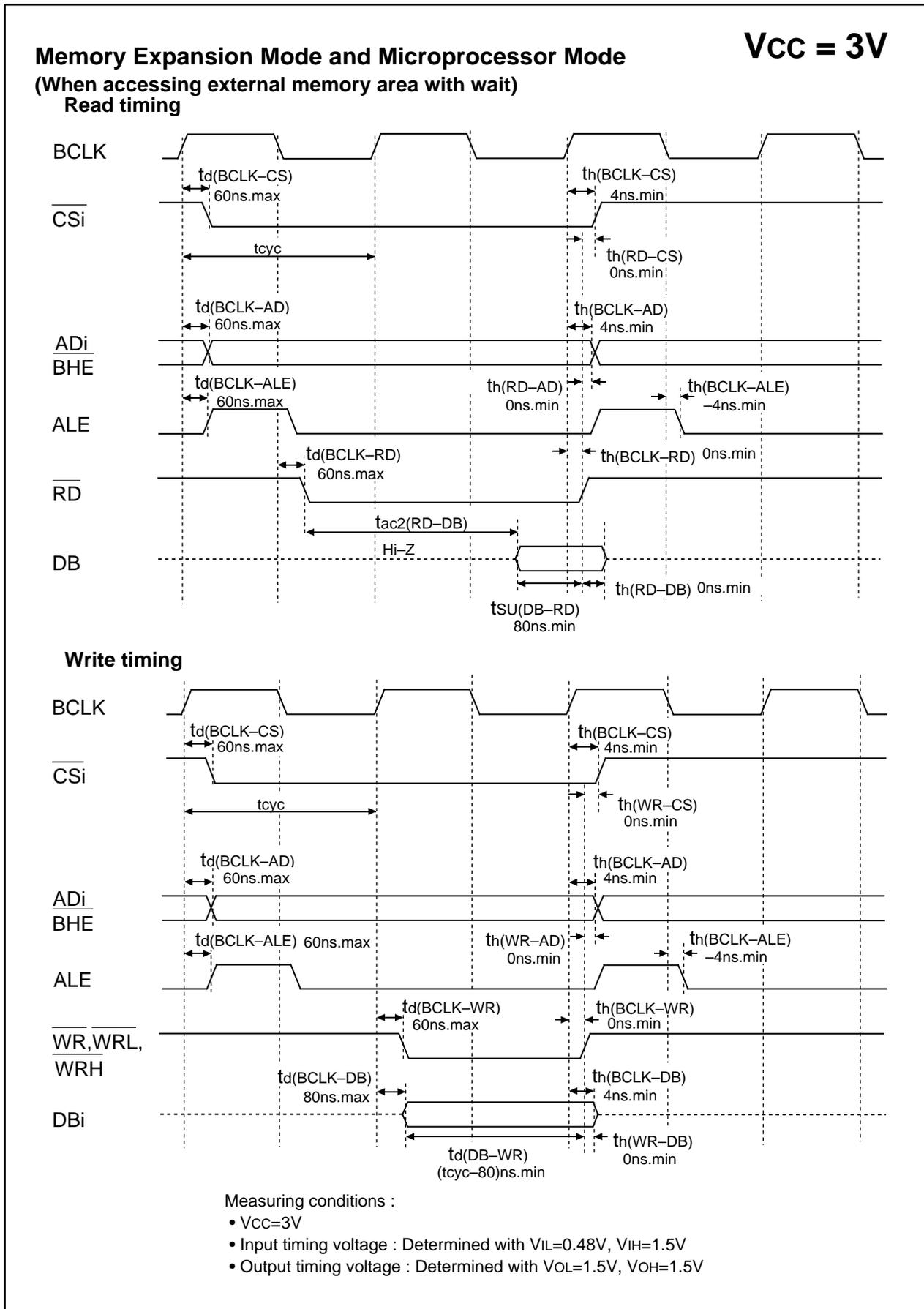
Figure 1.23.11. Vcc = 3V timing diagram (4)
