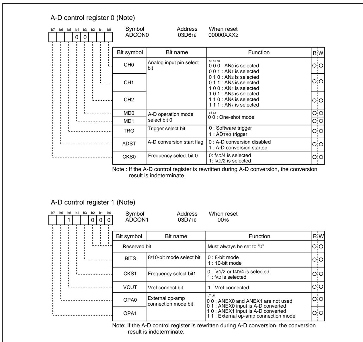
Figure 1.17.4. A-D conversion register in one-shot mode
