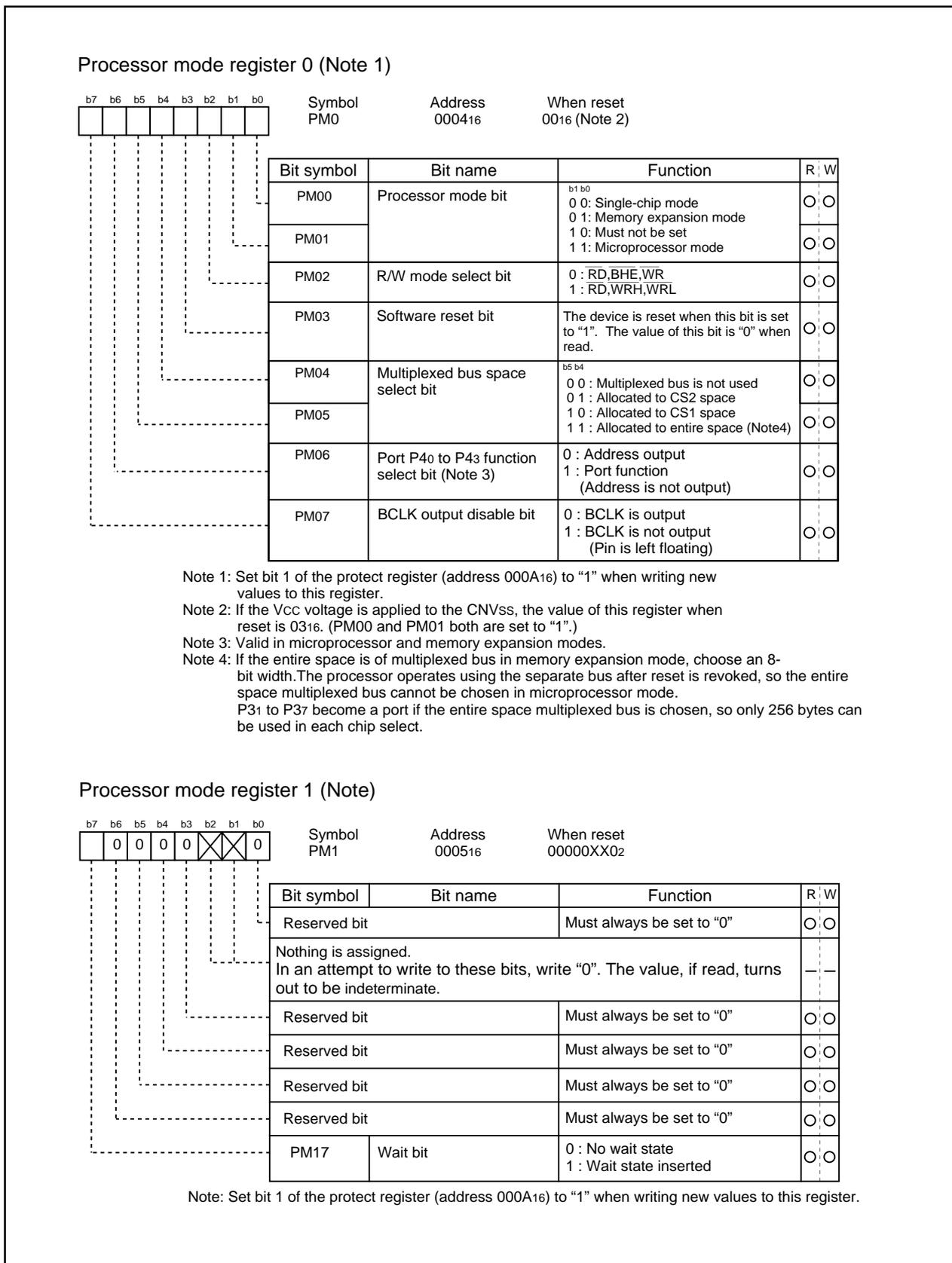
Figure 1.7.1. Processor mode register 0 and 1
