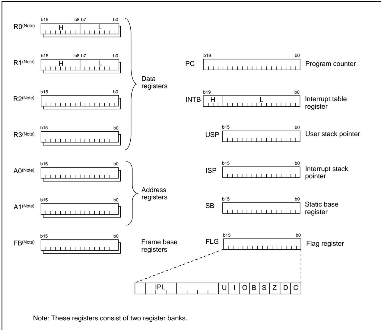
Figure 1.4.1. Central processing unit register
