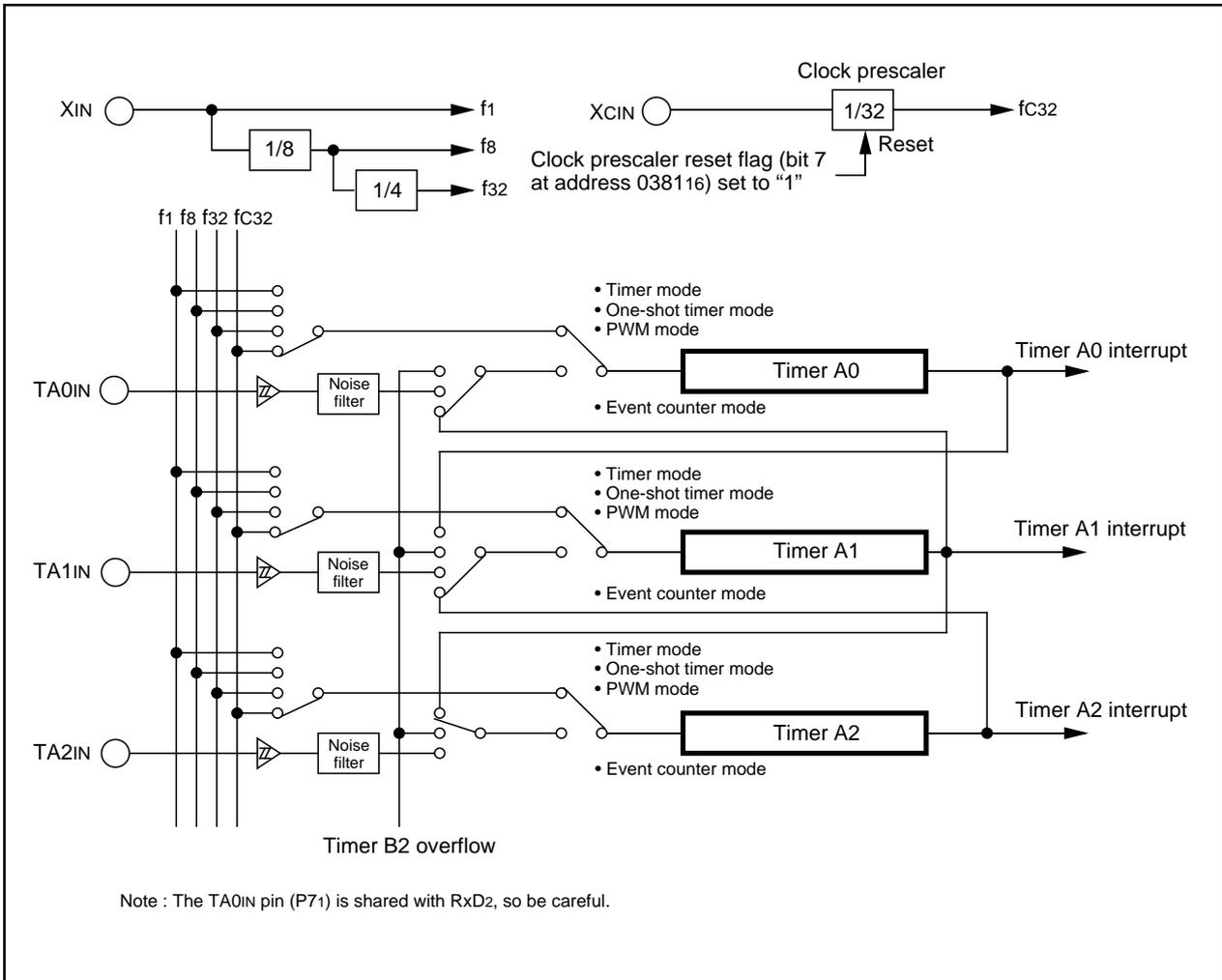
Figure 1.14.1. Timer A block diagram
