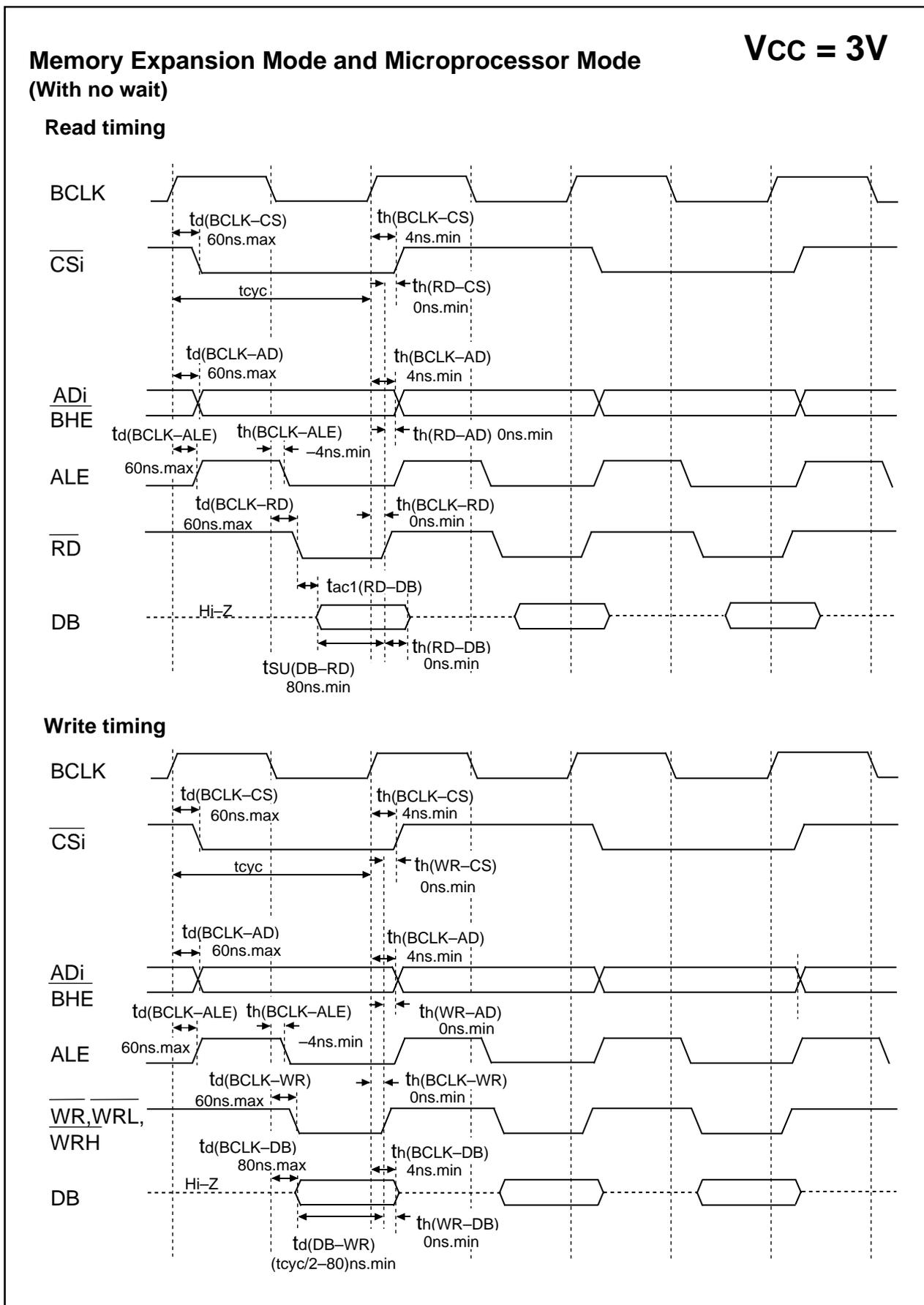
Figure 1.23.10.  $V_{CC} = 3V$  timing diagram (3)
