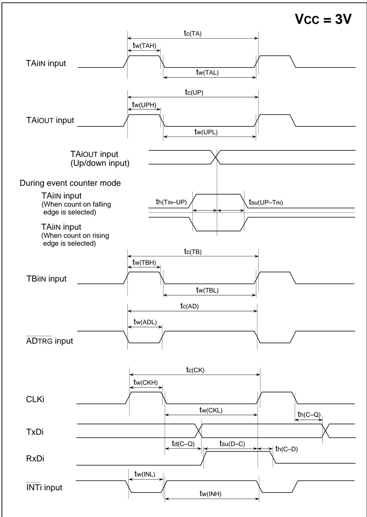
Figure 1.23.8.  $V_{CC} = 3V$  timing diagram (1)
