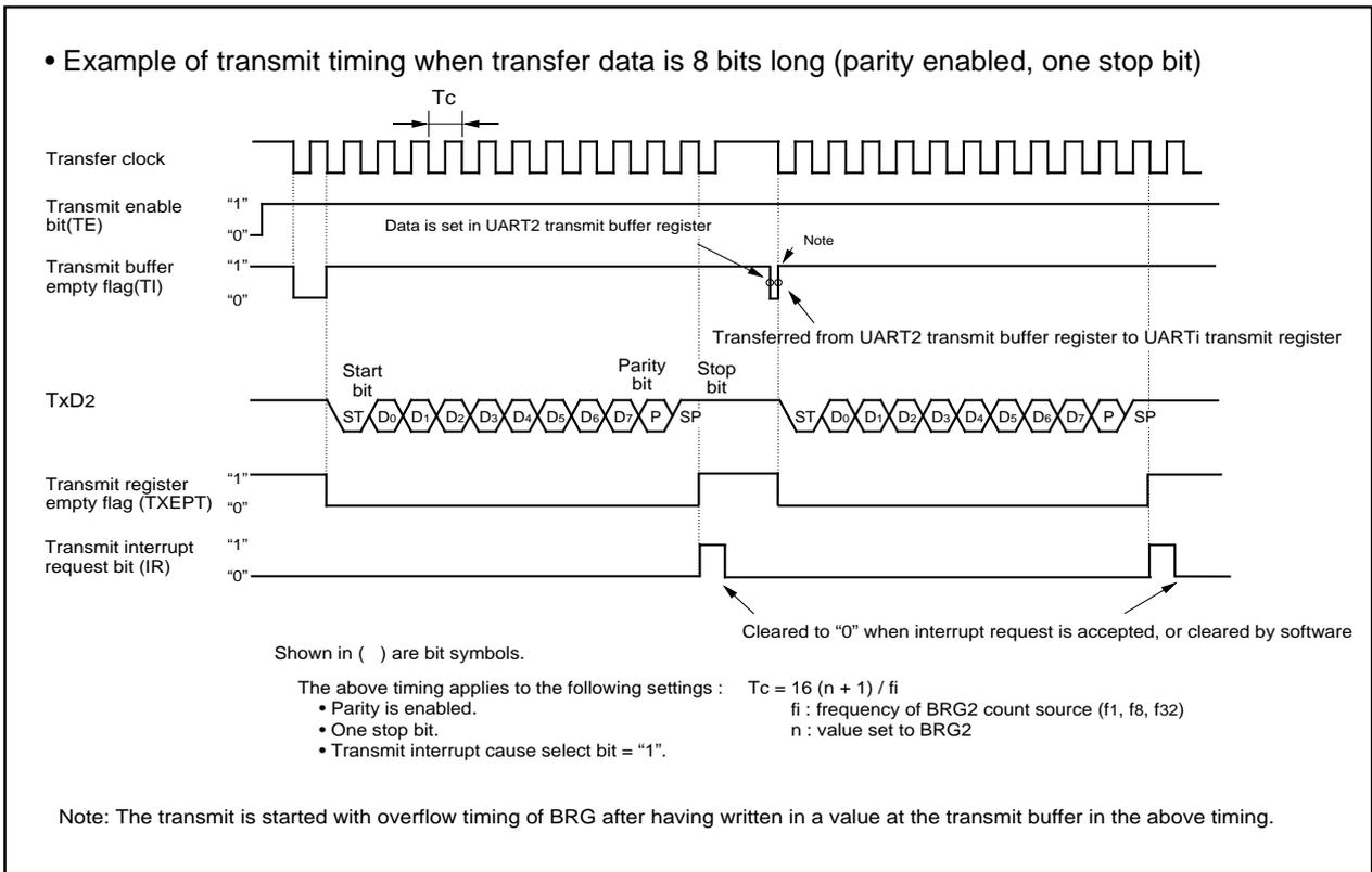
Figure 1.16.18. Typical transmit timings in UART mode(UART2)
