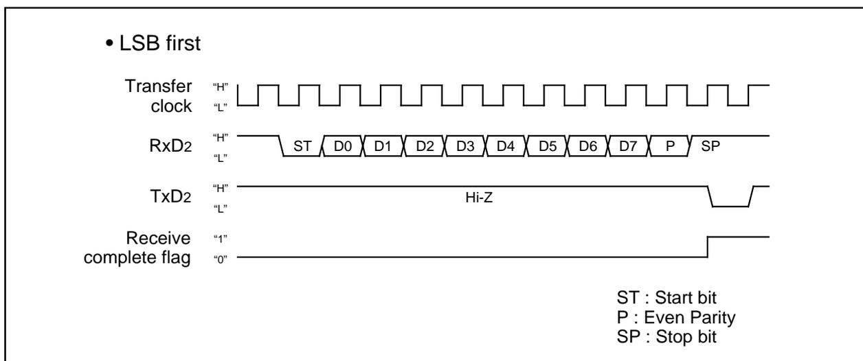
Figure 1.16.23. Output timing of the parity error signal
