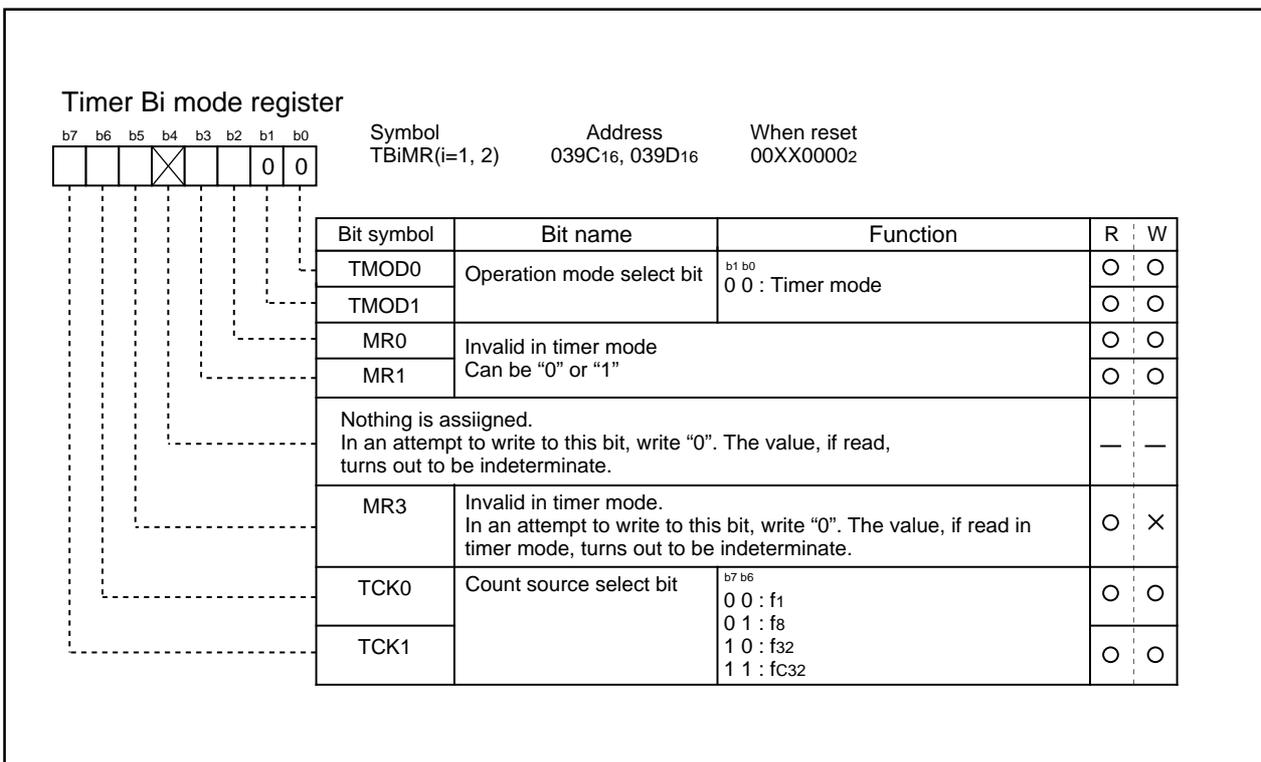
**Figure 1.14.17. Timer Bi mode register in timer mode**
