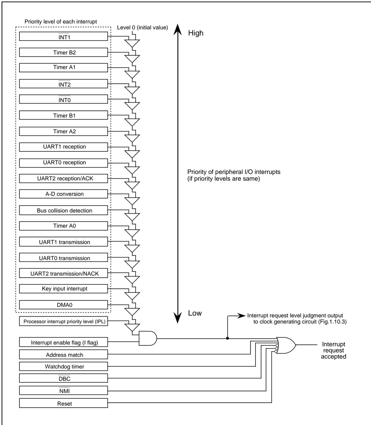
Figure 1.11.9. Maskable interrupts priorities (peripheral I/O interrupts)
