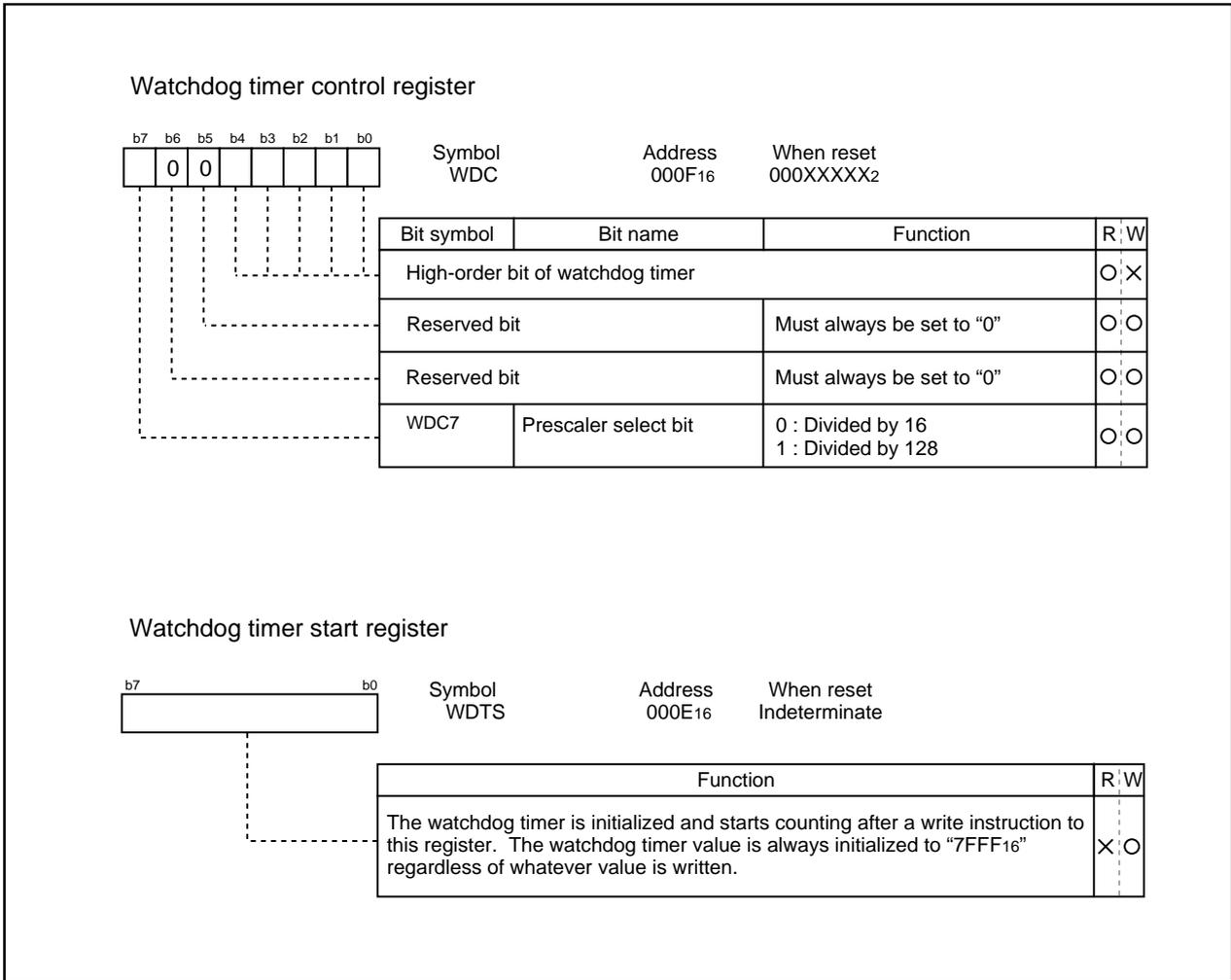
Figure 1.12.2. Watchdog timer control and start registers
