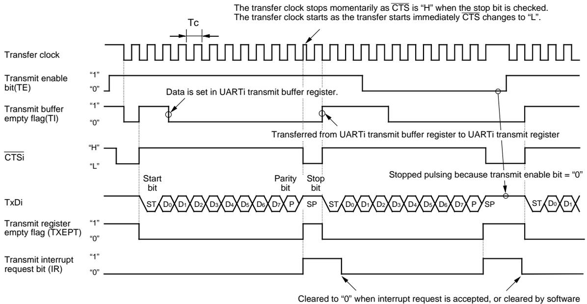
• Example of transmit timing when transfer data is 9 bits long (parity disabled, two stop bits)
