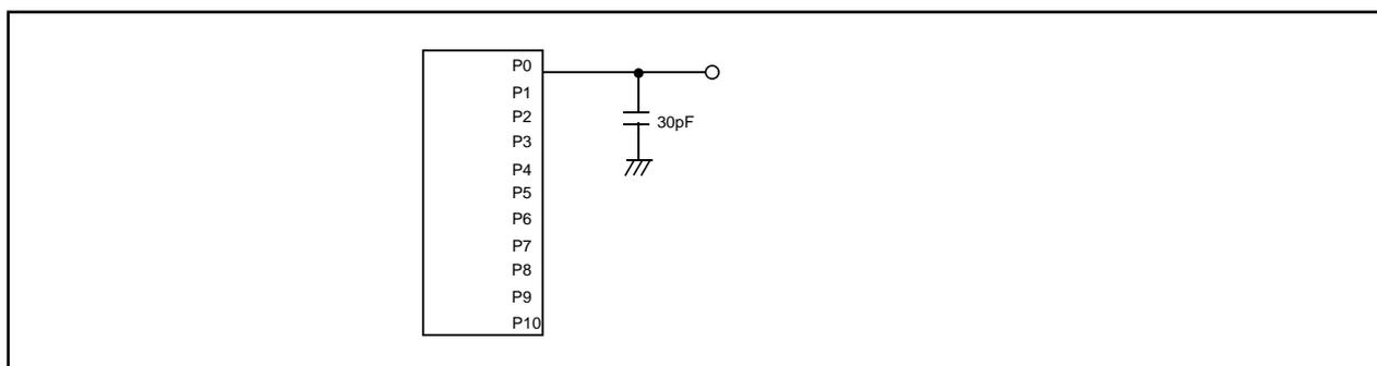
Figure 1.23.1. Port P0 to P10 measurement circuit
