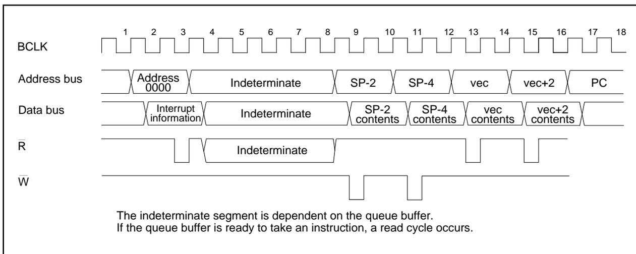
**Figure 1.11.5. Time required for executing the interrupt sequence**
