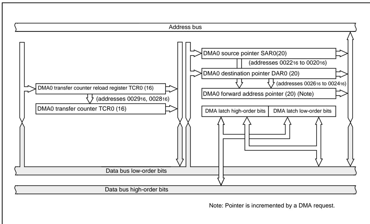
Figure 1.13.1. Block diagram of DMAC
