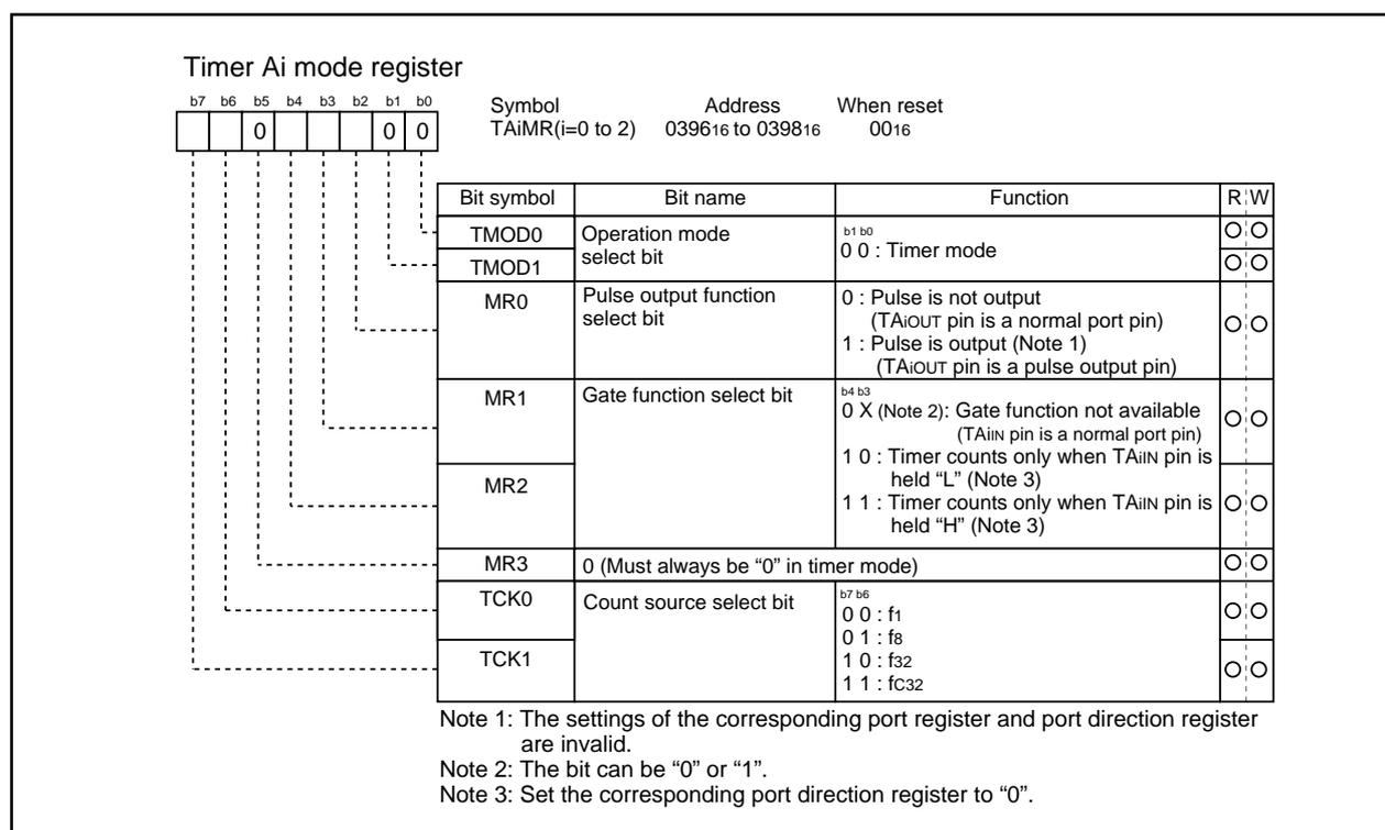
**Figure 1.14.7. Timer Ai mode register in timer mode**
