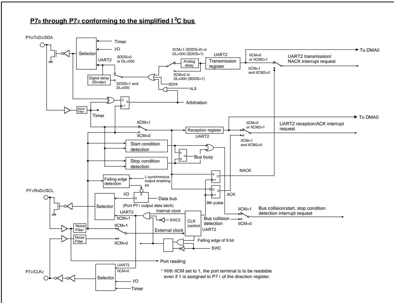
Figure 1.16.27. Functional block diagram for I<sup>2</sup>C mode
