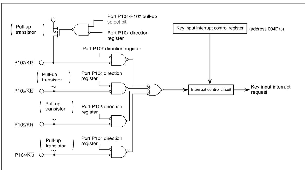
Figure 1.11.11. Block diagram of key input interrupt
