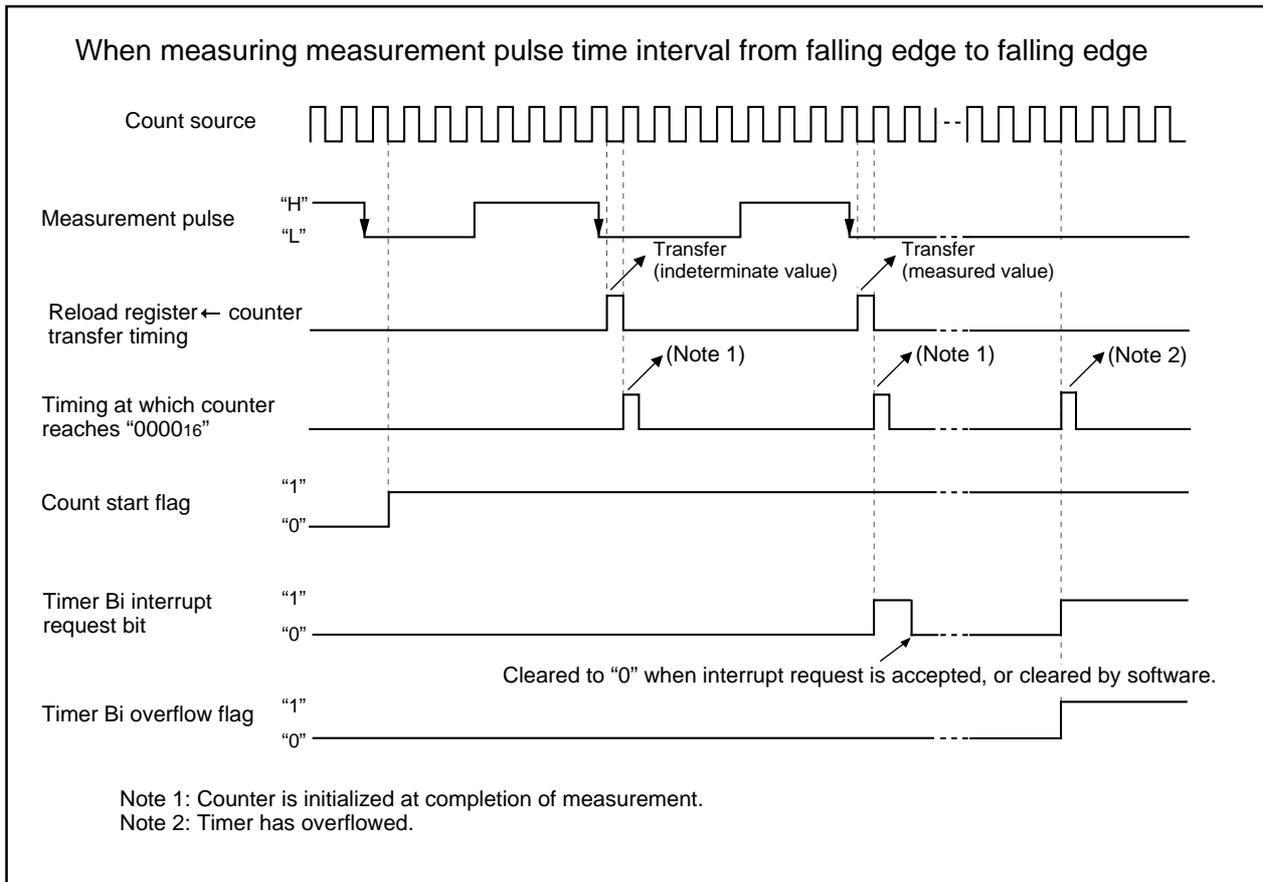
Figure 1.14.20. Operation timing when measuring a pulse period
