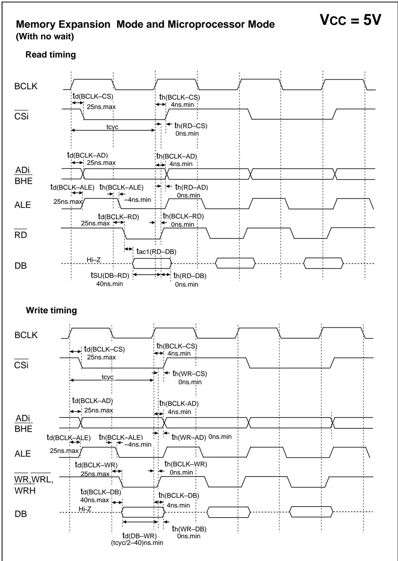
Figure 1.23.4. Vcc = 5V timing diagram (3)
