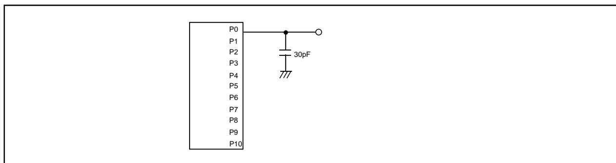
Figure 1.23.7. Port P0 to P10 measurement circuit
