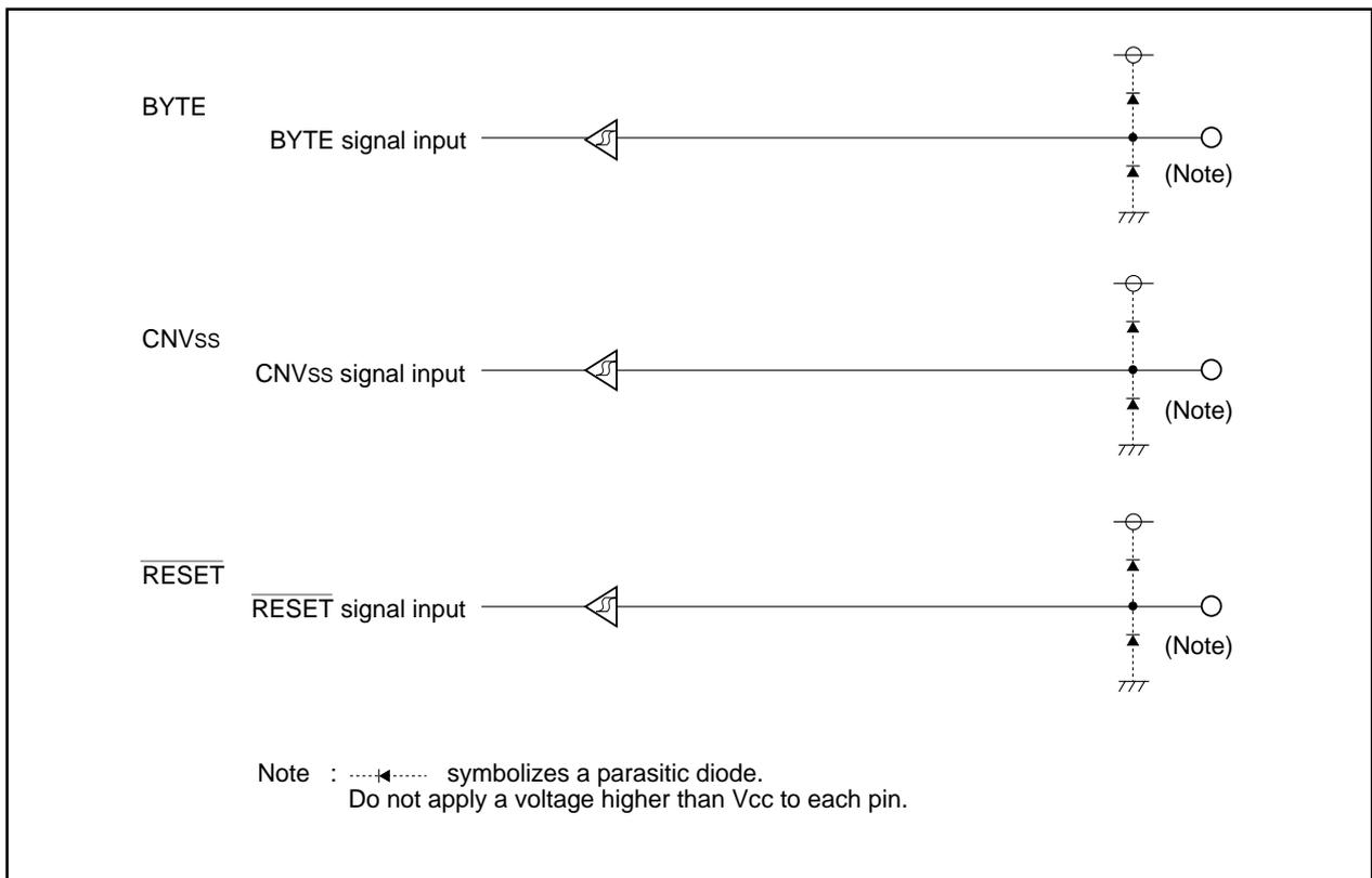
Figure 1.20.5. I/O pins
