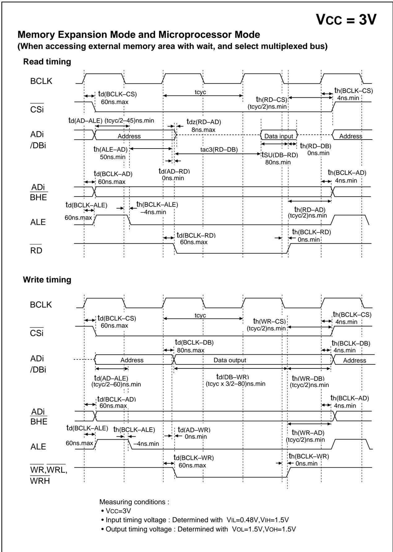
Figure 1.23.12.  $V_{CC} = 3V$  timing diagram (5)
