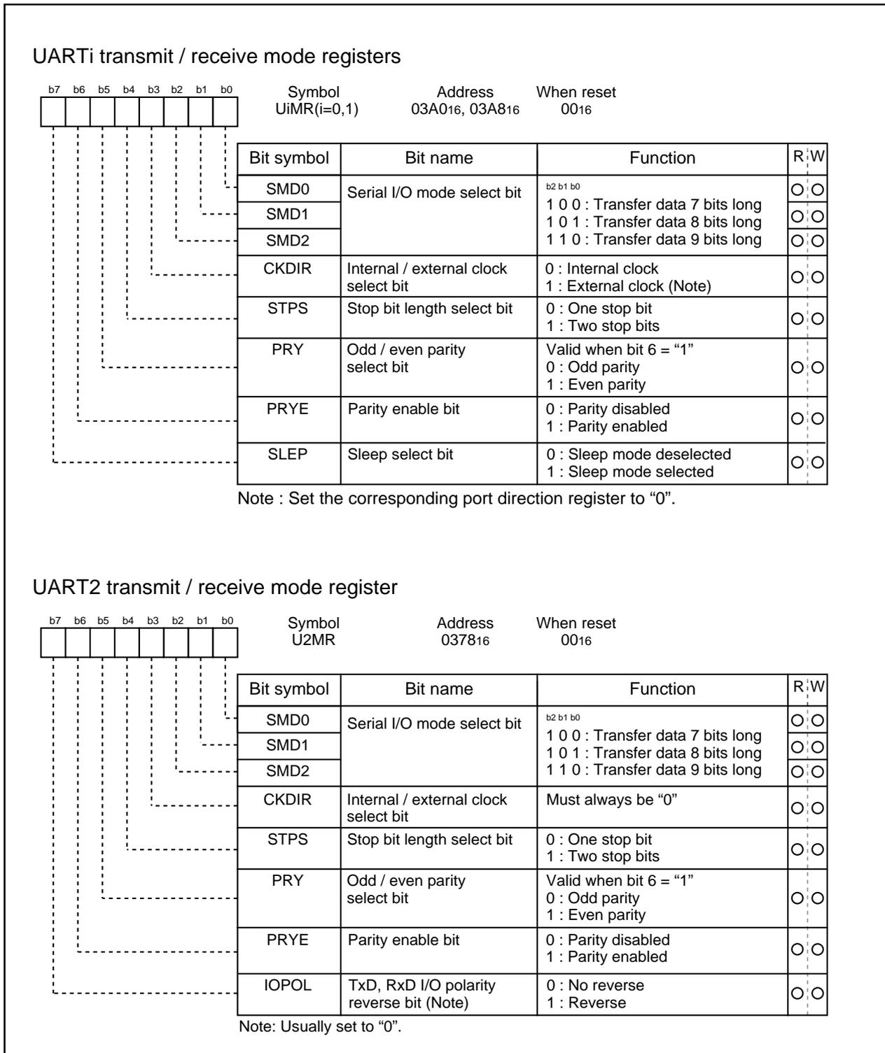
Figure 1.16.16. UART<sub>i</sub> transmit/receive mode register in UART mode
