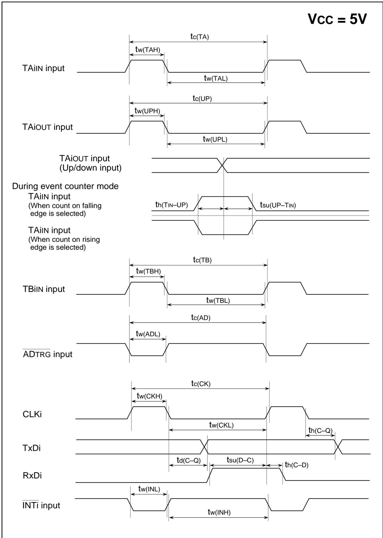
Figure 1.23.2.  $V_{CC} = 5V$  timing diagram (1)
