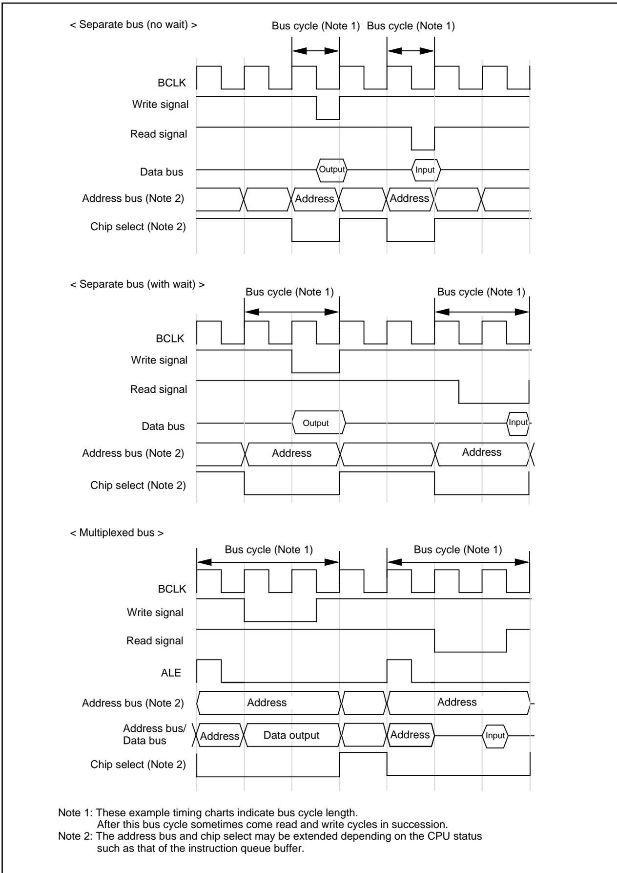
Figure 1.9.6. Typical bus timings using software wait
