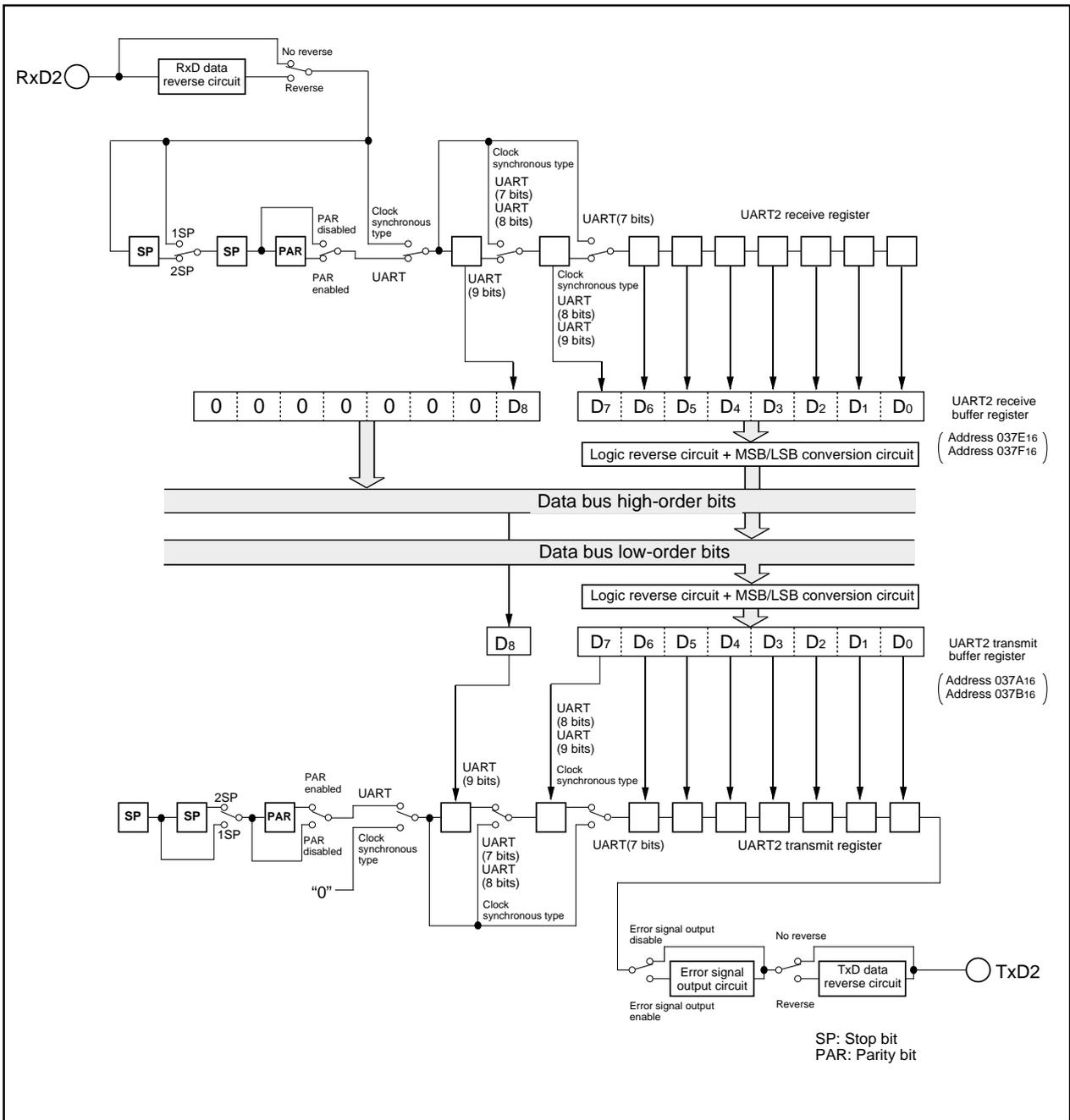
Figure 1.16.3. Block diagram of UART2 transmit/receive unit
