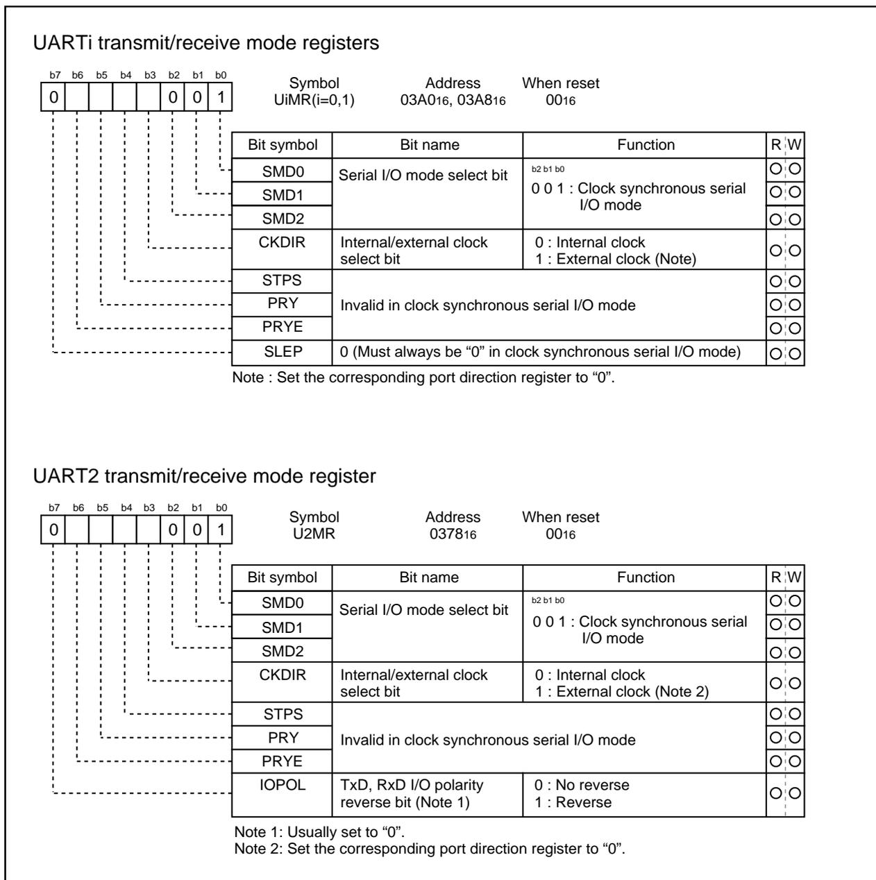
Figure 1.16.10. UART<sub>i</sub> transmit/receive mode register in clock synchronous serial I/O mode
