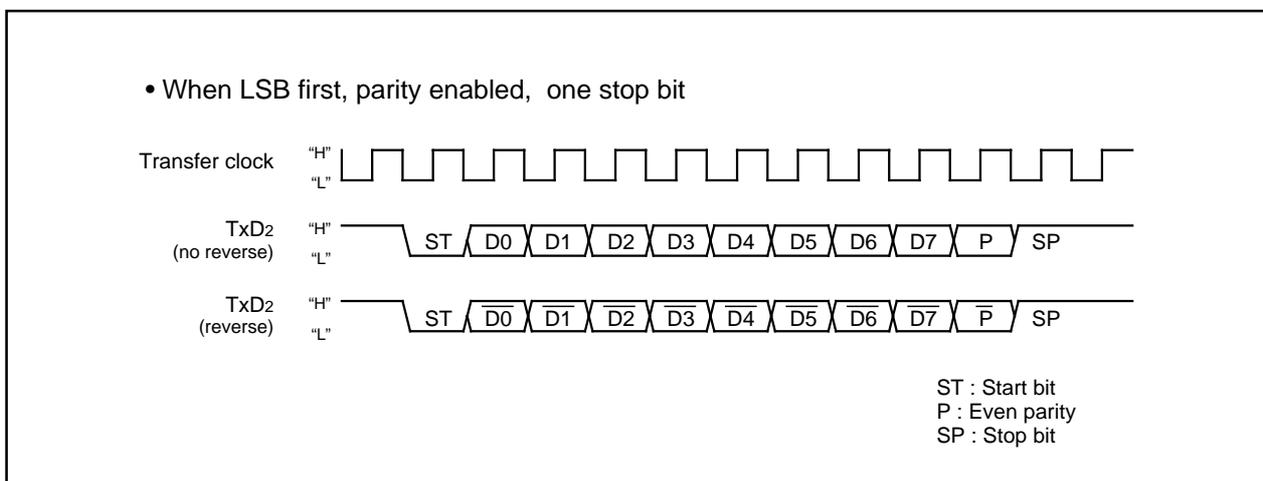
Figure 1.16.20. Timing for switching serial data logic
