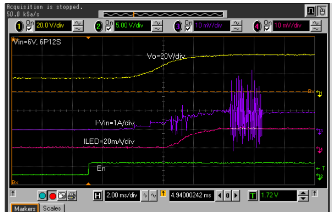
FIGURE 12. IN-RUSH and LED CURRENT AT V_{IN} = 6V FOR 6P12S AT 20mA/CHANNEL
