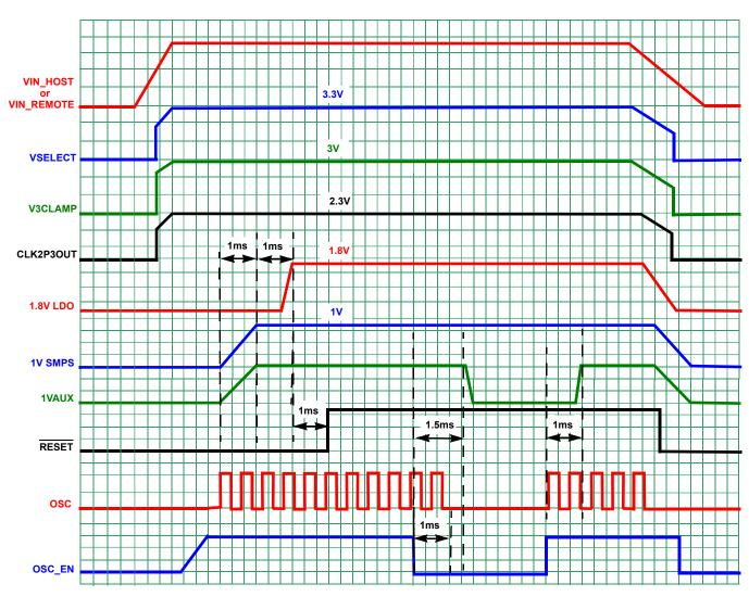
FIGURE 36. START-UP AND SHUTDOWN SEQUENCE
