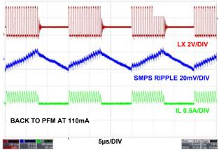
FIGURE 33. PWM TO PFM TRANSITION, VIN = 3.3V
