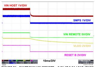
FIGURE 21. SHUTDOWN VIN REMOTE = 3.3V AT 0.8A LOAD (PWM)
