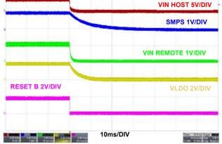
FIGURE 9. SHUT DOWN VIN HOST = 3.3V AT NO LOAD (PWM)
