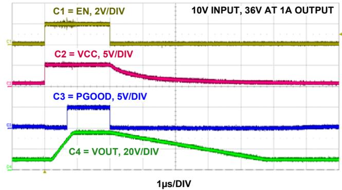
FIGURE 11. ENABLE/DISABLE WAVEFORMS
