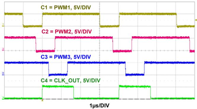
FIGURE 9. WAVEFORMS WITH PWM\_INV = V<sub>CC</sub>
