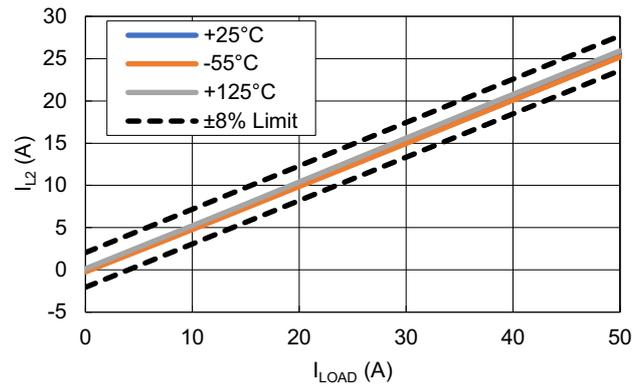
Figure 16. Phase 2 Current Share vs Temperature ( $V_{IN} = 5V$ )
