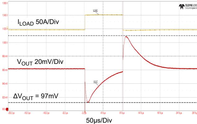
**Figure 55. Transient Response without Droop Regulation**
