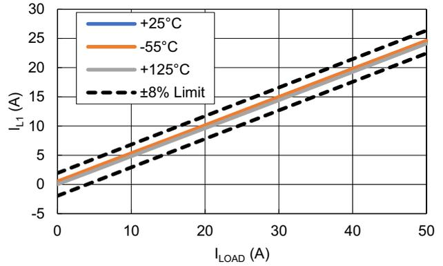
Figure 18. Phase 2 Current Share vs Temperature ( $V_{IN} = 12V$ )
