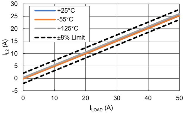
Figure 17. Phase 1 Current Share vs Temperature ( $V_{IN} = 12V$ )
