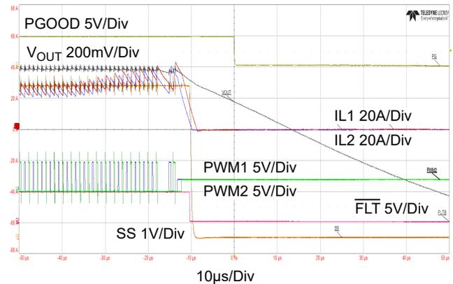
Figure 40. Overcurrent Protection ( $P_{VIN} = V_{DD} = 12V$ )
