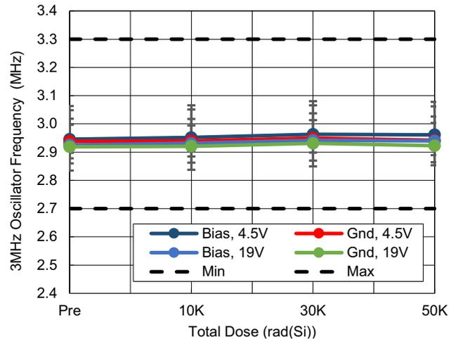
Figure 68. Oscillator Frequency vs TID (f<sub>OSC</sub> = 3MHz)
