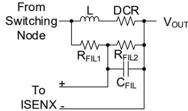
Figure 54. DCR Current Sensing when  $DCR > R_{SEN}$
