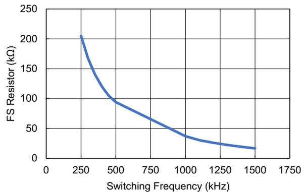
Figure 50. R<sub>FS</sub> vs Frequency
