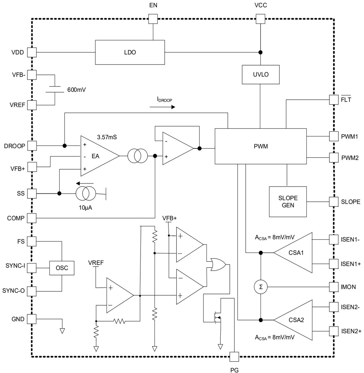
Figure 5. Block Diagram
