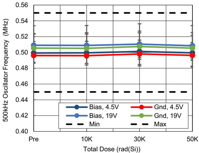
Figure 67. Oscillator Frequency vs TID (f<sub>OSC</sub> = 0.5MHz)
