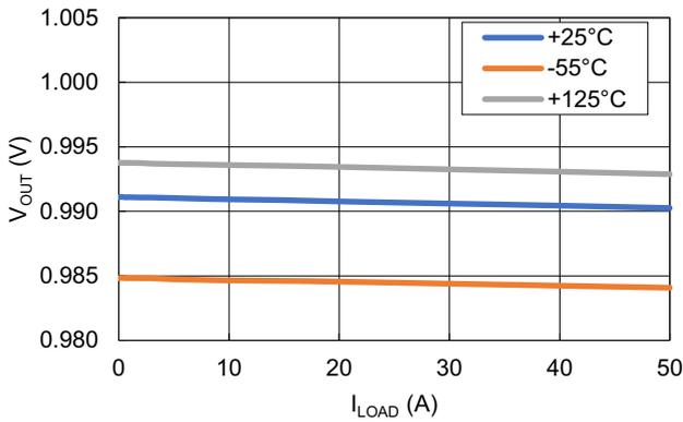
Figure 8. Load Regulation for Various Temperatures ( $V_{IN} = 5V$ )
