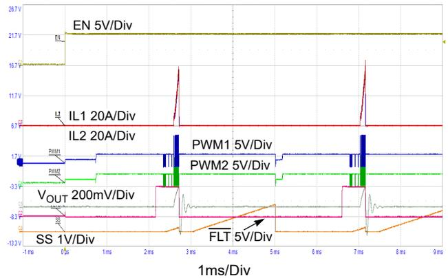
Figure 42. Start-Up with a Short ( $P_{VIN} = V_{DD} = 12V$ )
