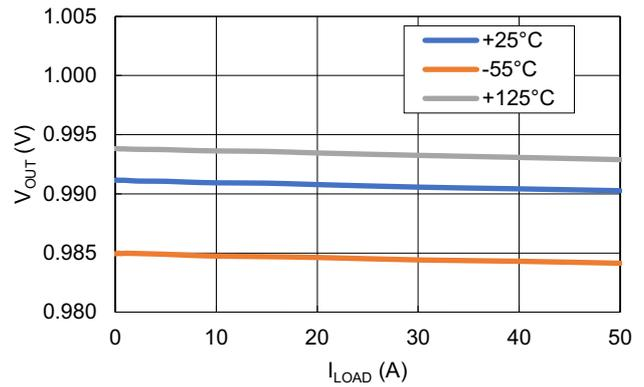
Figure 9. Load Regulation for Various Temperatures ( $V_{IN} = 12V$ )
