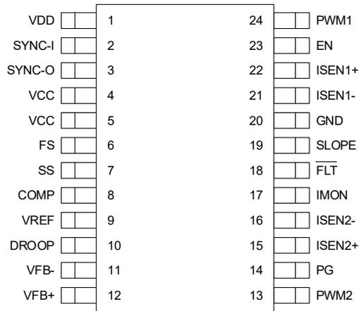
Figure 6. Pin Assignments - 24 Ld WSOIC Top View
