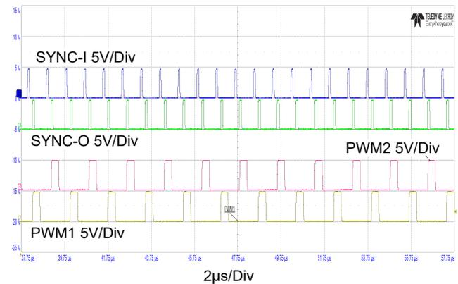
Figure 44. SYNC ( $V_{DD} = 5V$ ,  $P_{VIN} = 12V$ ,  $RSYNC-O = 100k\Omega$  to GND,  $FSYNC-I = 1.15MHz$ )
