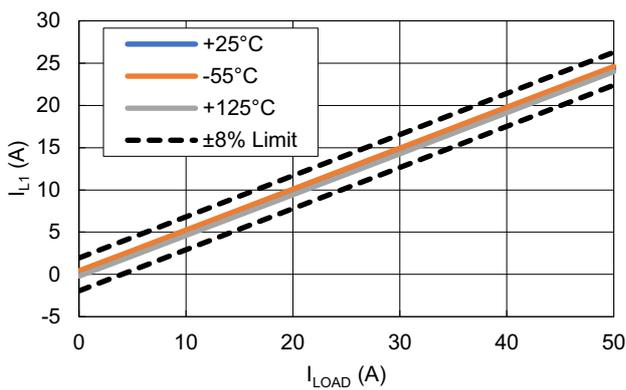
Figure 15. Phase 1 Current Share vs Temperature ( $V_{IN} = 5V$ )
