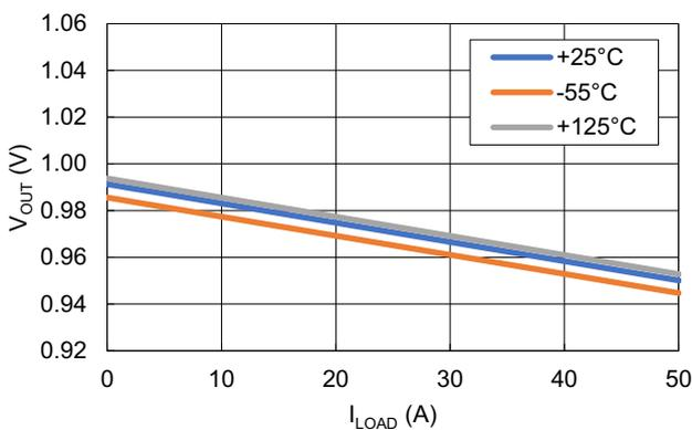
Figure 10. Droop Regulation for Various Temperatures ( $V_{IN} = 5V$ ,  $R_{DROOP} = 604\Omega$ )
