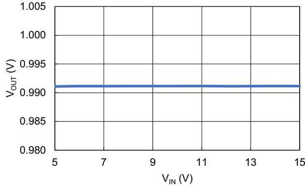
Figure 12. Line Regulation ( $I_{LOAD} = 0A$ )
