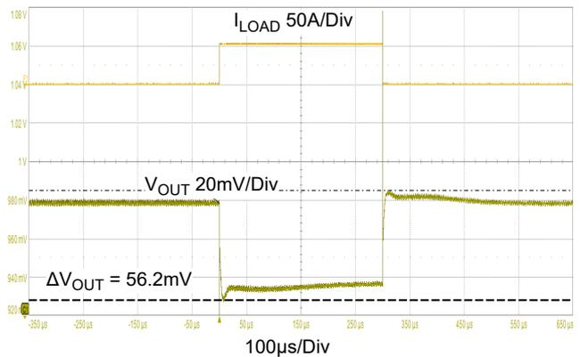
Figure 26. Load Transient Response
