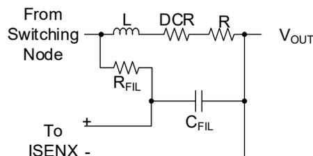
Figure 53. DCR Current Sensing when  $DCR < R_{SEN}$
