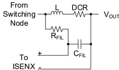
Figure 52. DCR Current Sensing when  $DCR = R_{SEN}$
