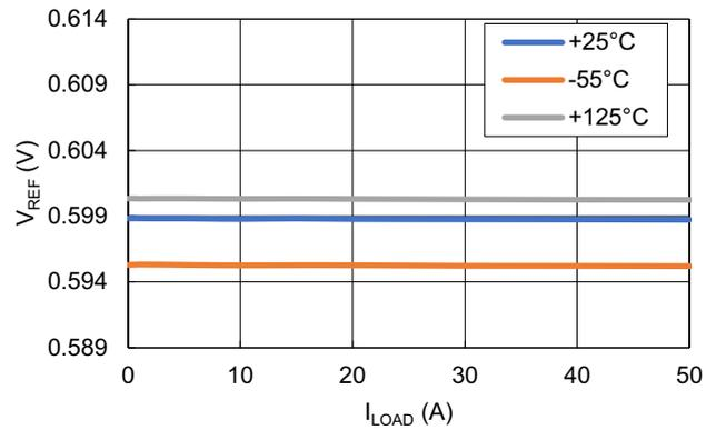
Figure 14.  $V_{REF}$  Accuracy for Various Temperatures ( $V_{IN} = 12V$ )
