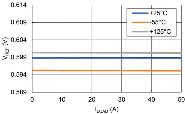
Figure 13.  $V_{REF}$  Accuracy for Various Temperatures ( $V_{IN} = 5V$ )
