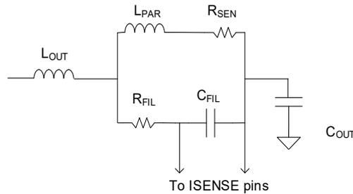
Figure 51.  $R_{SEN}$  Parasitic Inductance Compensation RC Circuit
