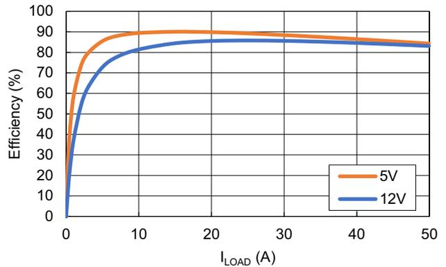
Figure 20. Conversion Efficiency for Various  $V_{IN}$  ( $f_{SW} = 250kHz$ , Tested on the ISL73847MDEMO1Z),  $L_{OUT} = 450nH$  per phase,  $C_{OUT} = 5.28mF$  per phase,  $C_{COMP} = 15nF$ ,  $C_{DROOP} = 100nF$ ,  $R_{FS} = 205k\Omega$
