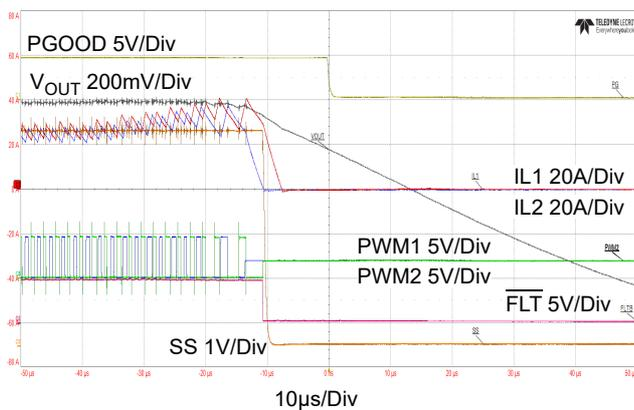
Figure 39. Overcurrent Protection ( $P_{VIN} = 12V$ ,  $V_{DD} = 5V$ )
