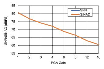
Figure 28. SNR and SINAD vs PGA Gain
