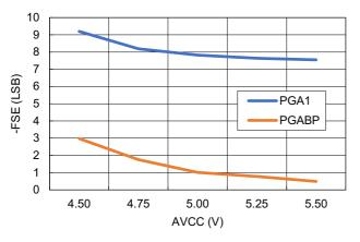
Figure 91. -Full-Scale Error vs AVCC
