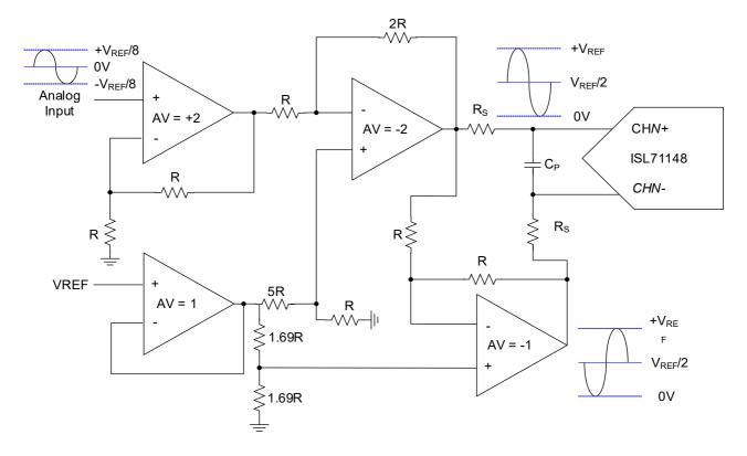
Figure 125. Common-Mode Conversion Amplifier Example Circuit
