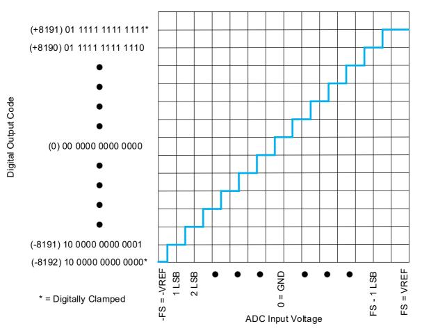
Figure 126. Transfer Function - Differential Input Channels
