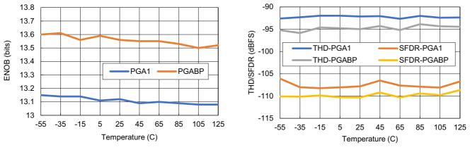
Figure 118. ENOB vs Temperature
