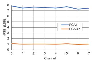
Figure 49. -Full-Scale Error vs Channel
