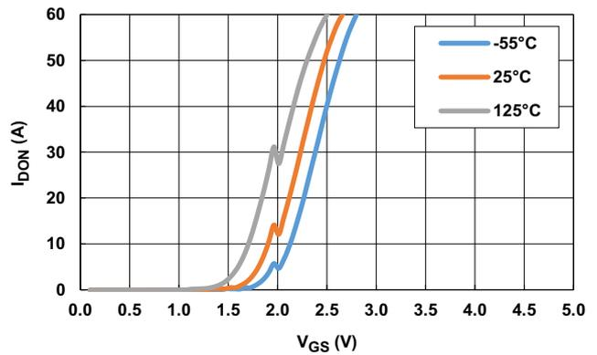
Figure 6. Transfer Characteristics
