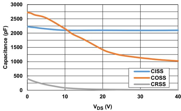
Figure 11. Capacitance (Linear Scale)
