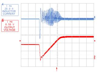
FIGURE 6. PRE-BIASED STARTUP IN CCM MODE
