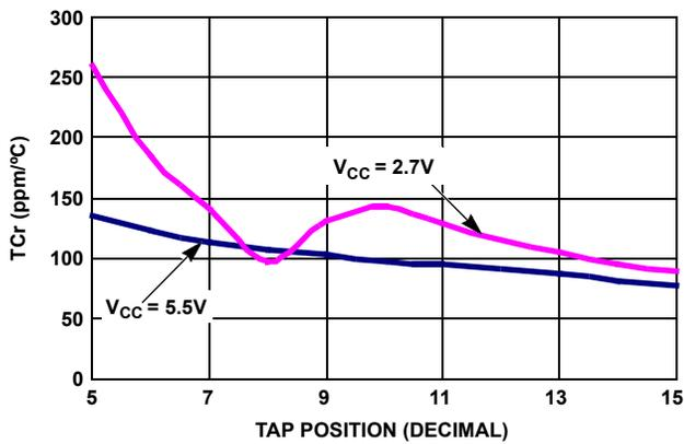
FIGURE 11. TC FOR RHEOSTAT MODE IN ppm
