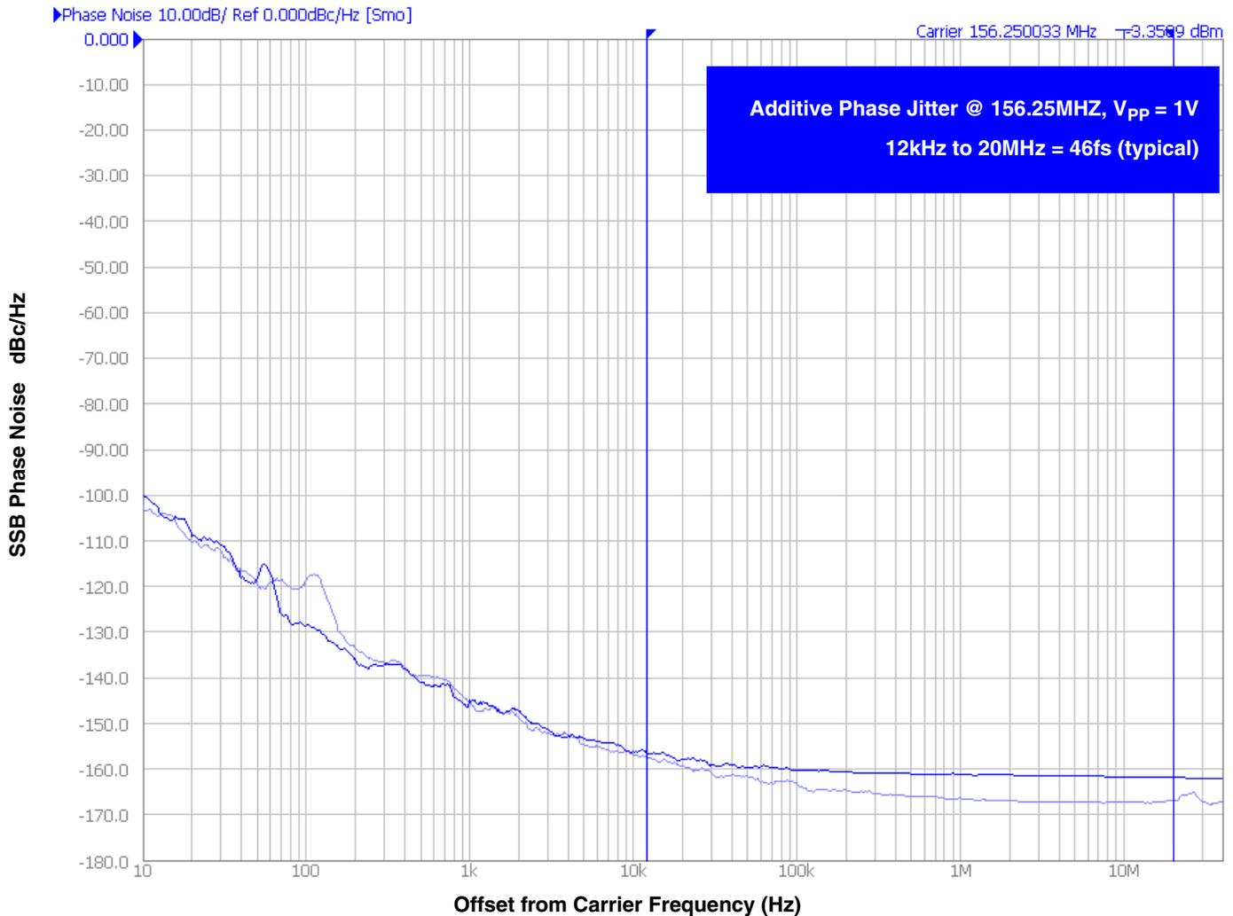
As with most timing specifications, phase noise measurements have issues relating to the limitations of the equipment. Often the noise floor of the equipment is higher than the noise floor of the device. This is illustrated above. The device meets the noise floor of what is shown, but can actually be lower. The phase noise is dependent on the input source and measurement equipment.
