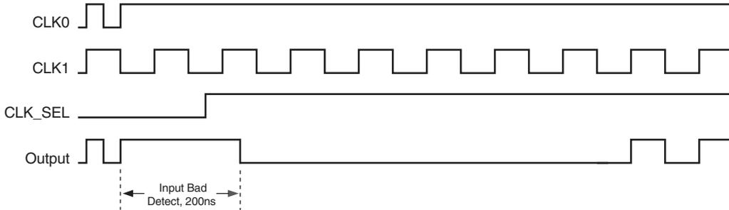
Figure 1G. CLK\_SEL with Bad Input Timing Diagram
