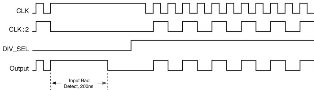
Figure 1E. DIV\_SELx with Bad Input Timing Diagram
