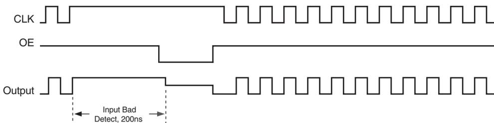
Figure 1F. OEx with Bad Input Timing Diagram
