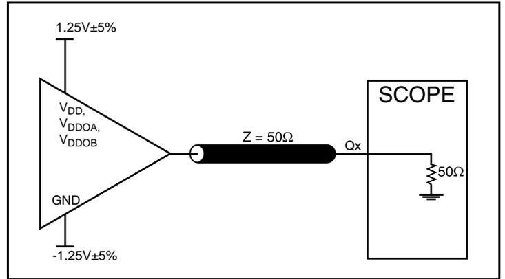
2.5V Output Load Test Circuit
