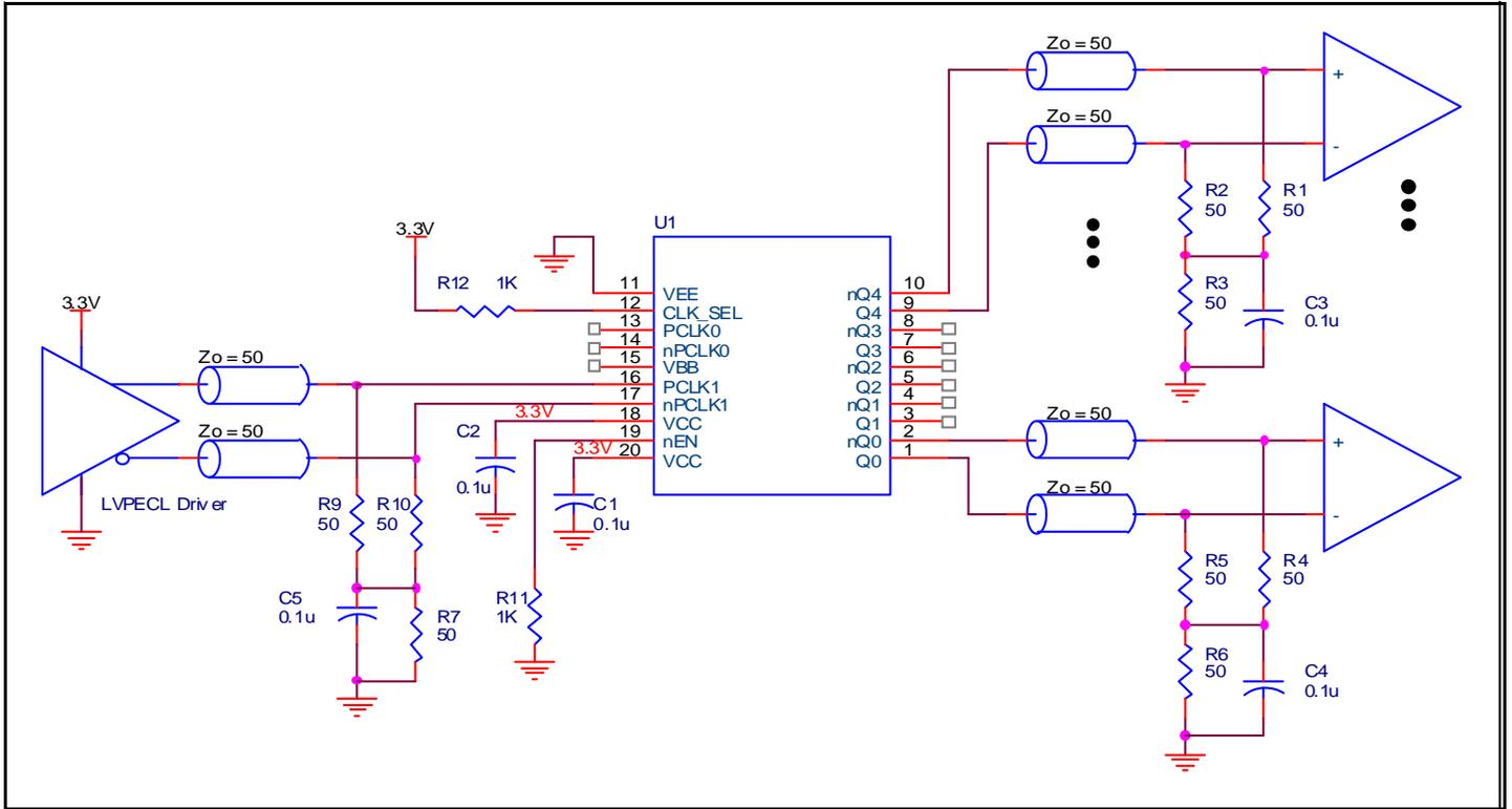
Figure 6. ICS853S014I Example LVPECL Clock Output Buffer Schematic
