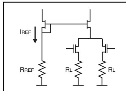
**Figure 1. HCSL Current Mirror and Output Drive**
