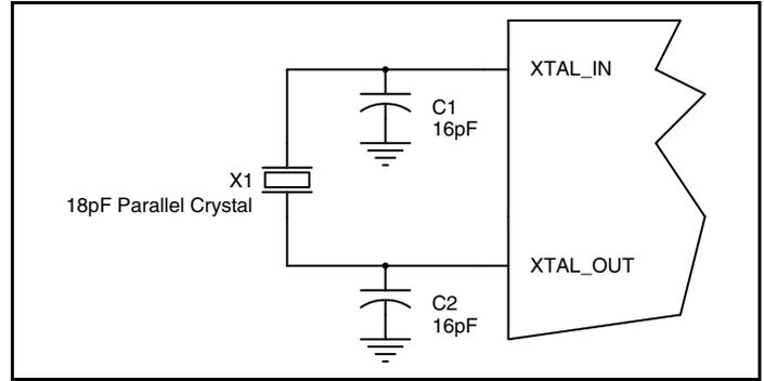
**Figure 2B. Crystal Input Interface, using 18pF crystal**
