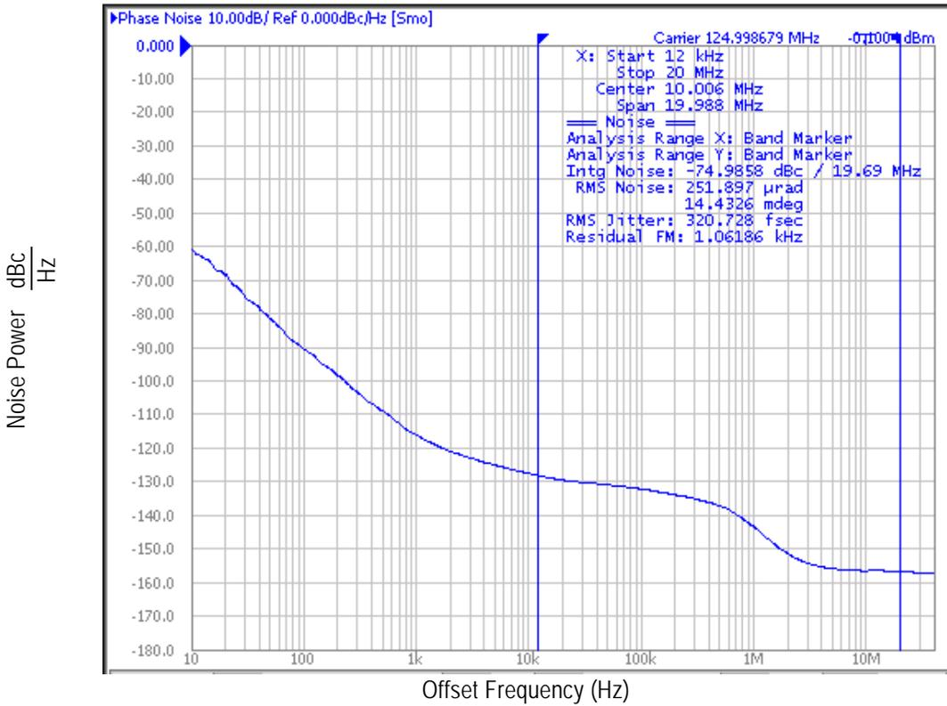
Typical Phase Noise at 150MHz (3.3V core, 3.3V output)
