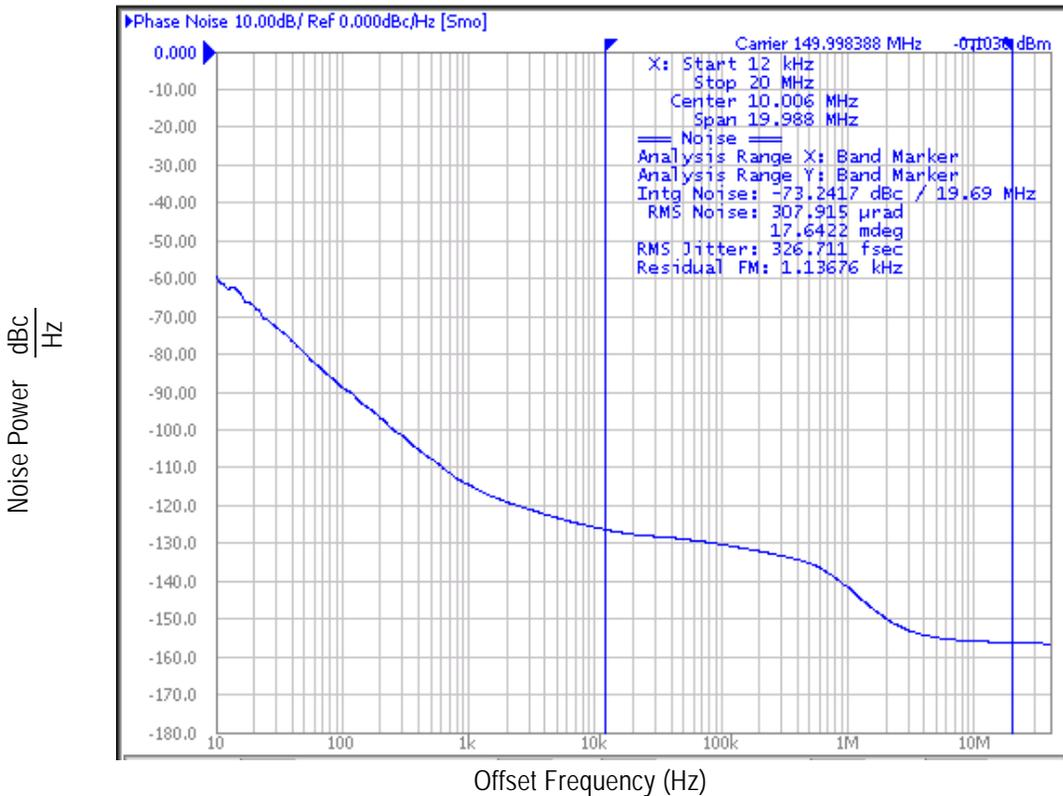
Typical Phase Noise at 156.25MHz (3.3V core, 3.3V output)
