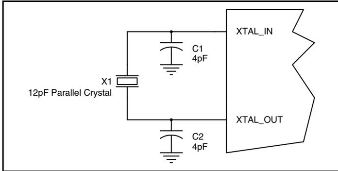
**Figure 2A. Crystal Input Interface, using 12pF crystal**
