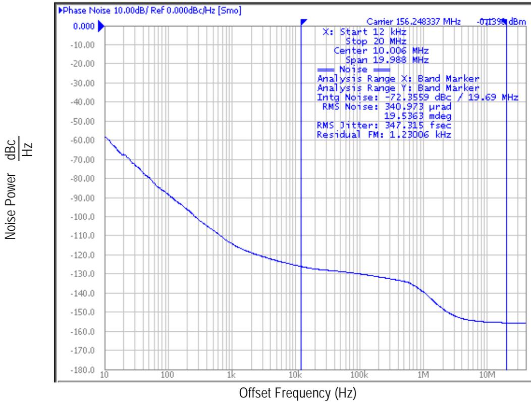
Typical Phase Noise at 187.5MHz (3.3V core, 3.3V output)
