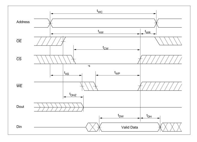
Write Timing Waveform (2) (OE Low Fixed)
