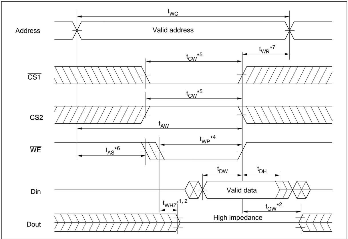
Write Cycle (2) ( $\overline{CS}$  Clock,  $\overline{OE} = V_{IH}$ )
