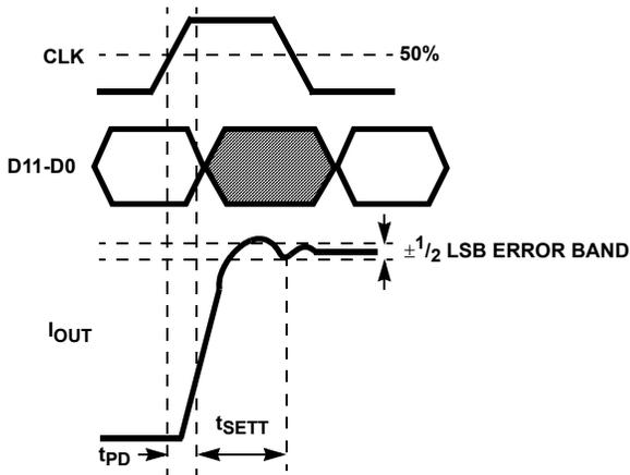
**FIGURE 1. FULL SCALE SETTLING TIME DIAGRAM**
