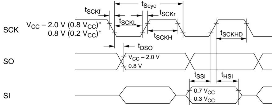
Note: \*  $V_{CC} - 2.0\text{ V}$  and  $0.8\text{ V}$  are the threshold voltages for transmit clock output.
