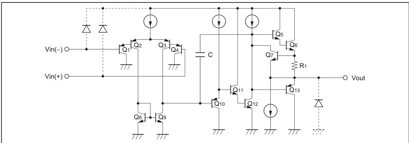
Note: If Input/Output terminals voltage over the absolute maximum ratings, there is possibility of mis-operation, characteristics deterioration and destruction, because of the current's flowing to parasitic diode in IC. The Input/Output terminals are recommended to be protected with the clamp circuit which using the diode with low forward voltage (like schottky barrier diode) when there is a possibility for the Input/Output terminals voltage exceeds the absolute maximum ratings.
