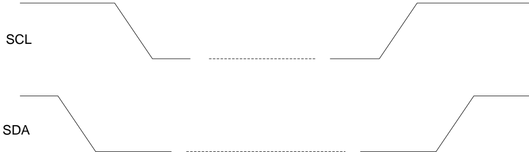
Figure 17: I 2 C START and STOP Condition Timing
