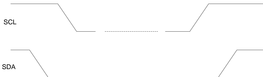
Figure 24. Timing of 2-WIRE START and STOP Condition
