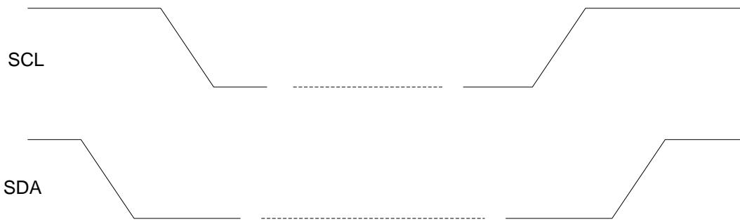
Figure 16. I<sup>2</sup>C START and STOP Condition Timing
