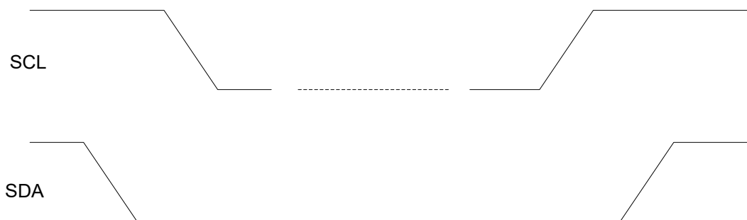
Figure 18: I 2 C START and STOP Condition Timing
