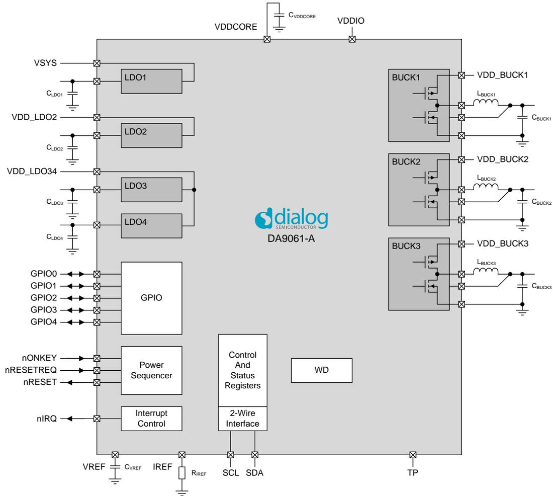
Figure 1: DA9061-A Block Diagram
