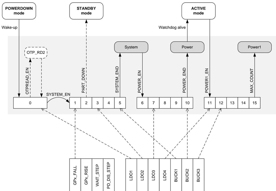
Figure 19: Structure of the Power Supply Sequencer
