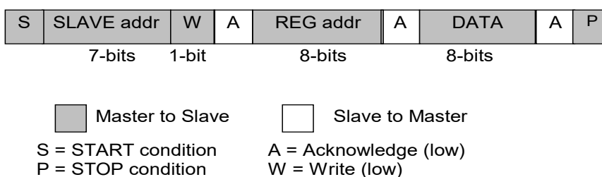
Figure 34: I²C Byte Write (SDA line)
