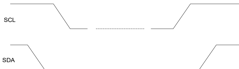
Figure 26. Timing of I 2 C START and STOP conditions
