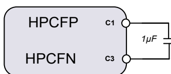
Figure 42. Charge pump flying capacitor
