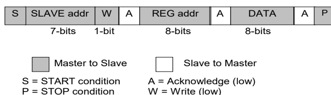
Figure 27. I 2 C byte write (SDA signal)
