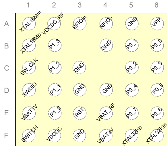
Figure 1: WLCSP34 ball assignment
