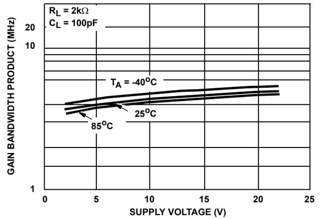
FIGURE 13. GAIN BANDWIDTH PRODUCT vs SUPPLY VOLTAGE
