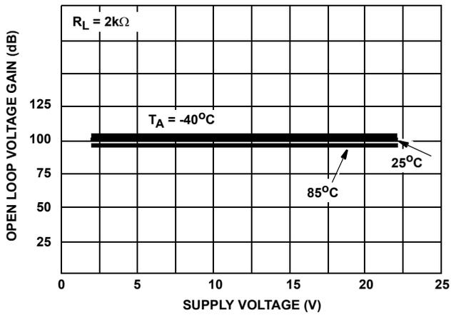
FIGURE 12. OPEN LOOP VOLTAGE GAIN vs SUPPLY VOLTAGE
