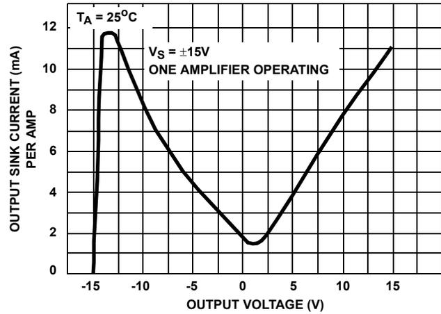
FIGURE 20. OUTPUT SINK CURRENT vs OUTPUT VOLTAGE
