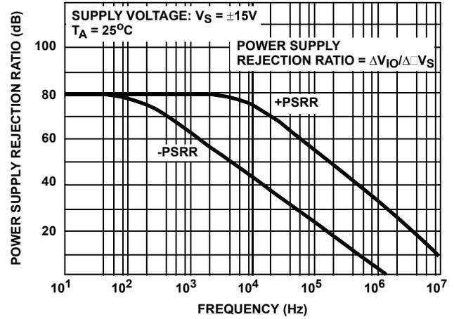
FIGURE 19. POWER SUPPLY REJECTION RATIO vs FREQUENCY
